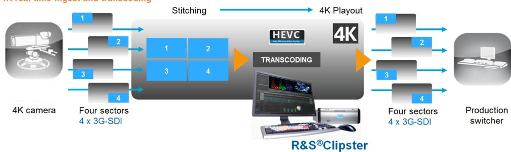
Fig. 2-2: R&S®Clipster – 4K real-time signal ingest via 4 x 3G-SDI, transcoding and playout. This feature will be available in 2014.
