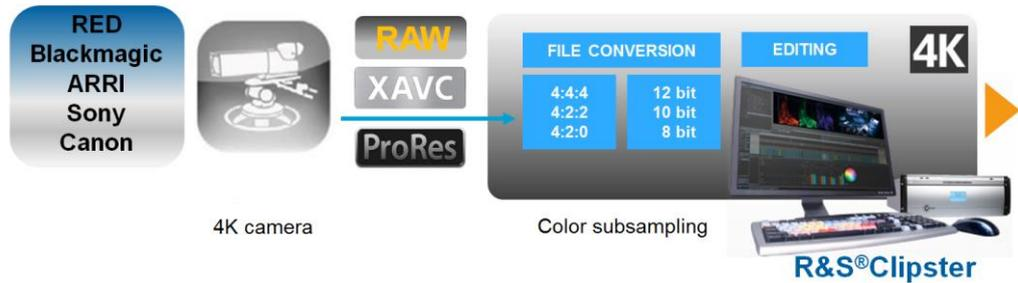
Fig. 2-1: R&S®Clipster – 4K camera file-based ingest supporting various formats and file conversion using different chroma samplings.
