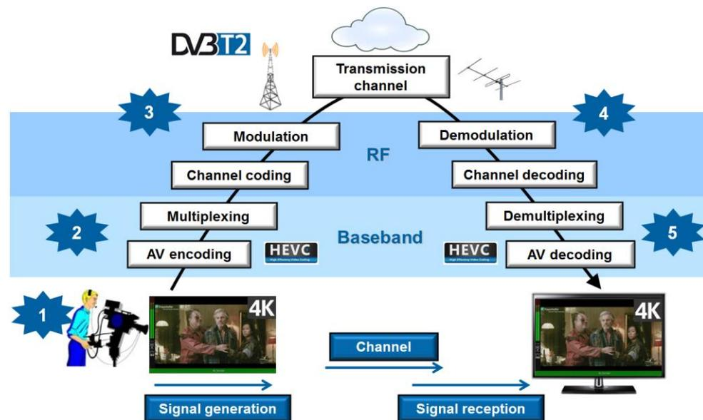
Fig. 1-1: Illustration of the broadcasting chain showing UHD 4K content acquisition and delivery from post production to households over terrestrial network in five steps.
