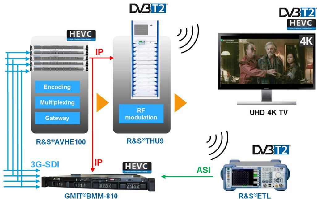
Fig. 5-1: DVB-T2 RF demodulation by the R&S®ETL TV analyzer and real time HEVC decoding and comparison (uncompressed and compressed UHD) using the GMIT®BMM-810.
