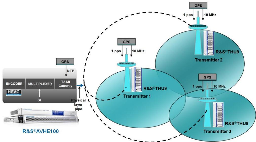
Fig. 4-1: DVB-T2 SFN configuration of three transmitter sites using the R&S® AVHE100 encoder/multiplexer/gateway and the R&S® THU9 high-power DVB-T2 transmitter from Rohde & Schwarz.
