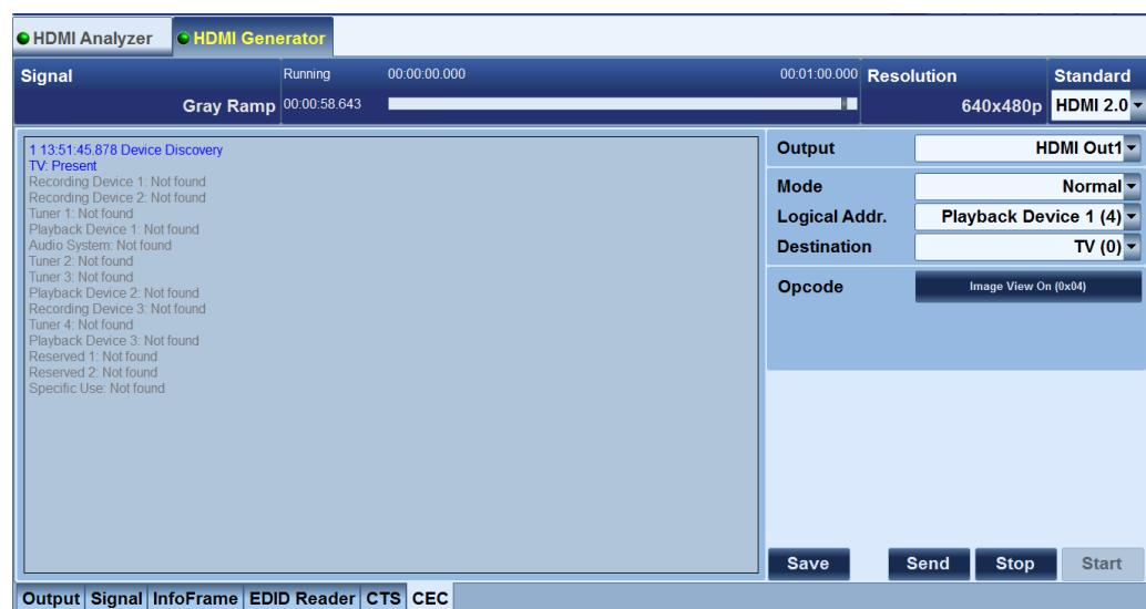
Fig. 5-9: R&S®VTC/VTE/VTS: Checking CEC commands.
