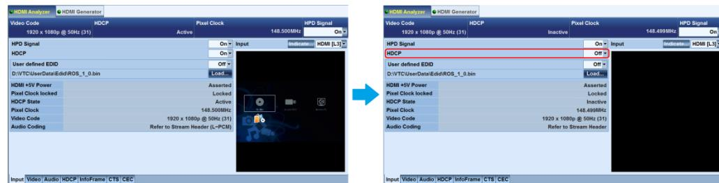
**Fig. 4-5: R&S®VTC/VTE/VTS:** After HDCP is disabled (right), the picture and sound for protected A/V material must not be visible or audible.
