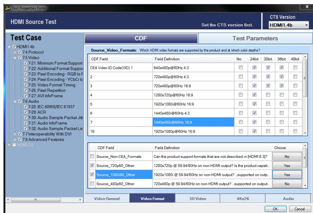
Fig. 3-2: R&S®AVBrun HDMI Test Suite: DUT functional range defined in the CDF.
