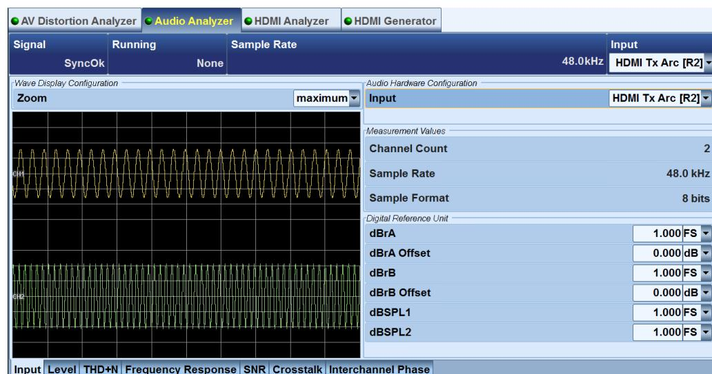
Fig. 5-7: R&S®VTC/VTE/VTS: Checking the audio data transmitted via the ARC.
