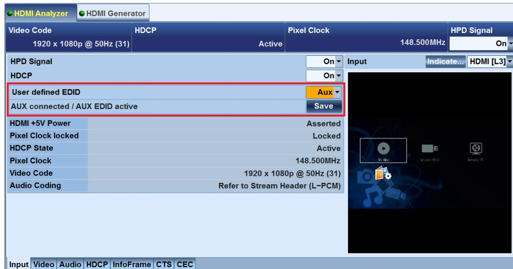
Fig. 4-13: R&S®VTC/VTE/VTS: Configuration for emulating a connected sink.
