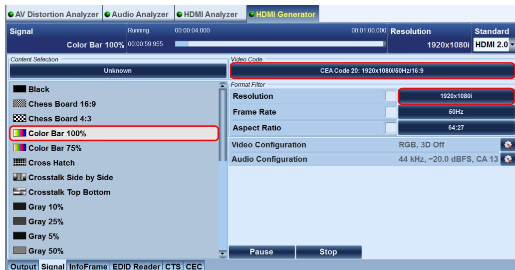
Fig. 5-3: R&S®VTC/VTE/VTS: Selecting the video content and configuring the video format.
