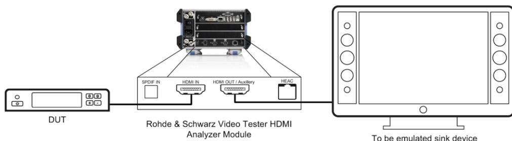
Fig. 4-12: Test setup for emulating a connected sink.
