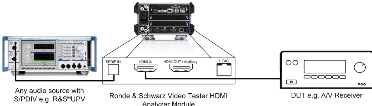
**Fig. 4-10: Testing the ARC using the R&S®VTC/VTE/VTS.**
