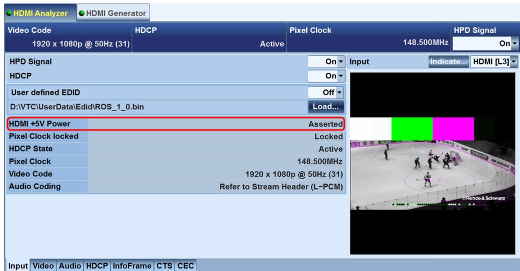
Fig. 4-11: R&S®VTC/VTE/VTs: Display of the present and stable supply voltage.
