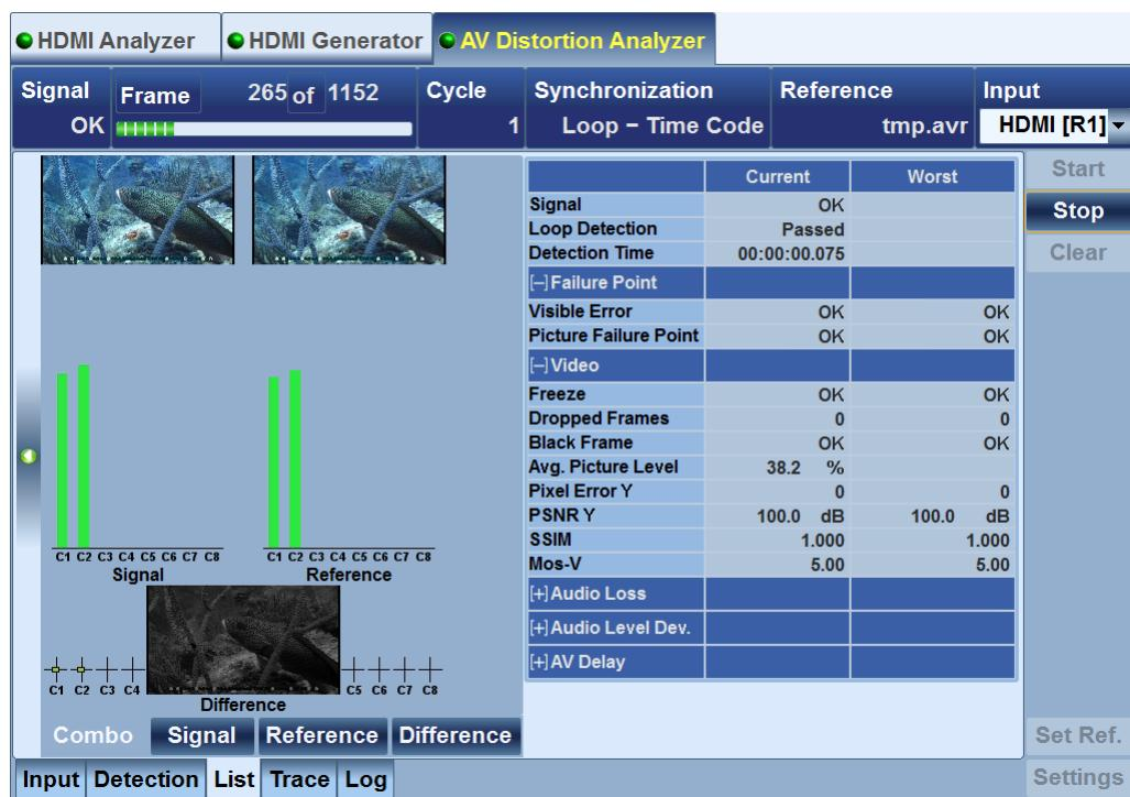
Fig. 4-16: R&S®VTC/VTE/VTS: A/V distortion analysis for assessment of the A/V quality.
