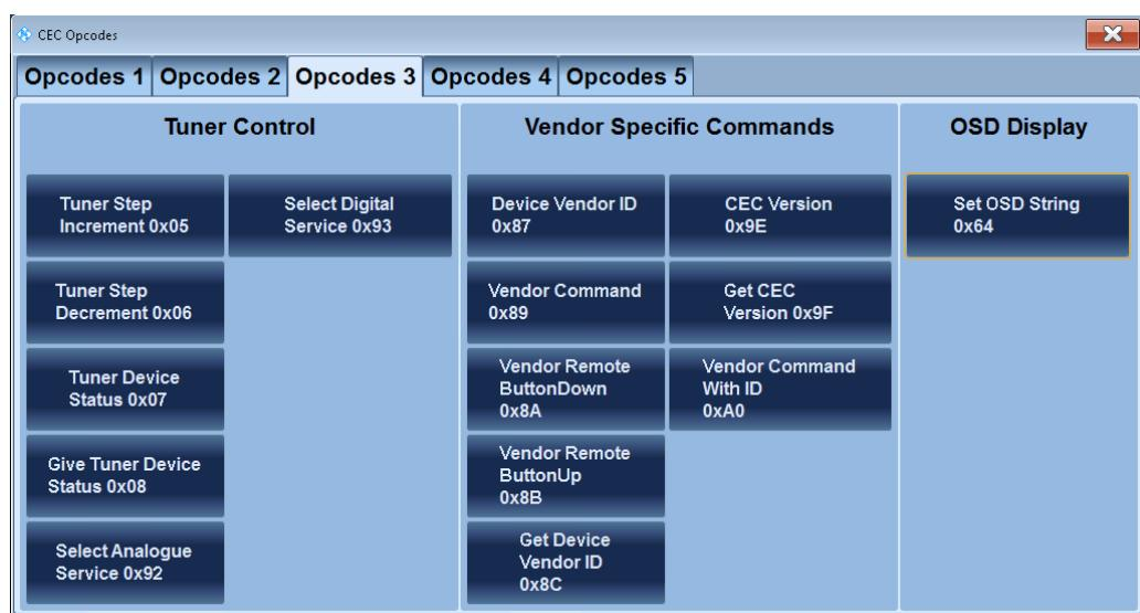
Fig. 4-15: R&S®VTC/VTE/VTS: Selecting the CEC command.
