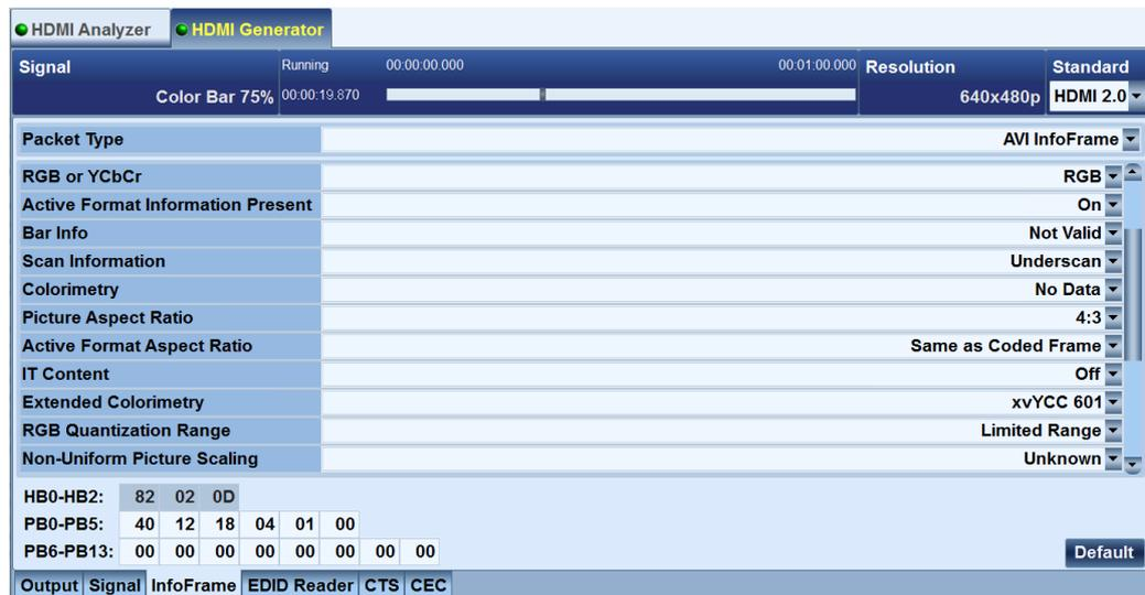
Fig. 5-5: R&S®VTC/VTE/VTs: Configuring the InfoFrames independently of the transmitted A/V data.
