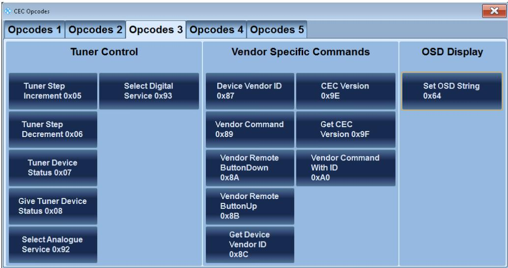
Fig. 4-15: R&S®VTC/VTE/VTs: Selecting the CEC command.
