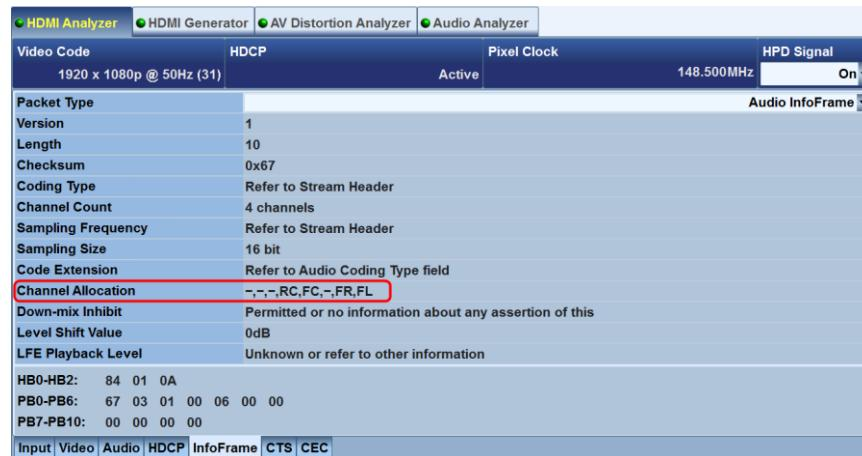
Fig. 4-8: R&S®VTC/VTE/VTS: Audio InfoFrame and the Channel Allocation parameter.
