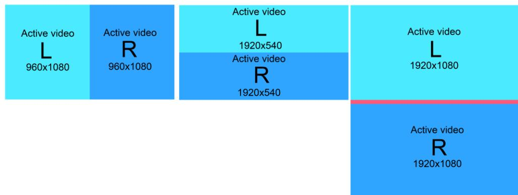
**Fig. 2-4: The various 3D formats: Side-by-side (left), top-and-bottom (middle) and frame packing (right).**
