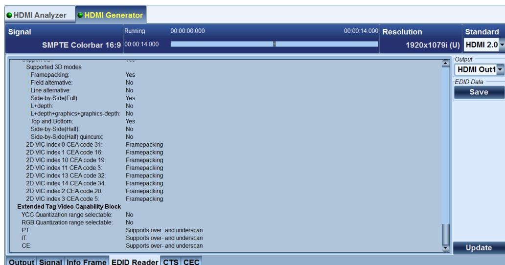
Fig. 5-8: R&S®VTC/VTE/VTS: Reading out the EDID data for a connected sink that is powered off.
