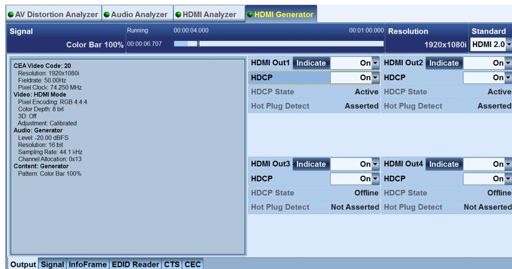
**Fig. 5-1:** R&S®VTC/VTE/VTS: The HDMI generator module permits up to four DUTs to be supplied with the HDMI signal simultaneously.
