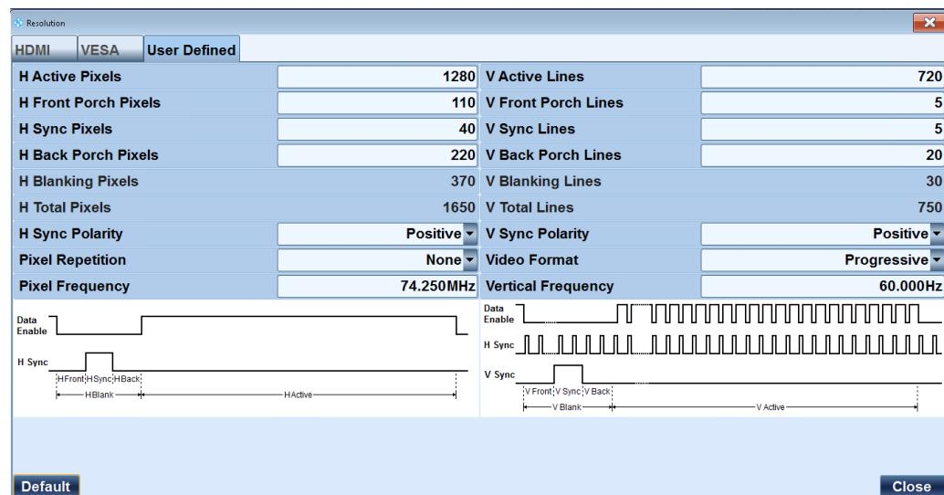
Fig. 5-4: R&S®VTC/VTE/VTS: Configuring a user-defined video format.
