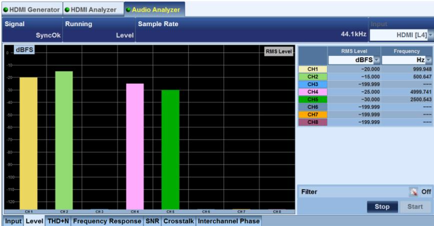
Fig. 4-9: R&S®VTC/VTE/VTs: Checking which channels are transmitting audio data.
