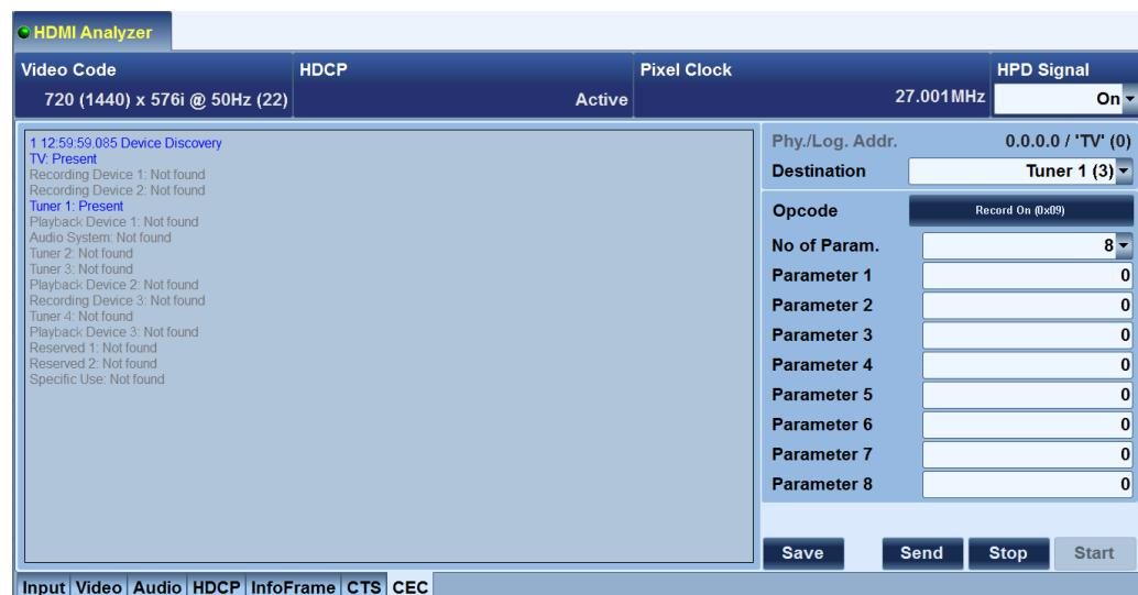
Fig. 4-14: R&S®VTC/VTE/VTS: Display on the instrument after a device discovery.
