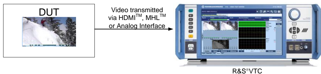
Fig. 2: Audio/video distortion analysis for a DUT, e.g. set-top box or smartphone.
