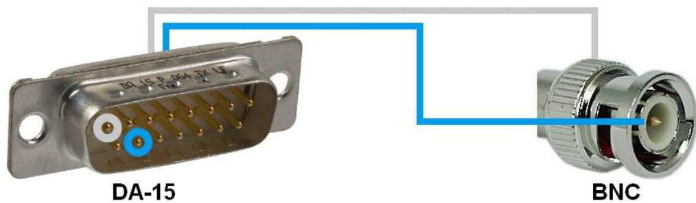
Fig. 4: The required adapter cable connects the DA-15 pin (blue) with the BNC inner contact and the other pin (gray) with the outer contact
