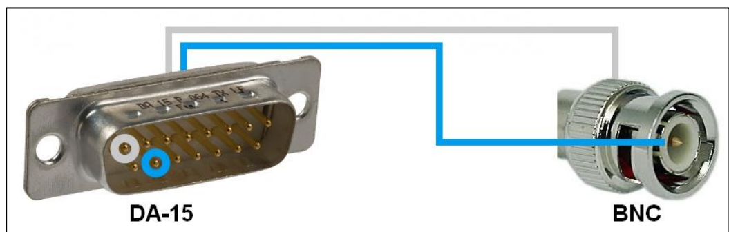
Fig. 6: The required adapter cable connects the DA-15 pin (blue) with the BNC inner contact and the other pin (grey) with the outer contact
