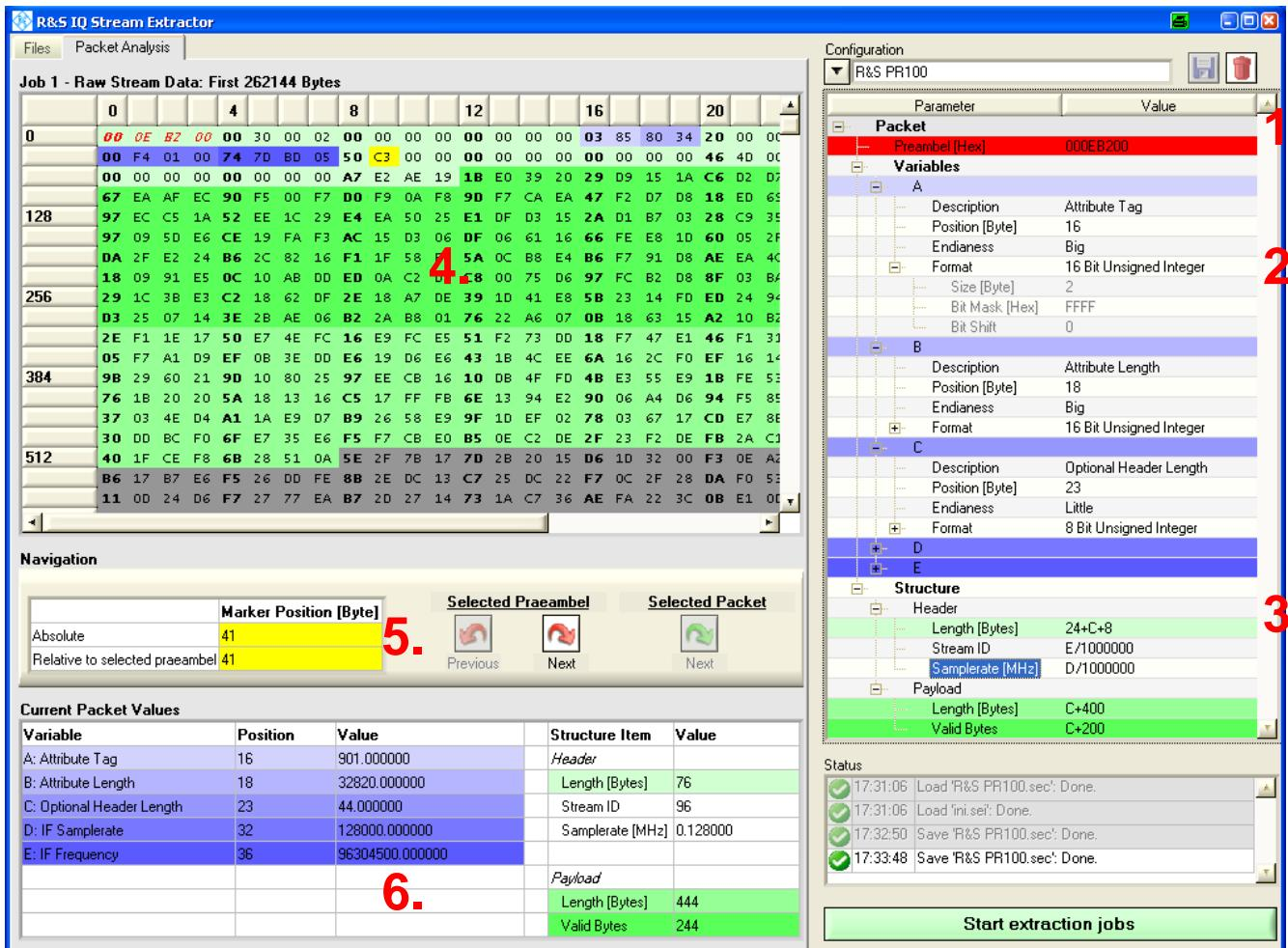
Fig. 10: Packet Analysis view.
