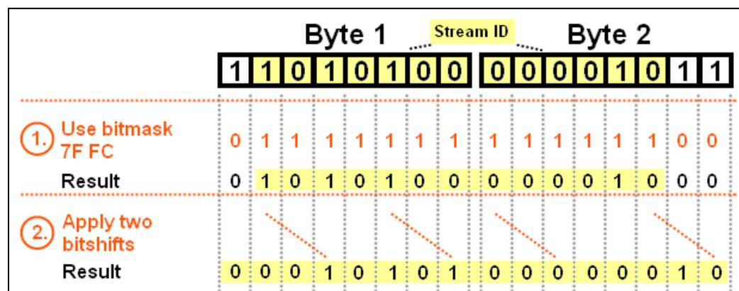
Fig. 9: Example of bit-level extraction of the "stream ID" header information.
