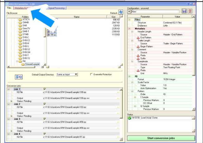
3 The first configuration parameters to be defined tell the software how to handle the metadata; i.e., the header and trailer of the input files. In this case, this structure was generated by R&S IQ Stream Extractor. The header and trailer preview in R&S IQ Converter make the necessary settings easily recognizable:
