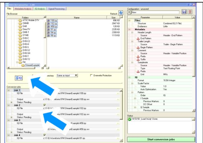
2c Click the "Metadata Analysis" tab in the upper left-hand corner to switch to the Metadata Analysis view.
