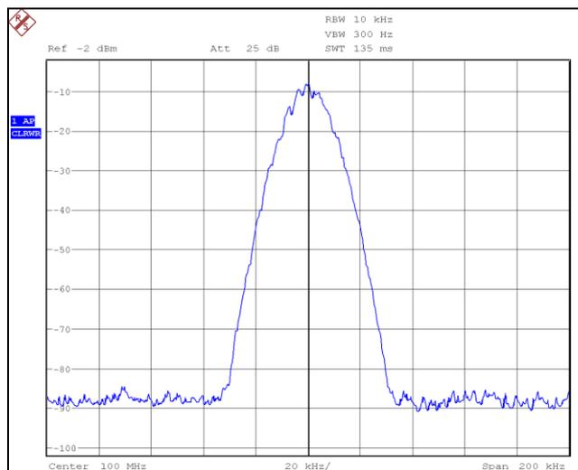
Fig. 12: Spectrum of "100.iqs.wv" waveform after reconstruction by the R&S SFU.
