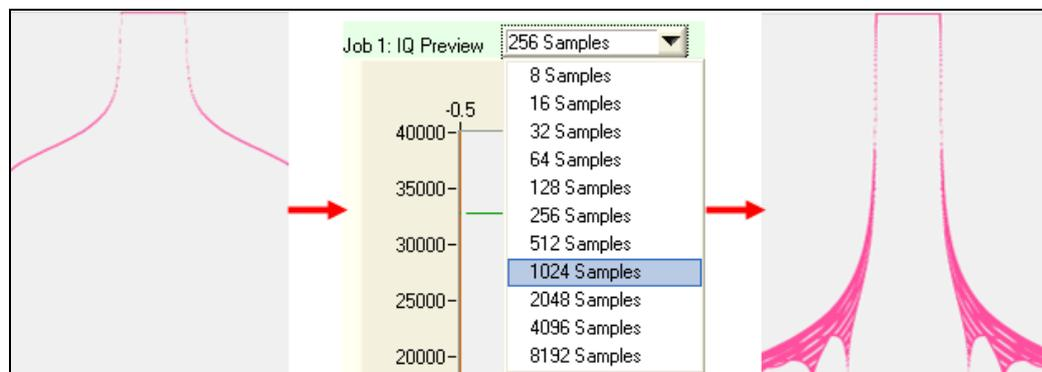
Fig. 13: Effect of the number of I/Q samples used for preview on the filter display.
