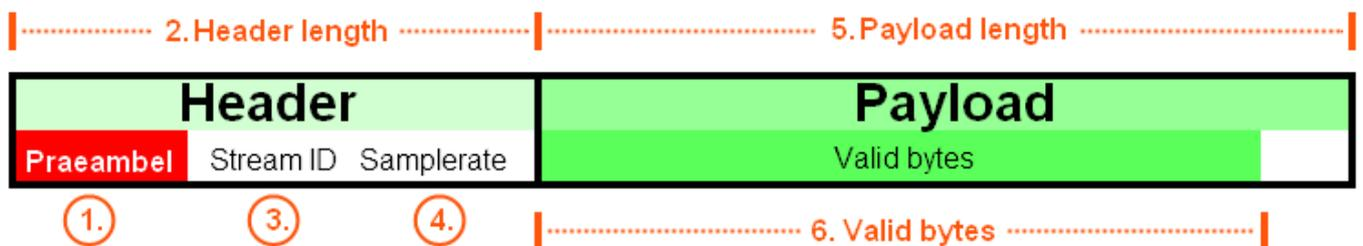
Fig. 8: R&S IQ Stream Extractor focuses on six main attributes per packet.
