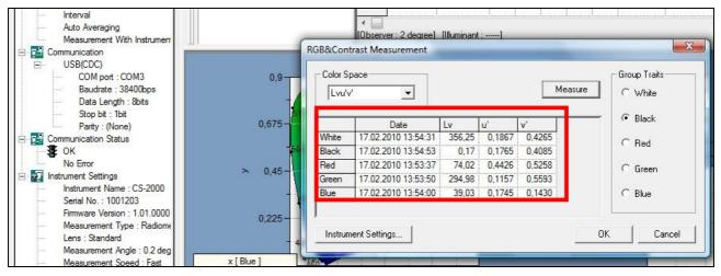
Figure 11: Completed measurement series for red, green, blue, black, and white
