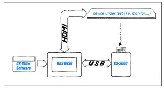
Figure 1: Typical test setup with the R&S<sup>®</sup>DVSG, Konica Minolta CS-2000 and Konica Minolta CS-S10w software
