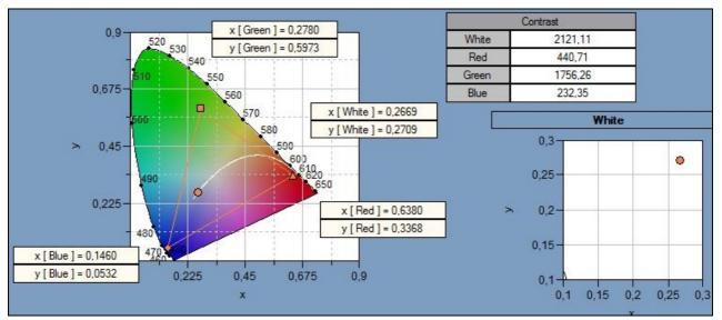
Figure 12: Measurement results display
