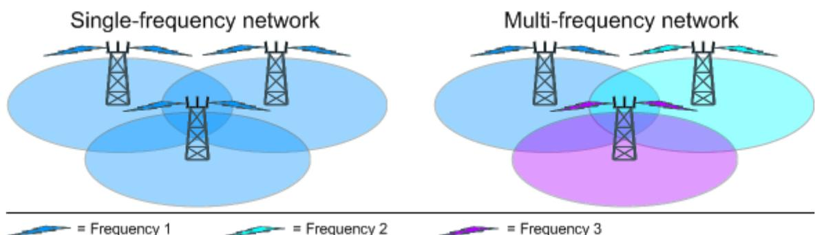
**Fig 1: Single-frequency and multi-frequency approach for a cell structured network**
