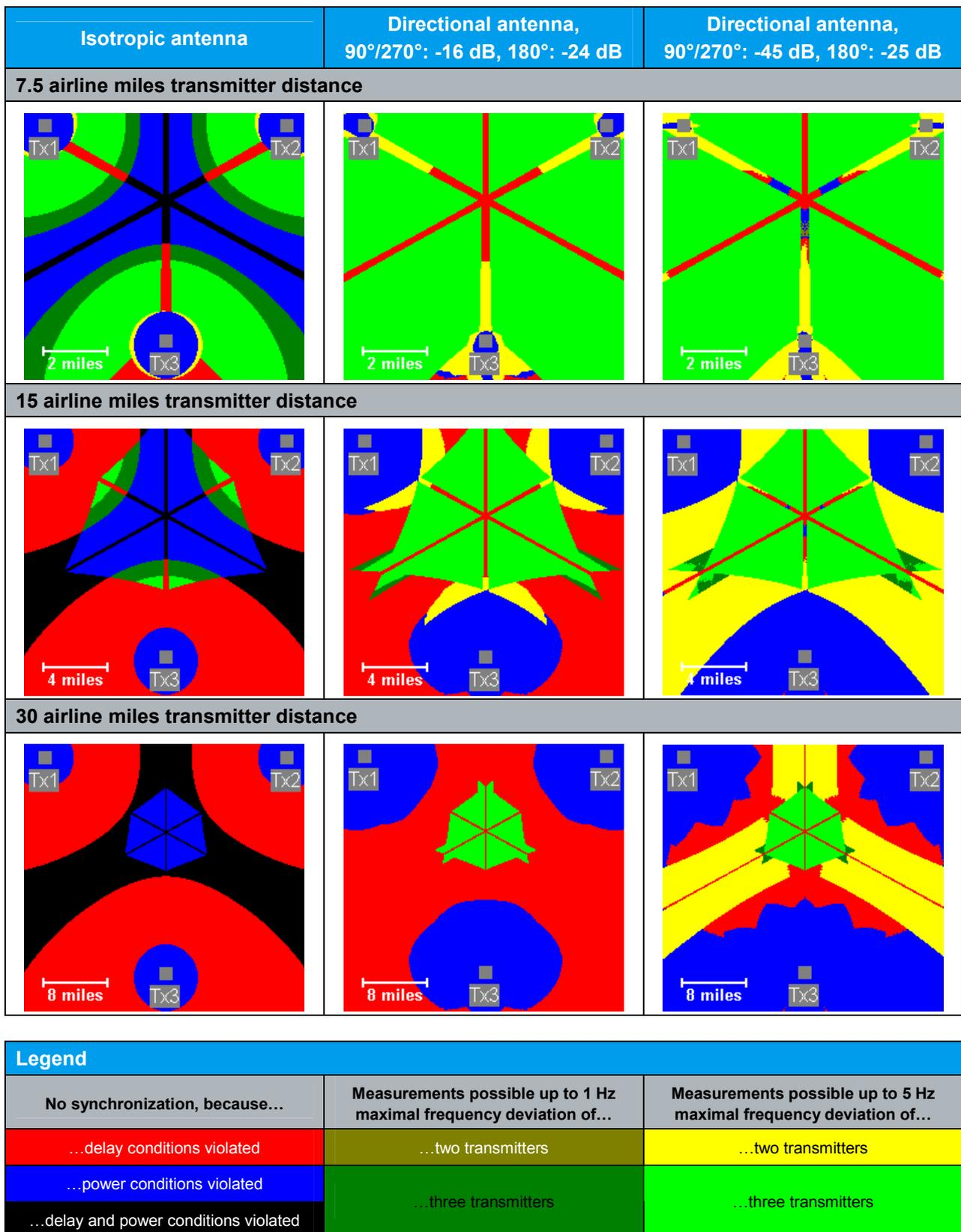
Table 1: Illustration of the ETL® ATSC (or ATSC Mobile DTV) SFN measurement range
