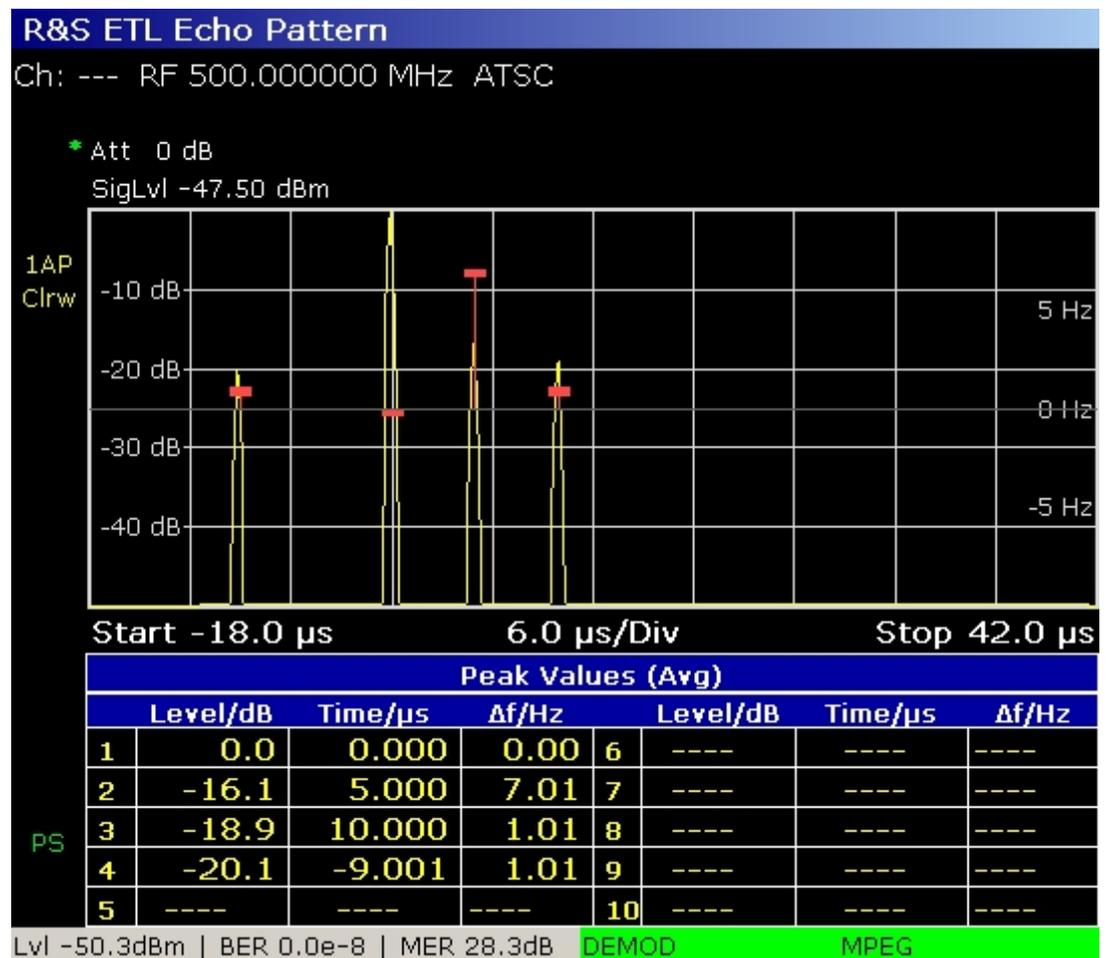
Fig 3: R&S®ETL ATSC (or ATSC Mobile DTV) SFN measurement screen
