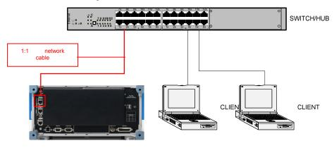
Fig. 15: Typical setup within a corporate network
