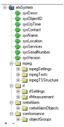
Fig. 11: MIB tree of the R&S<sup>®</sup>ETX-T
