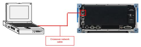
Fig. 13: Direct connection between measurement instrument and manager, using the R&S<sup>®</sup>DVM as an example
