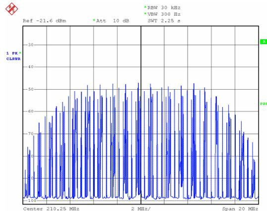
Fig. 12 Example: spectrum of impulsive noise at max. power
