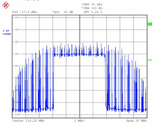
Fig. 15 Noise floor at 46 dB of DVB-T spectrum with superposed impulsive noise and extended dynamic range
