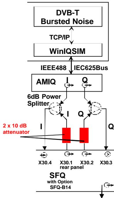
Fig. 14 Increasing the dynamic range of Impulsive Noise
