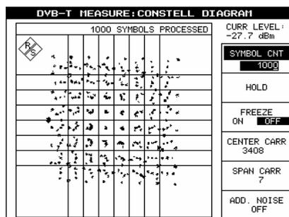
Fig. 4 Constellation diagram of 7 innermost carriers and central carrier in 8k mode.
