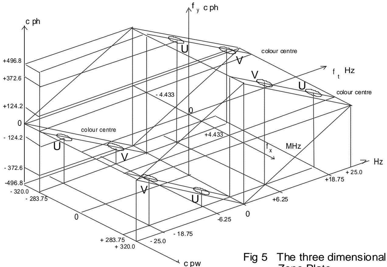
Fig 5 The three dimensional Zone Plate
