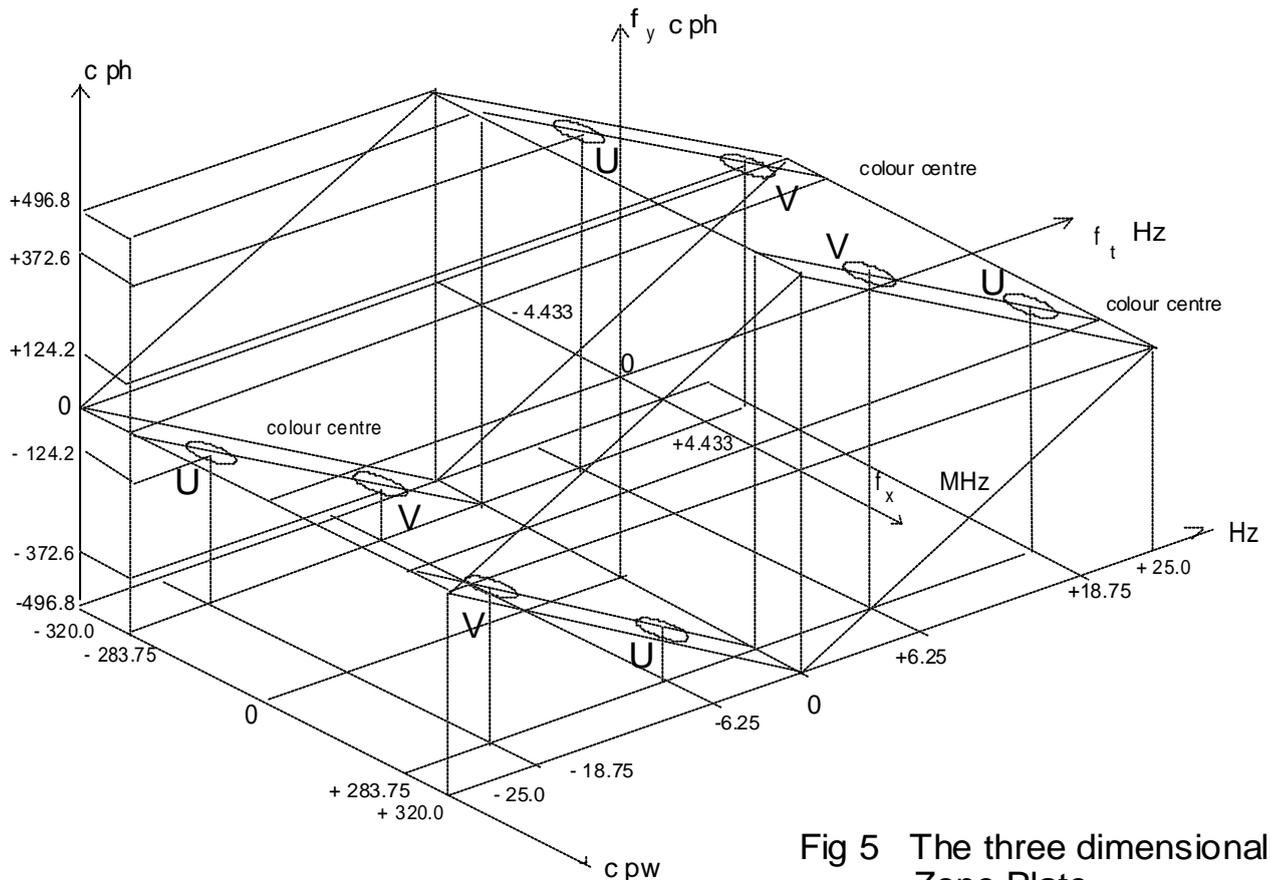
Fig 5 The three dimensional Zone Plate
