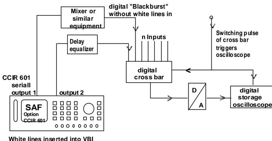
Fig. 7 Measurement of switching time at digital crossbar
