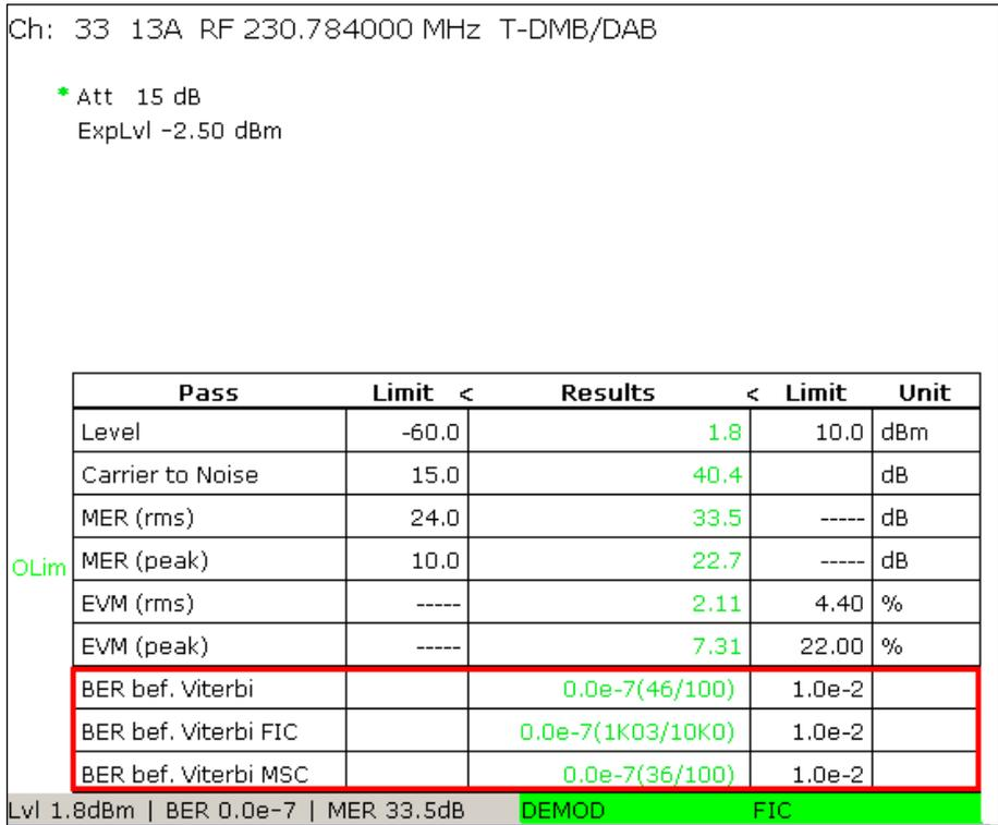
Fig. 13: TV/radio analyzer/receiver mode, MEAS→Modulation Analysis→Modulation Errors menu: BER before Viterbi
