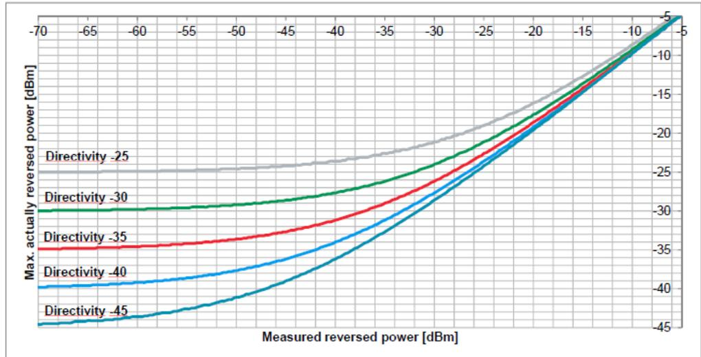
**Fig. 18: Maximum actually reversed power based on measured reverse power**
