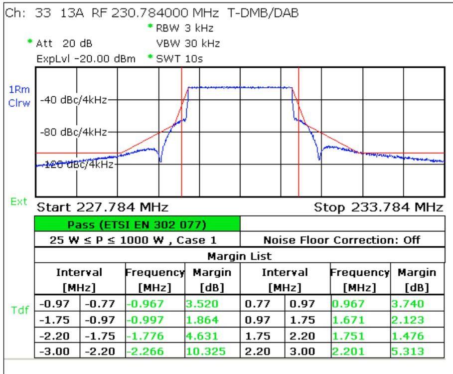
Fig. 8: TV/radio analyzer/receiver mode, MEAS→Spectrum→OutOfBandEmission menu: Measuring the shoulder attenuation and adjacent channel emissions
