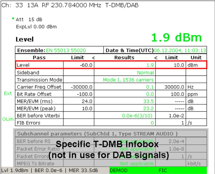
Fig. 2: TV/radio analyzer/receiver mode, MEAS→Overview menu: The level can be read in the first table row, in the status bar on the test screen or in the zoomed view (MEAS→Overview→Zoom)
