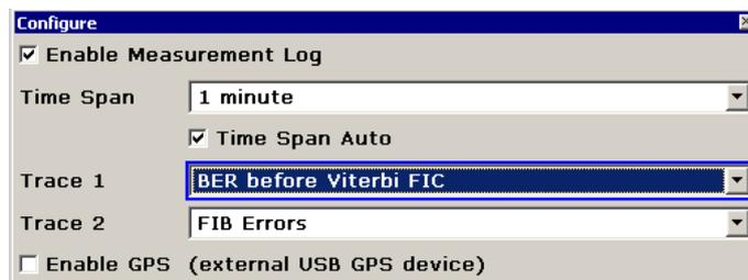
**Fig. 14:** TV/radio analyzer/receiver mode, MEAS→Measure Log→Configure menu: Configuration for the BER measurement
