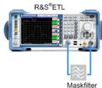
**Fig. 20: Connection setup to assess the frequency response of a mask filter.**
