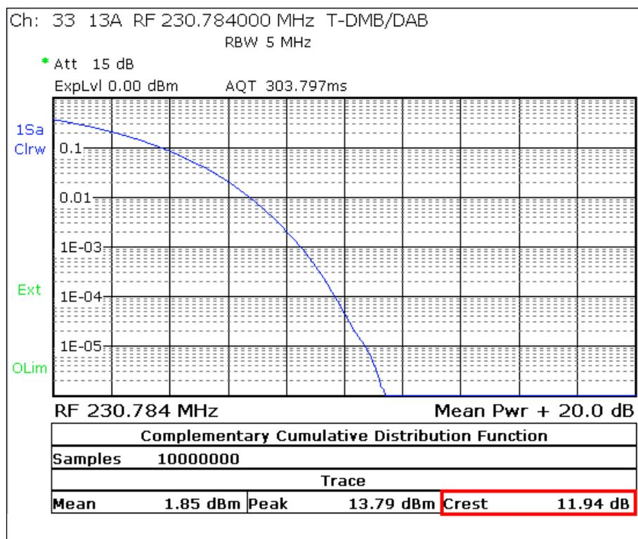
Fig. 4: TV/radio analyzer/receiver mode, MEAS→Modulation Analysis→CCDF menu: View with the calculated crest factor at the bottom right
