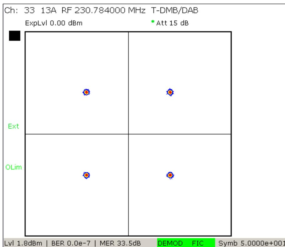
**Fig. 12:** TV/radio analyzer/receiver mode, MEAS→Modulation Analysis→Const Diagram menu: DAB constellation diagram (layer A, 64QAM)
