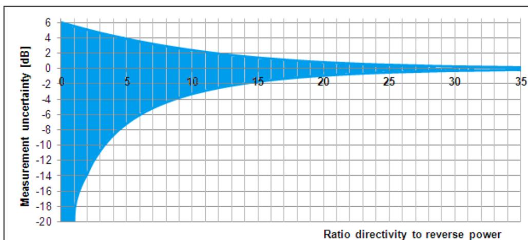
**Fig. 17:** Measurement uncertainty of the scalar measurement, dependent on the ratio of the directional coupler directivity to the reverse power (insertion loss of the directional coupler is disregarded).
