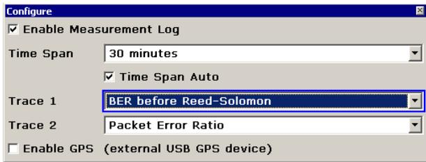
Fig. 13: TV/radio analyzer/receiver mode, MEAS→Measure Log→Configure menu: Configuration of the R&S®ETL measurement log for the BER measurement.
