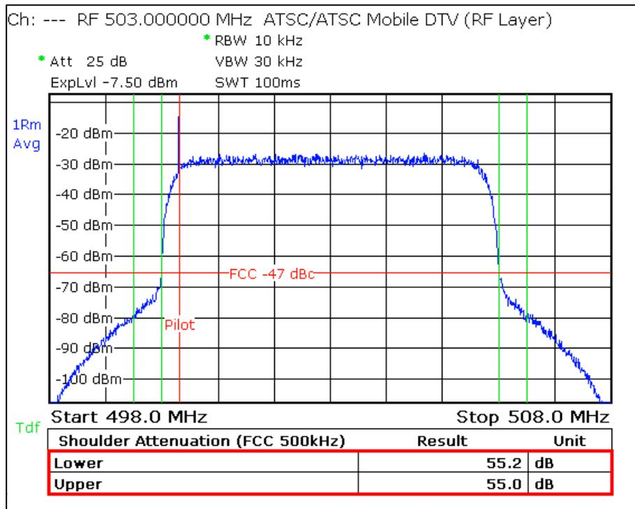
Fig. 7: TV/radio analyzer/receiver mode, MEAS→Spectrum→Shoulder Atten menu: Measuring the shoulder attenuation in accordance with FCC.
