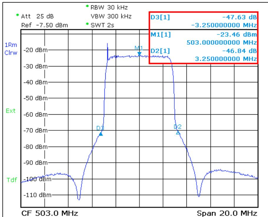
Fig. 6: Spectrum analyzer mode: Measuring the shoulder attenuation at +/- 3.25 MHz using the cursor method with active transducer file in the 6 MHz ATSC channel.
