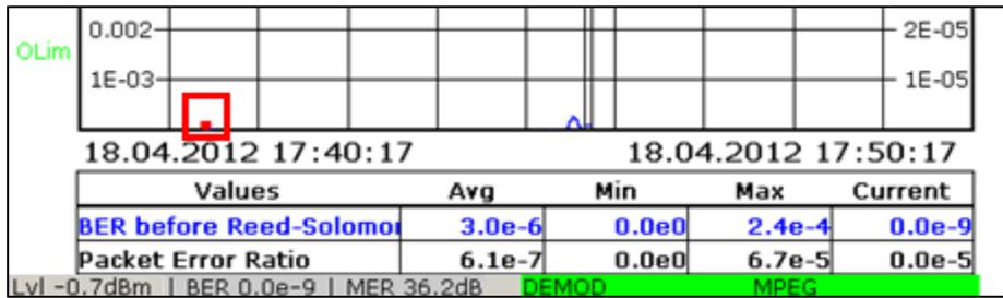
Fig. 14: TV/radio analyzer/receiver mode, MEAS→Measure Log menu: BER measurement with the measurement log. Red markers directly above the time axis (here in the 2nd time segment) indicate a loss of synchronization. In this case, the BER measurement is invalid.
