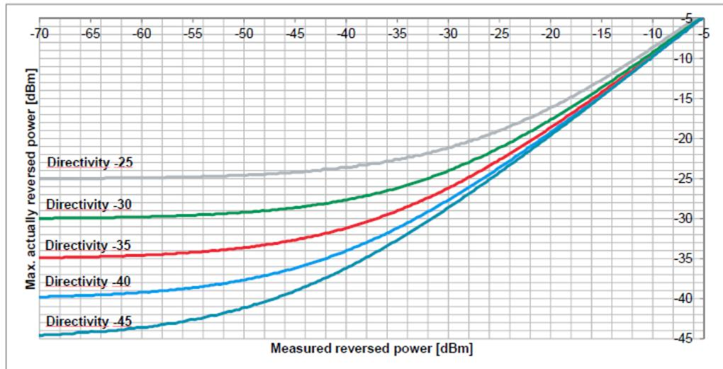
**Fig. 18: Maximum actually reversed power based on measured reverse power.**
