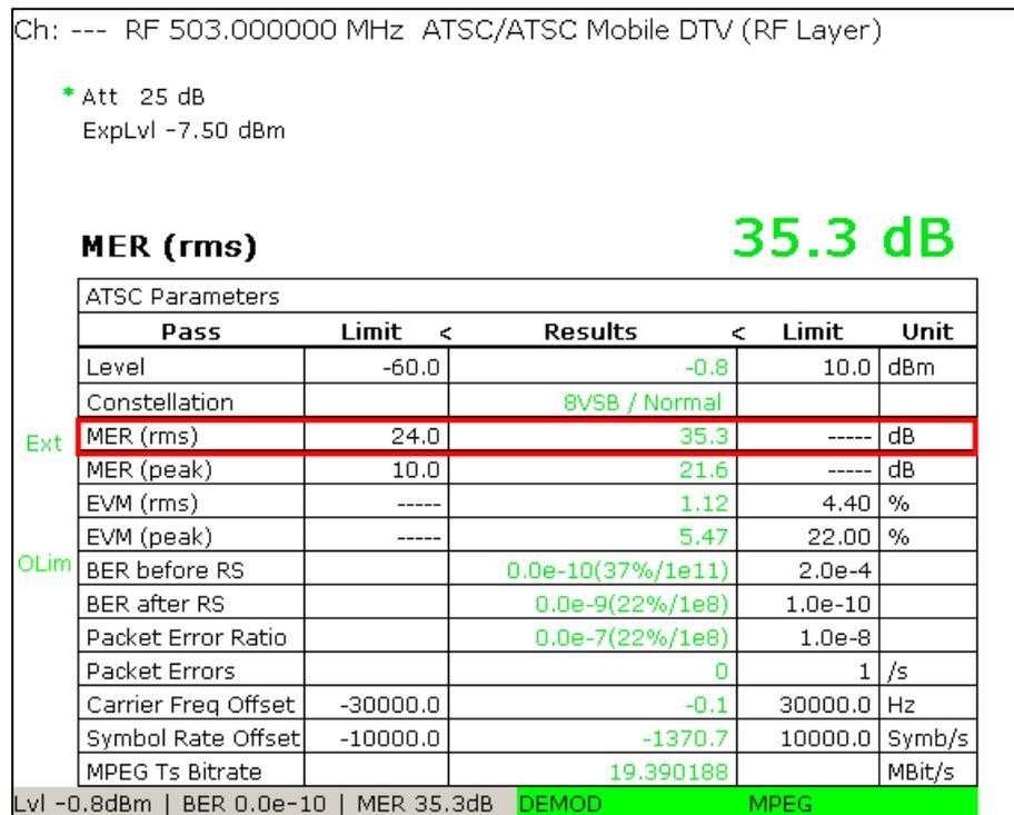
**Fig. 11: TV/radio analyzer/receivermode, MEAS→Overview menu: The MER can be read in the third table row, in the status bar on the test screen or in the zoomed view (MEAS→Overview→Zoom).**
