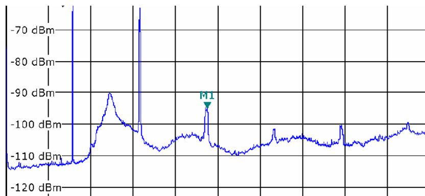
**Fig. 9: Spectrum analyzer mode: Useful channel attenuated using the highpass filter; the harmonics, which can be assessed using the marker function, are clearly visible.**
