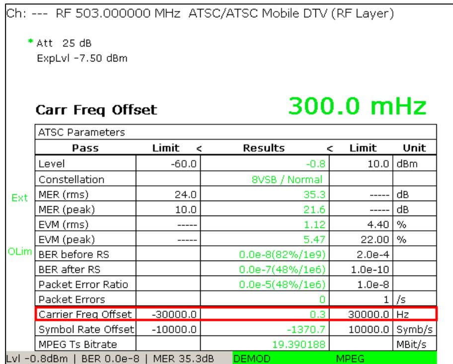
Fig. 10: TV/radio analyzer/receiver mode, MEAS→Overview menu: The frequency accuracy can be read in the 11th table row, as well as in the zoomed view (MEAS→Overview→Zoom).
