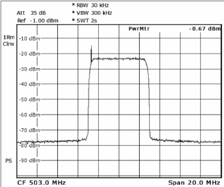
Fig. 3: Spectrum analyzer mode: ATSC spectrum with integrated reading from the power sensor displayed at the top right.
