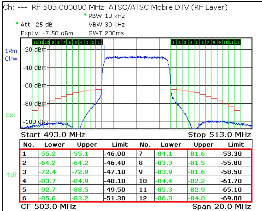
Fig. 8: TV/radio analyzer/receiver mode, MEAS→Spectrum→OutOfBandEmission menu: Adjacent channel emissions checked with stringent mask.
