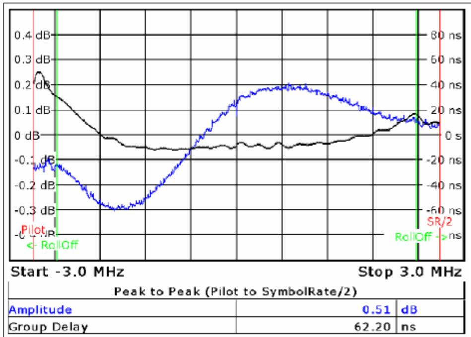
Fig. 5: TV/radio analyzer/receiver mode, MEAS→Channel Analysis→Amplitude & Group Delay menu: Amplitude frequency response and group delay after an uncompensated mask filter.
