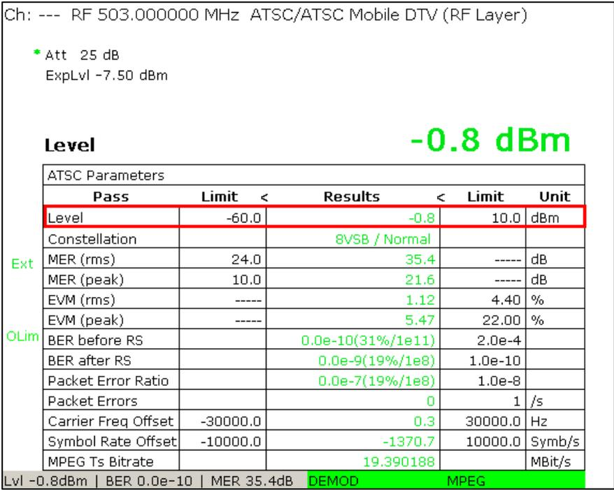
Fig. 2: TV/radio analyzer/receivermode, MEAS→Overview menu: The level can be read in the first table row, in the status bar on the test screen or in the zoomed view (MEAS→Overview→Zoom).
