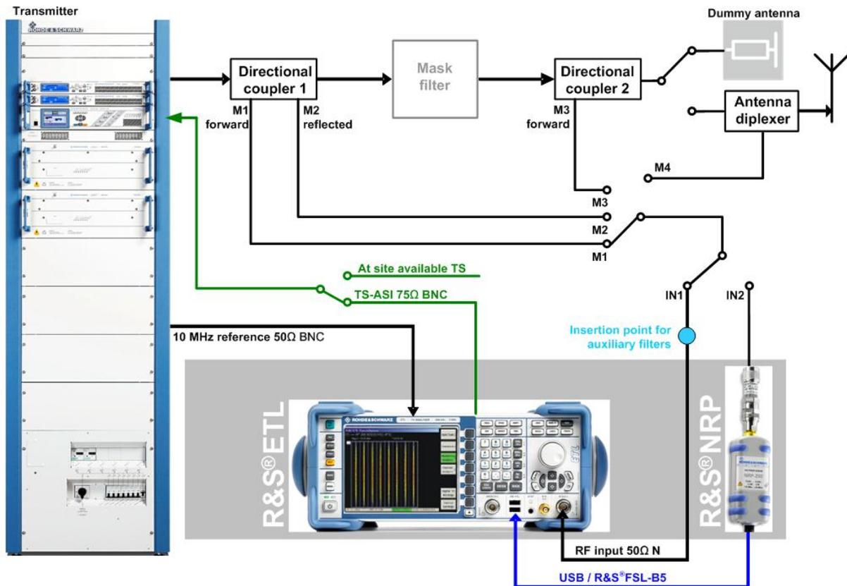
**Fig. 1:** Test setup for transmitter acceptance measurements.
