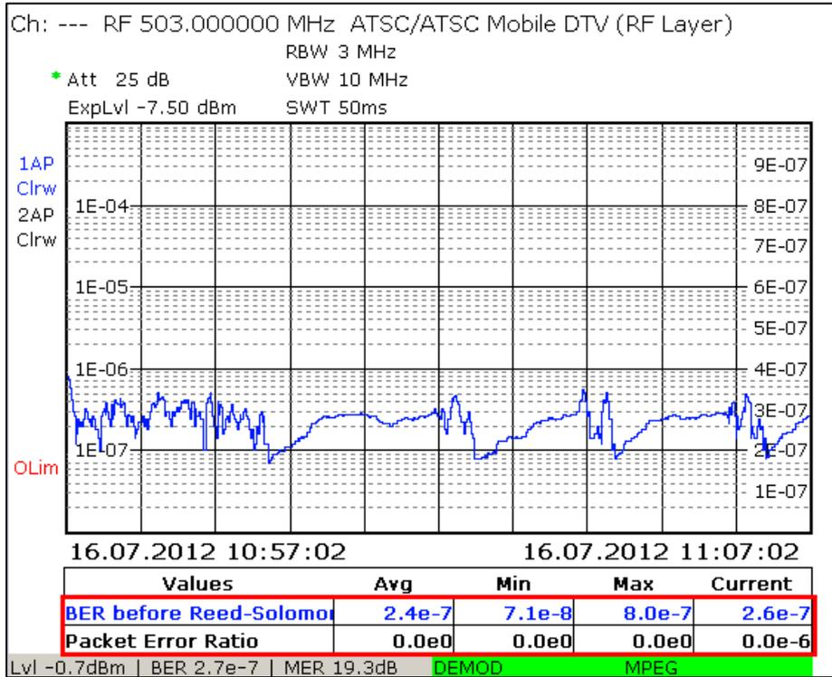
Fig. 15: TV/radio analyzer/receiver mode, MEAS→Measure Log menu: Valid BER measurement.
