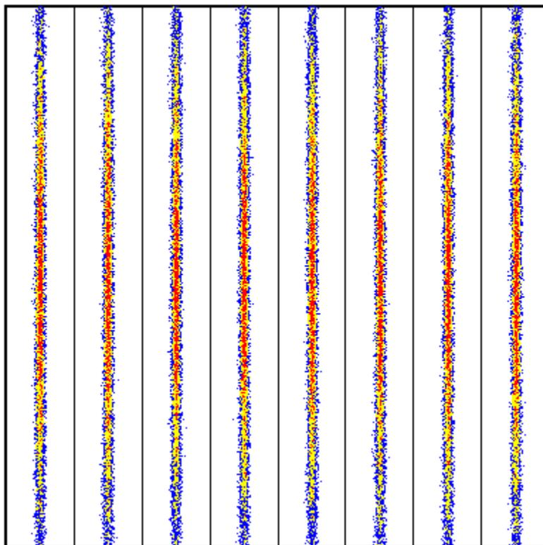
Fig. 12: TV/radio analyzer/receivermode, MEAS→Modulation Analysis→Const Diagram menu: ATSC constellation diagram with a MER of 36 dB.
