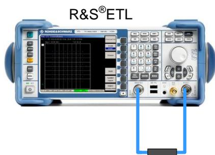
**Fig. 19: Connection setup to regulate the cable.**
