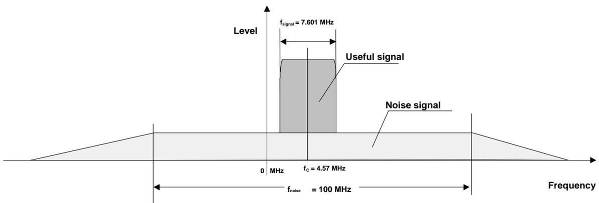
Fig. 8 Non-physical spectrum and broadband noise spectrum
