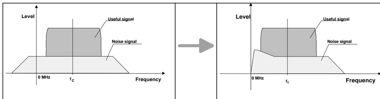
Fig. 3 Frequency reflection about 0 Hz
