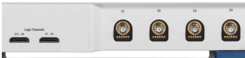
Figure 2. Many oscilloscopes have a tradeoff between the number of channels that are enabled, and the maximum memory available per channel.
