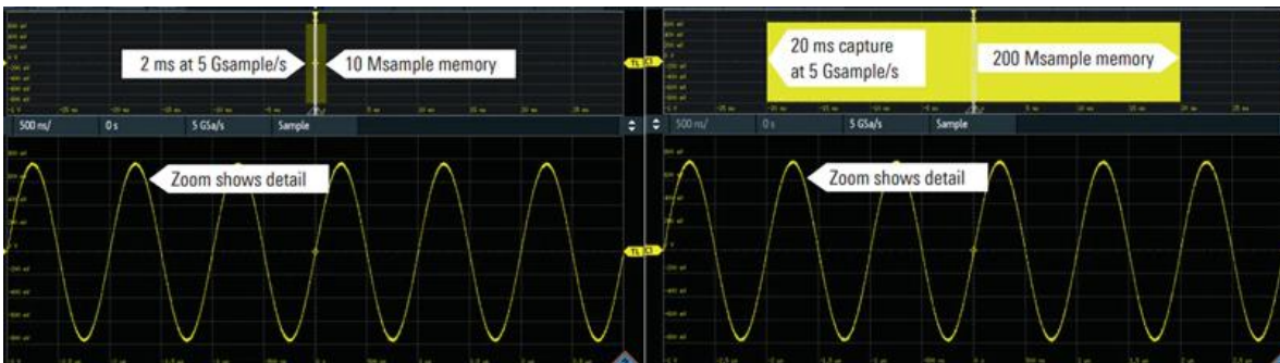
Figure 3. More memory means an oscilloscope can capture more time at a given sample rate.
