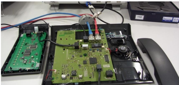
Fig. 4-7: Test setup for EMI debugging on a modern IP telephone. In this example, a current probe is connected to measure the common-mode RFI current on the connected lines.
