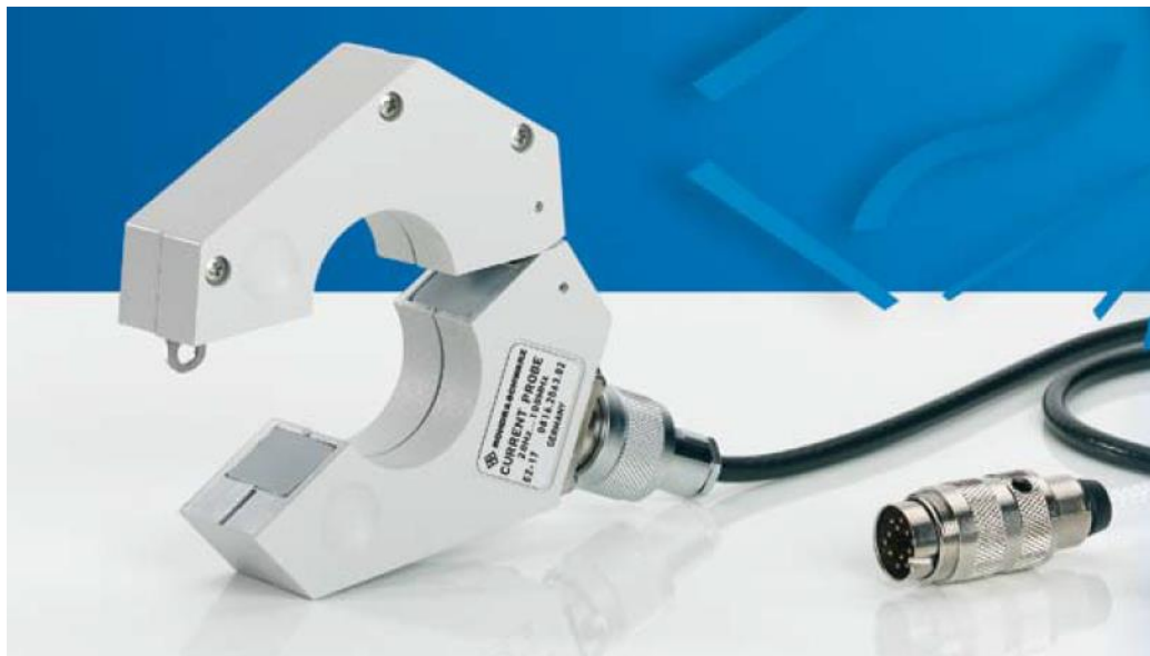
Fig. 3-3: The R&S®EZ-17 current probe with 10 dB \Omega transfer impedance (model 02) or 17 dB \Omega transfer impedance (model 03) and 20 Hz to 100 MHz bandwidth is a good example of a device suitable for measuring RFI currents. The large inner diameter of 30 mm allows measurements on cable bundles.
