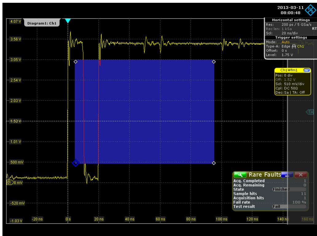
Figure 21 – Applied MASK Test (stop on fail)
