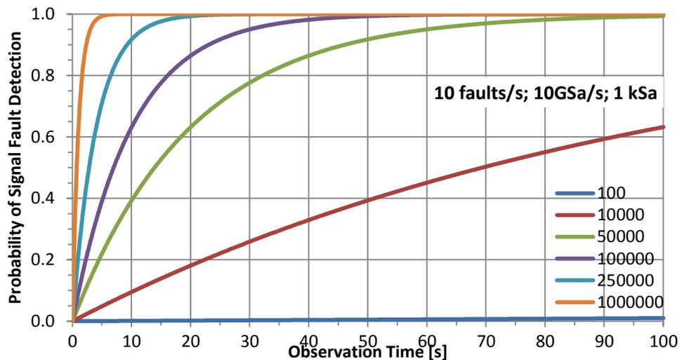
Figure 10 – Fault Detection Probability
