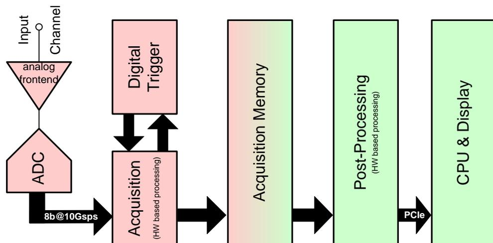
Figure 1 – R&S®RTO Oscilloscope Block Diagram
