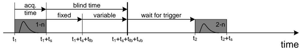
Figure 9 – Acquisition and Post-Processing Cycle of a Digital Oscilloscope
