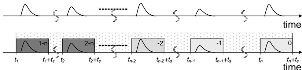
Figure 7 – Acquisition of a Pulse Train with Single or Multiple Acquisitions
