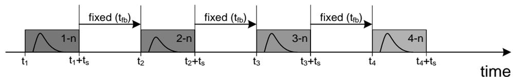
Figure 12 – Ultra-Segmentation Cycle of a Digital Oscilloscope
