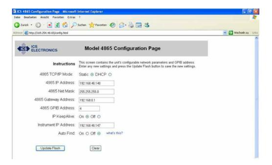
If this configuration is saved by clicking 'Update Flash', the ICS-4865 welcome page is again called up and the following screen appears. The set 'Instrument IP Address' is not shown, but internally this instrument address is still set and still functions.
