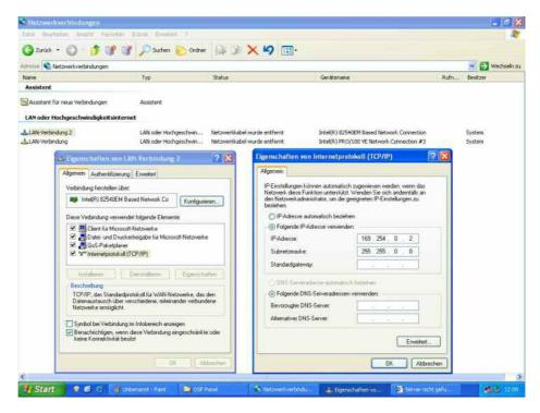
Connect the ICS-4865 to the PC's network card with a **crossover Ethernet cable**. Then turn on the ICS-4865 and wait until it finishes booting up (approx. 20 seconds). In a web browser, enter the IP address <a href="http://169.254.48.65">http://169.254.48.65</a>.
