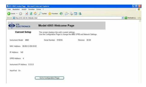
The ICS-4865 can also be configured so that instead of looking for a connected instrument in its own address range, it only looks for a set IP address and expects to find a VXI-11.3 instrument there (e.g. the R&S®OSP) (see the following screenshot).
