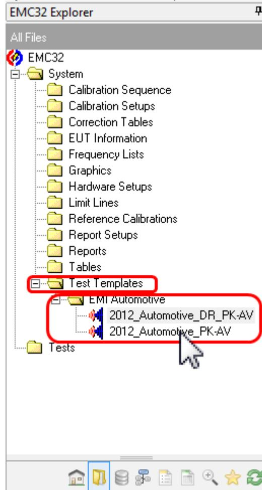
**Figure 7: A mouse click on an existing file open the template editor with this EMI Automotive Test Template**
