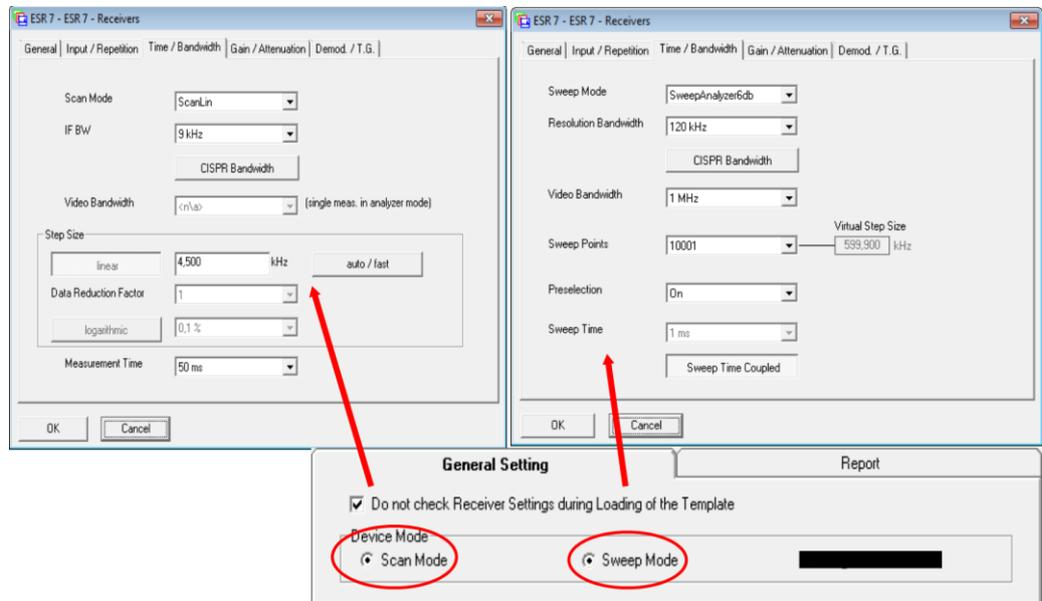
Figure 20: Receiver settings according to the chosen mode
