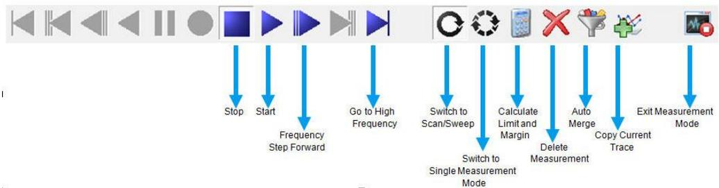
Figure 39: Test Control Toolbar before start
