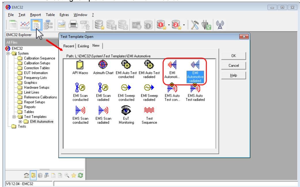
Figure 9: Generation a new template via icon "Test Template new/open ..."
