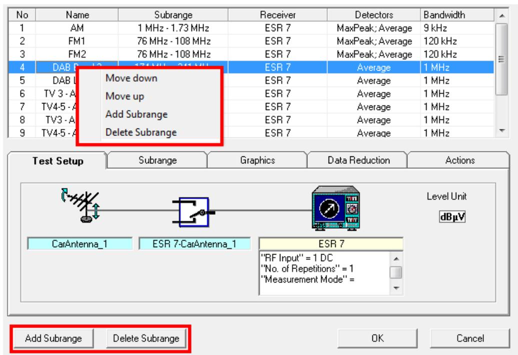
Figure 15: The pop-up menu and the two buttons allow basic changes
