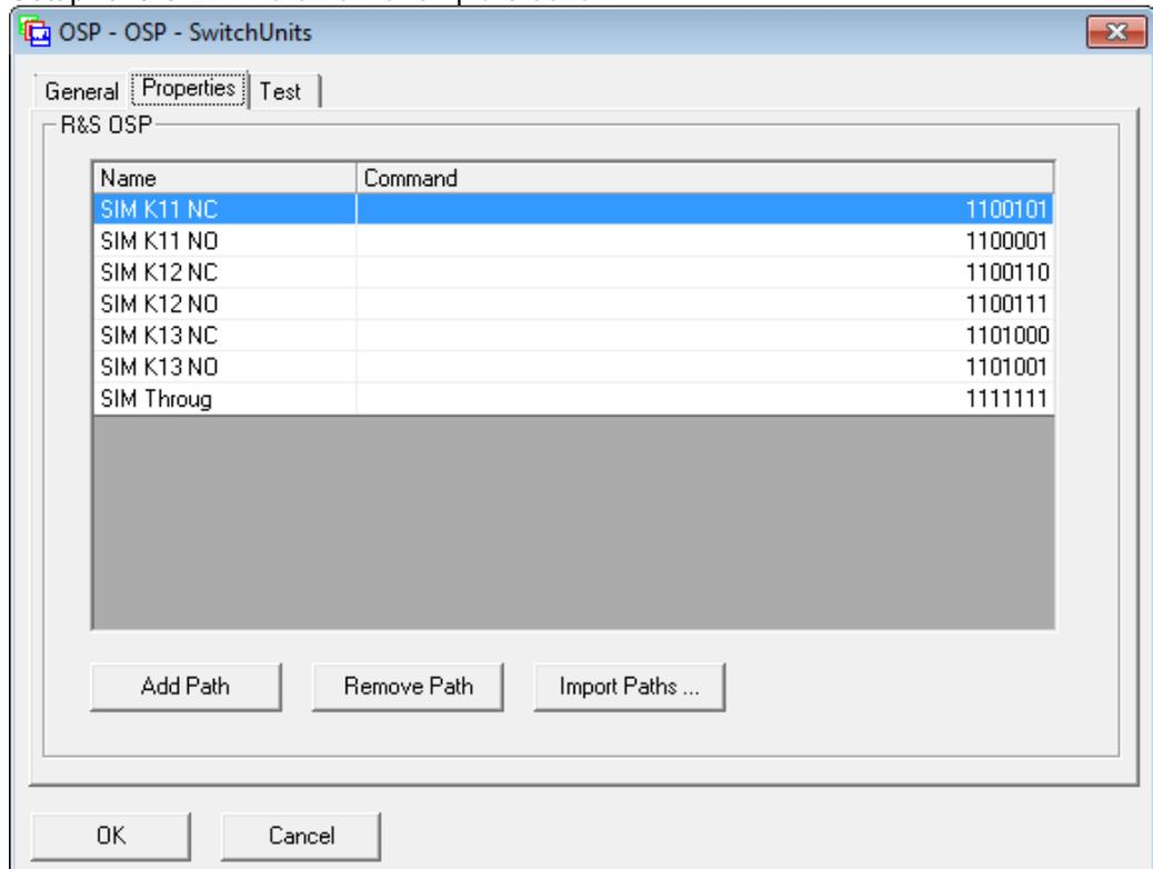
Figure 6: OSP with settings for paths as an example for a switch unit
