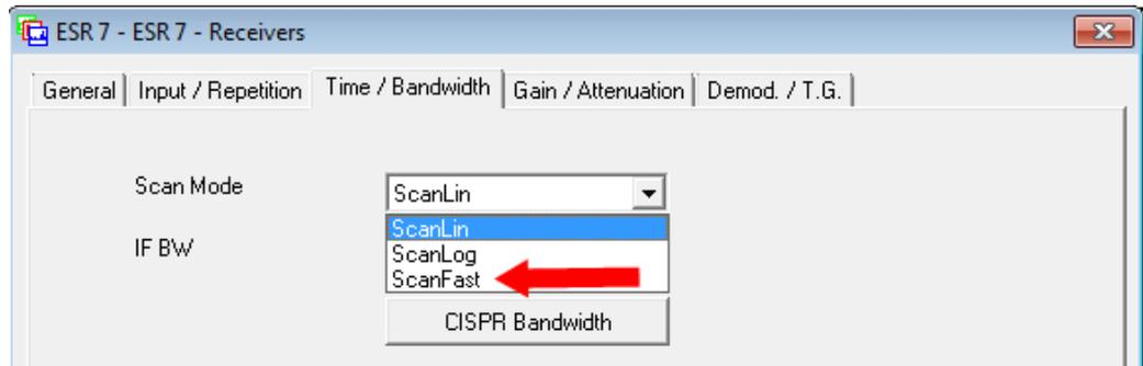
**Figure 22: Switching the Test Receiver to Time Domain Scan (TD-Scan: FFT Mode) use ScanFast as Scan Mode**
