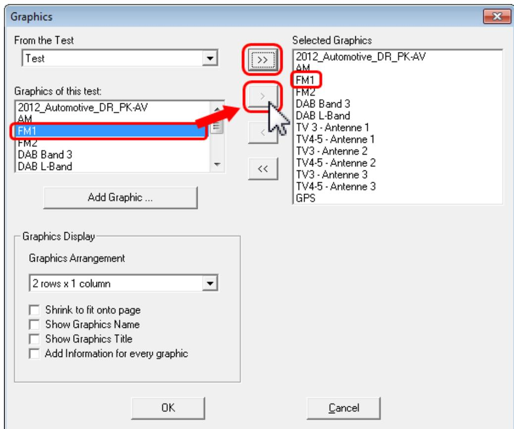
Figure 46: The properties allow selecting single graphics as well as all graphics by click on upper button
