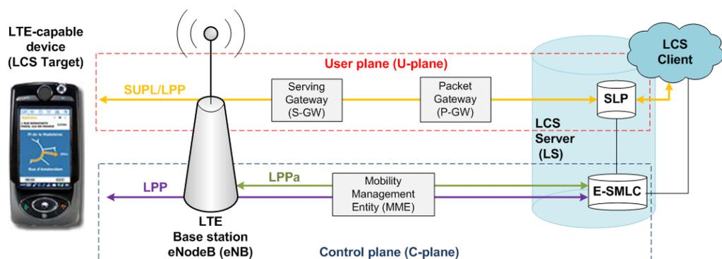
Figure 9: E-UTRA positioning network architecture
