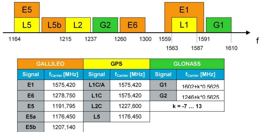
Figure 1: Frequencies being used by GPS, GALLILEO and GLONASS
