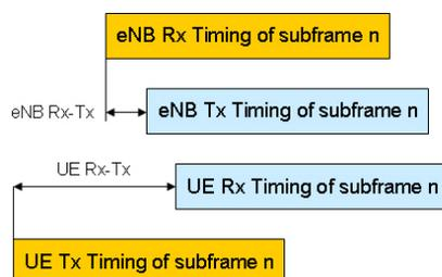
Figure 14: eNB and UE receive-transmit timing difference
