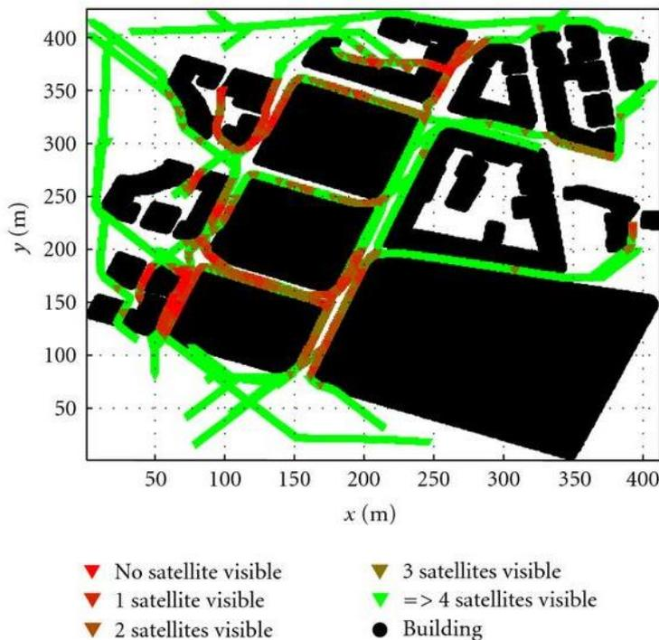
Figure 2: Number of visible GPS satellites in a city centre [4]
