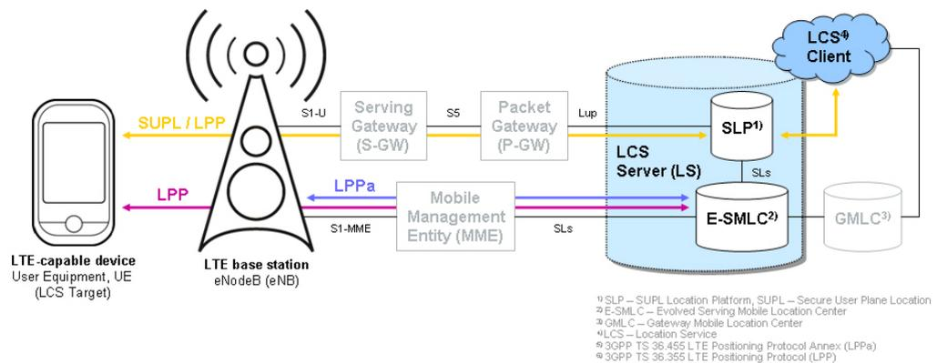
**Figure 6: E-UTRA positioning network architecture**
