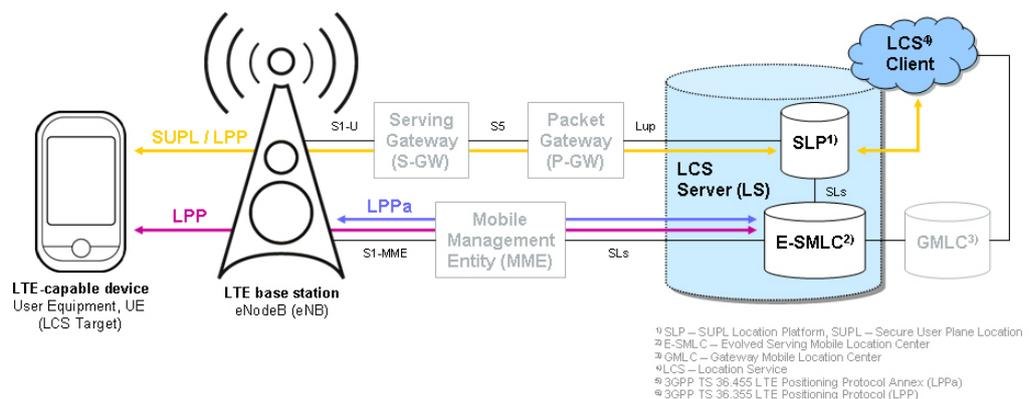
**Figure 6: E-UTRA positioning network architecture**
