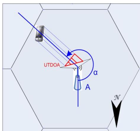
Figure 15: Angle-of-Arrival (AoA) measurement
