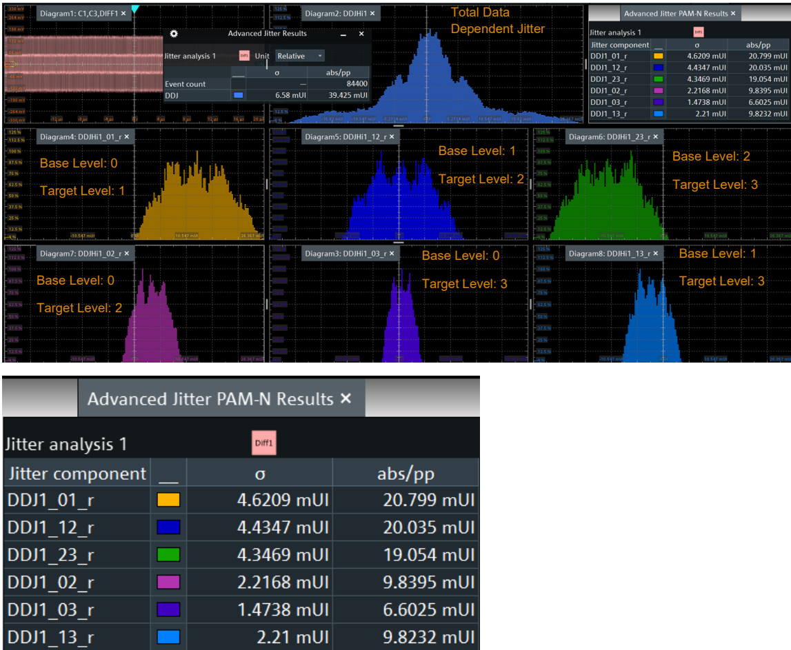
Figure 11: Transition-Level Jitter Decomposition – PAM4
