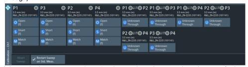
It is required to measure at least 3 unknown through connections, however further measured connections will increase the accuracy.
