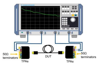
To avoid confusion, throughout the document the test fixtures are referred to by their orientation in this diagram (left, right), or simply by an "L" or "R" subscript when appropriate.
