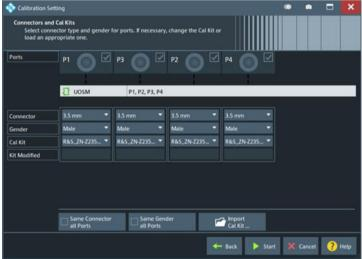
5. Start calibration and connect all required calibration standards (open, short, match and unknown through).
