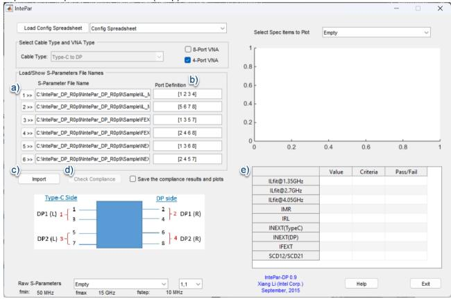
a) Load in S-parameter Files for DUT
