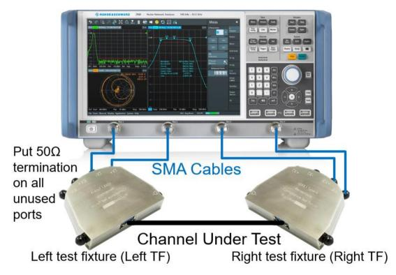
Equipment needed for testing is listed in Error! Reference source not found.. Below is an example setup u sing the R&S<sup>®</sup>ZNB20.
