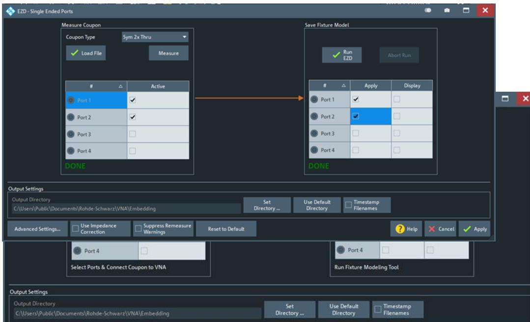
All pop-up dialogs should be closed, and the main firmware interface is present. The test fixture file for the left-side, top-layer fixture has been created.
