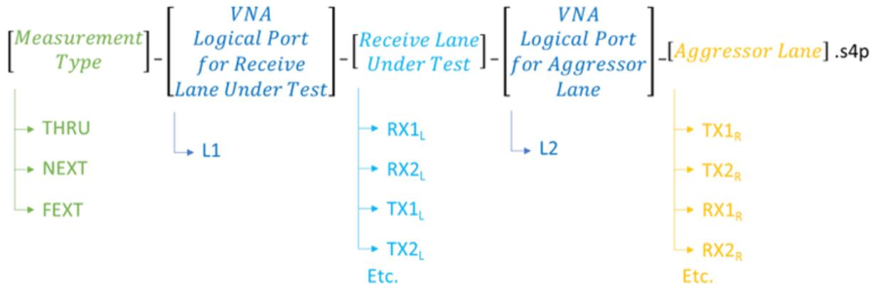
For example, when collecting the touchstone file which includes the differential insertion loss and differential return loss of TX1, or the TX1 "Thru" file, the file name would be:
