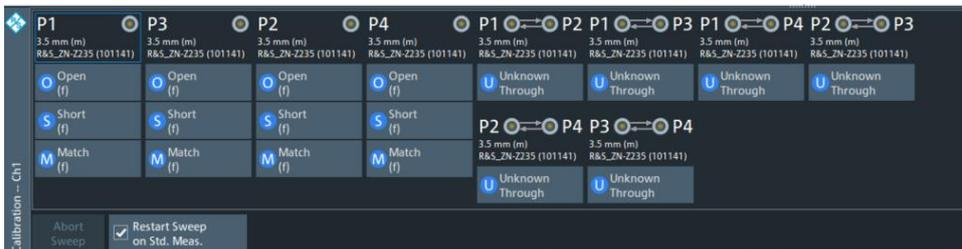
It is required to measure at least 3 unknown through connections, however further measured connections will increase the accuracy.
