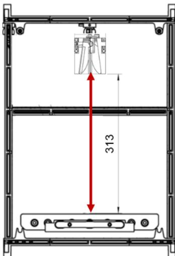
Figure 3-34 Distance between drawer table position 1 and Vivaldi antenna (313 mm)
