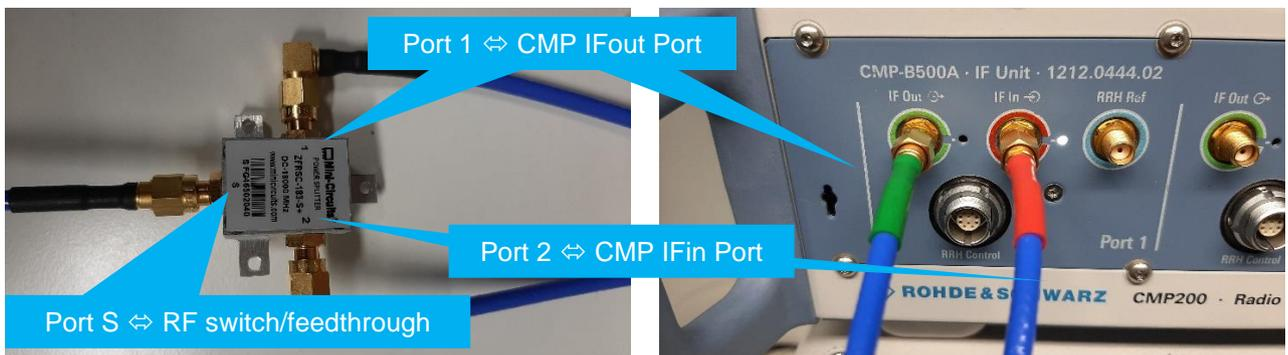
Figure 3-31 Cabling of power splitter and its connections to RF ports of CMP200
