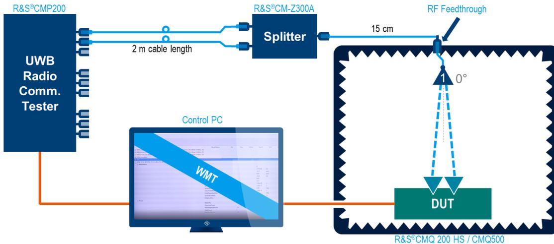
Figure 3-2 Block diagram of system variant 1: UWB OTA testing environment with RF feedthrough for Tx, Rx and ToF measurement (single Vivaldi antenna)
