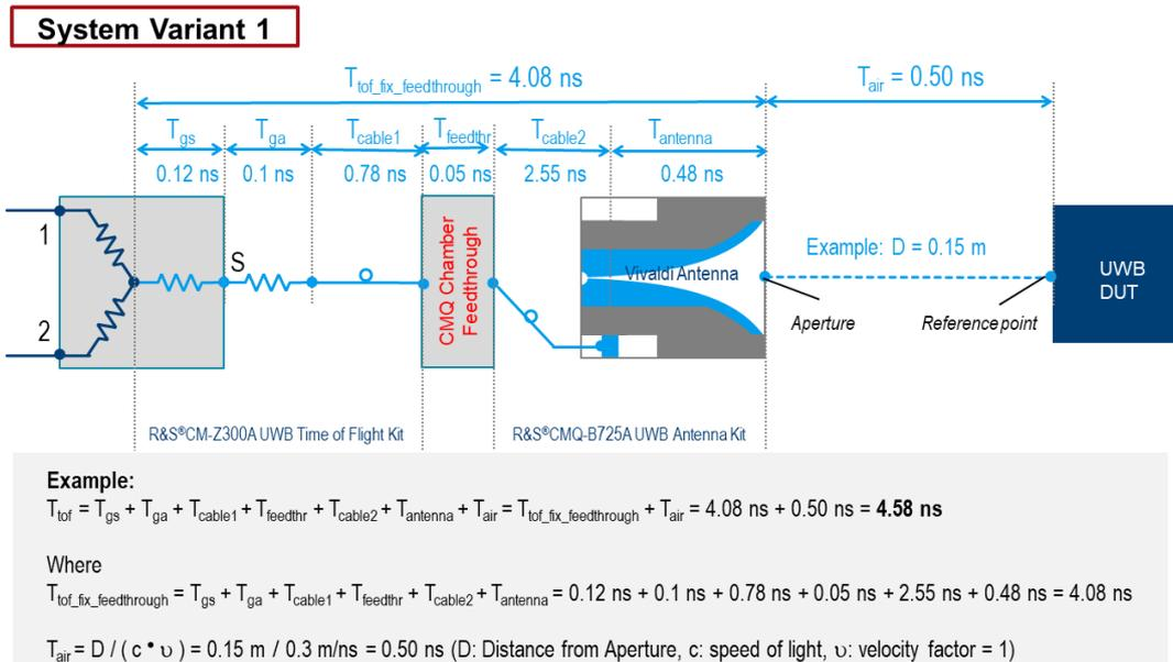
Figure 3-52 An example of ToF calculation for RF feedthrough (system variant 1) with 0.15 meter OTA distance
