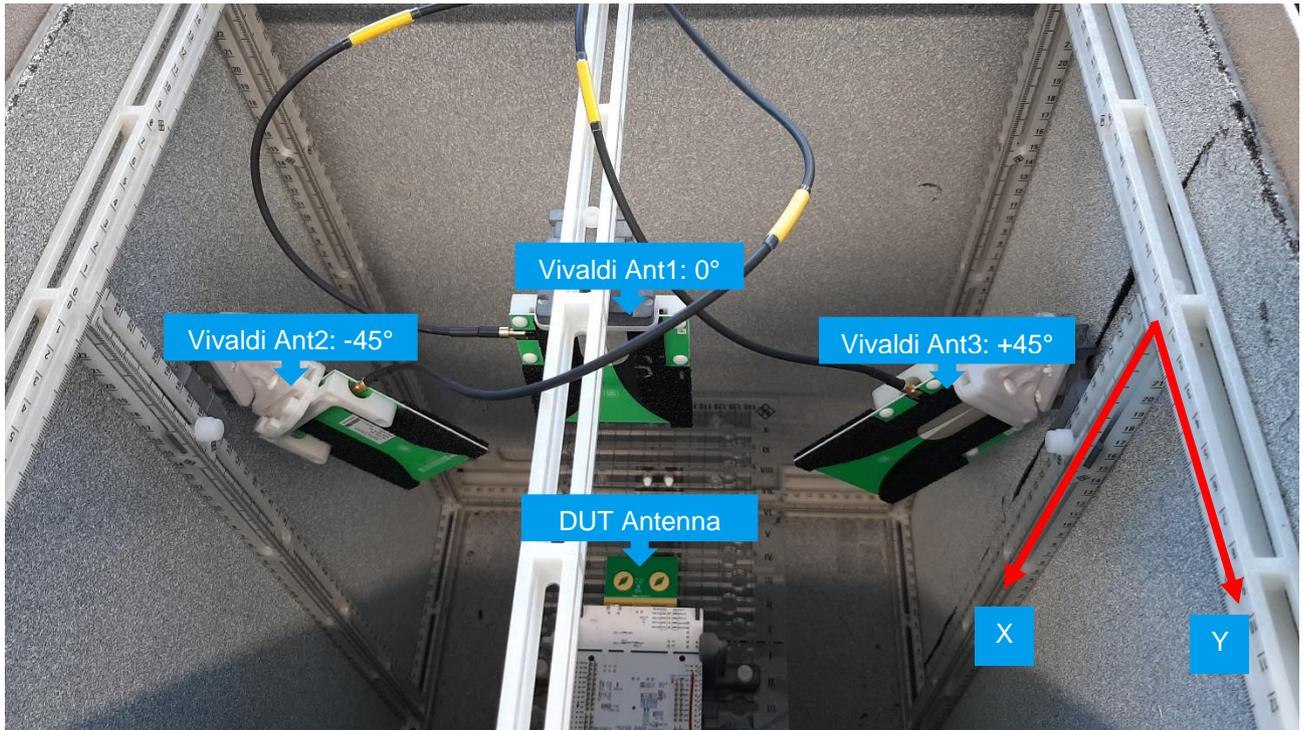
Figure 3-35 Positioning of UWB DUT and measurement antennas (Vivaldi) in a CMQ200 chamber for UWB AoA testing
