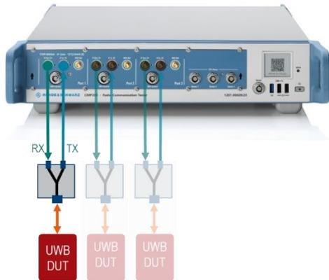
Figure 3-5 R&S CMP200 with multiple switchable ports
