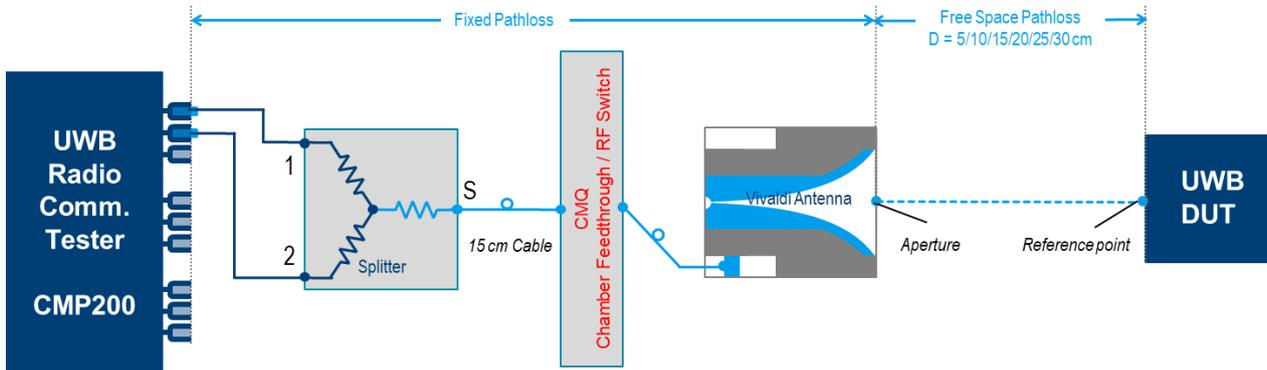
Figure 3-45 Sketch of overall pathloss consists of fixed insertion loss on the signal path plus distance and frequency dependent free space pathloss
