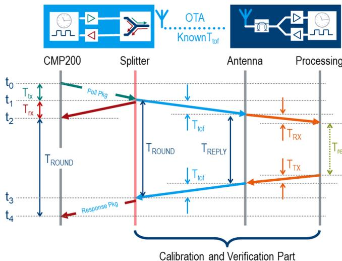
Figure 3-51 Principle of antenna delay calibration and ToF verification (cf. Table 3-4)
