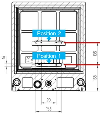
Figure 3-33 Two fixed positions in CMQ200/CMQ500 chamber with drawer table layout
