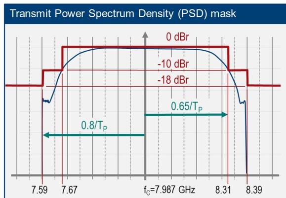
Figure 3-61 Transmit spectrum mask for channel 9
