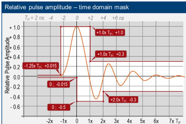
Figure 3-60 Time domain mask of HRP UWB PHY pulse with 2 ns  $T_p$
