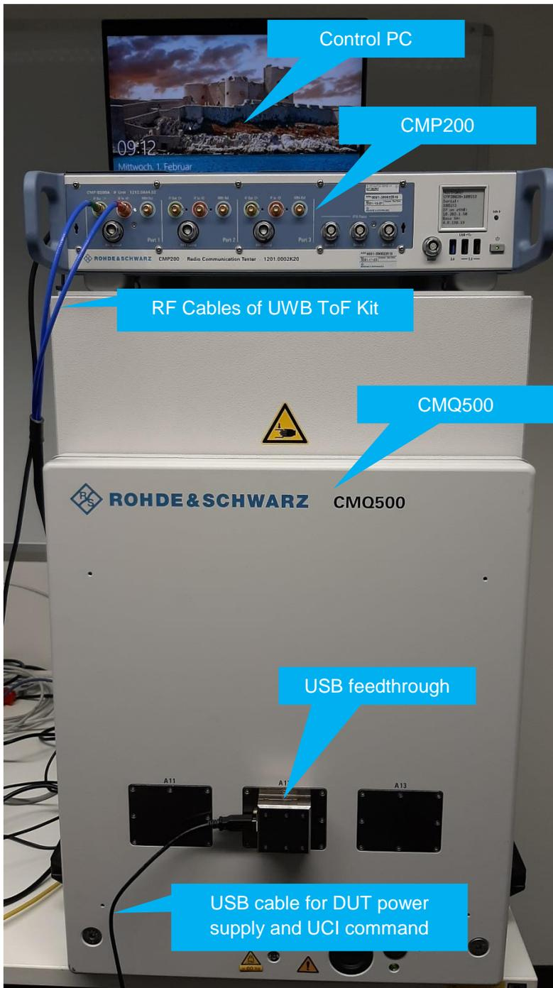
Figure 3-29 Front view of setup with cabling
