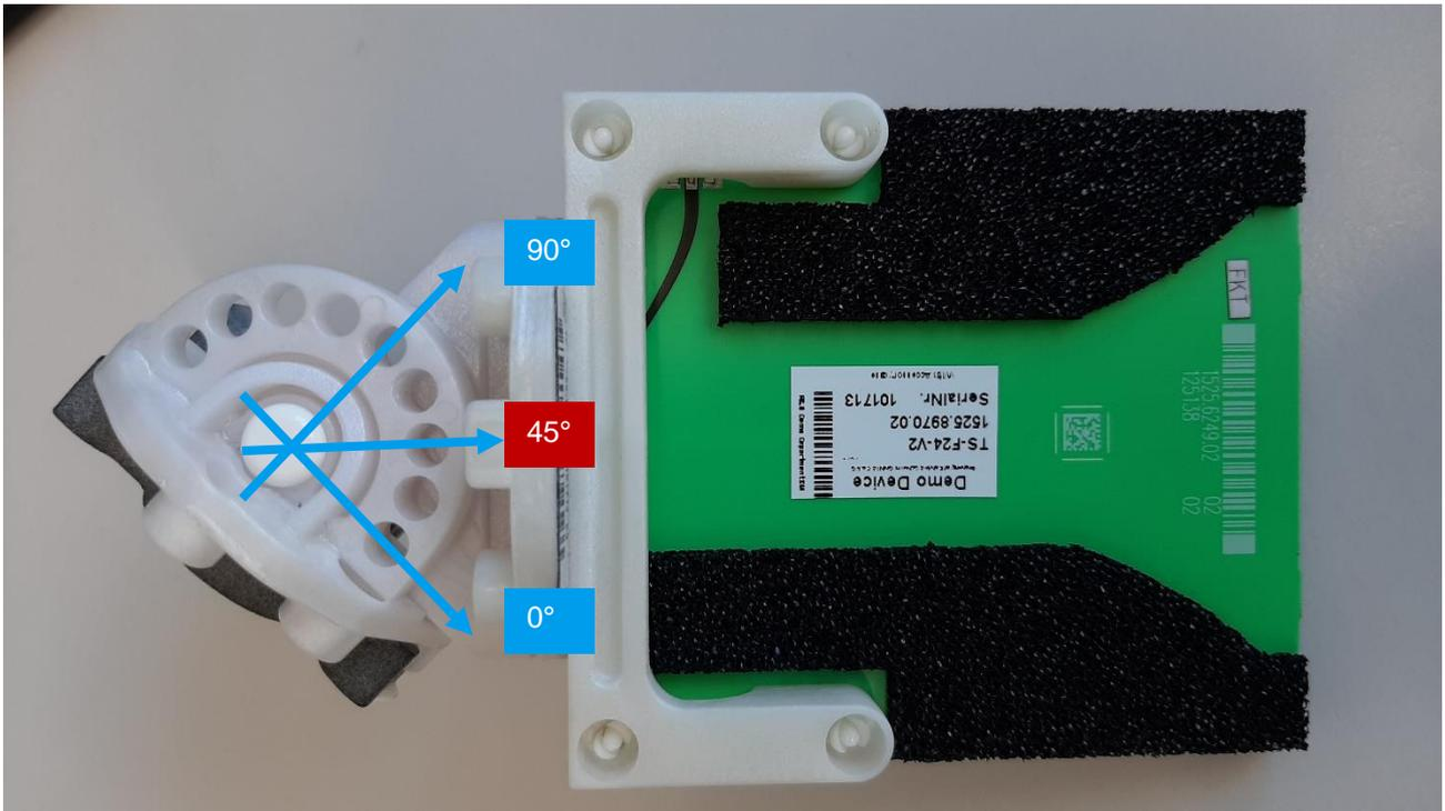
Figure 3-36 Angle adjustment of the Vivaldi antenna with the adaptor (45°)
