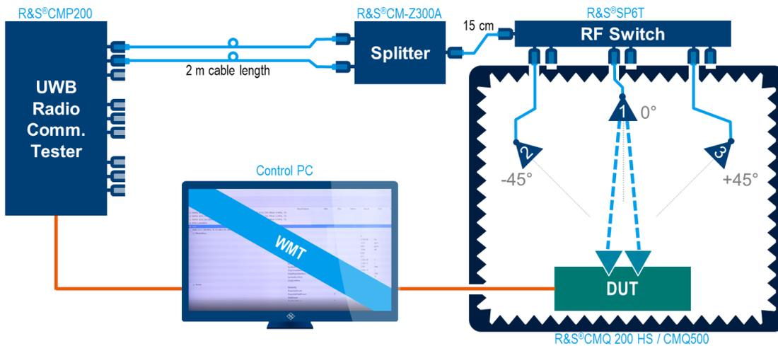
Figure 3-3 Block diagram of system variant 2: UWB OTA testing environment with RF switch for Tx, Rx, ToF and AoA measurement (multiple Vivaldi antennas)
