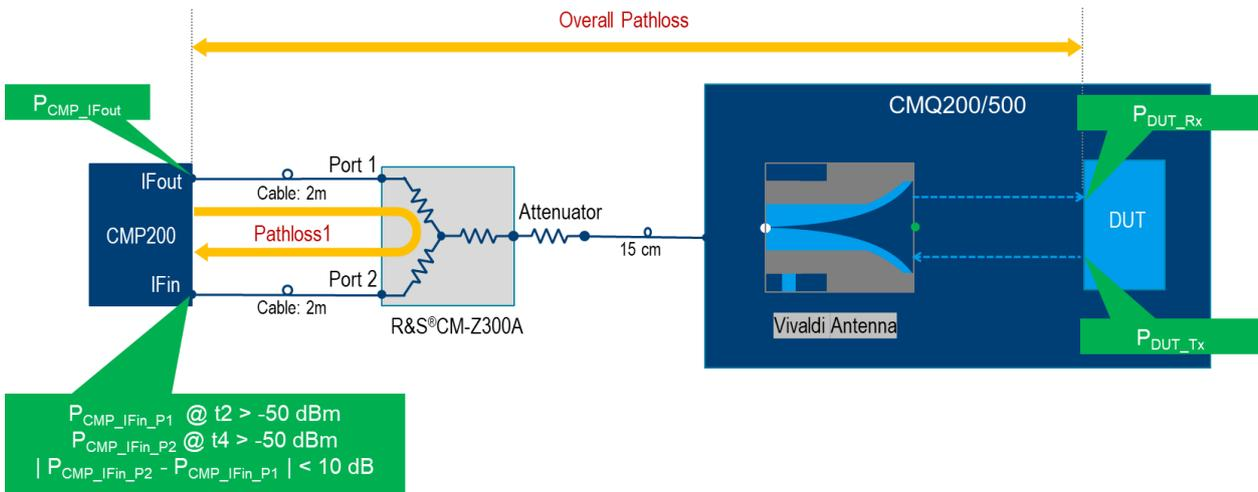
Figure 5-5 Power level consideration for ToF calibration/verification
