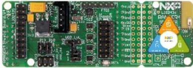
Figure 3-4 NXP Trimension™ NCJ29D5 evaluation board
