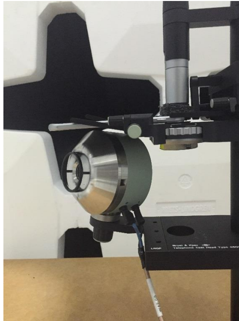
Fig. 2-7 and Fig. 2-8: EUT mounted to Telephone Test Head for Uplink Calibration.
