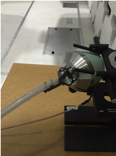
Fig. 2-10 and Fig. 2-11: Setup of Downlink Calibration
