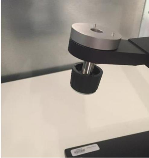
Fig. 1-3: Finger Screw inserted in LRGP subassembly
