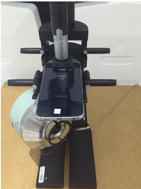
Fig. 2-7 and Fig. 2-8: EUT mounted to Telephone Test Head for Uplink Calibration.
