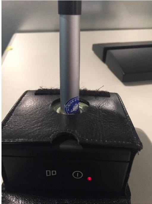
Fig. 2-3: Reference Microphone inserted into sound calibrator
