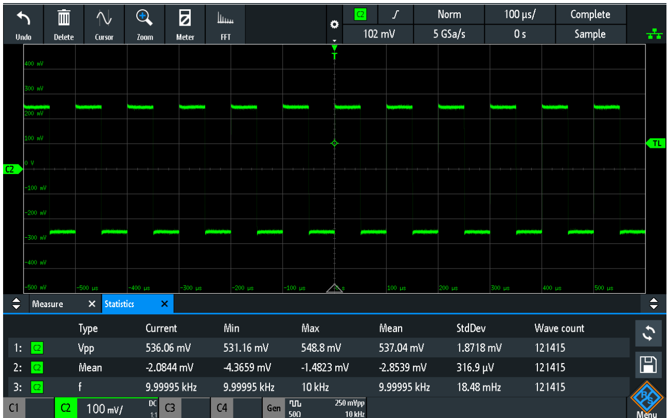
Figure 2 -- Captured waveform as a screenshot
