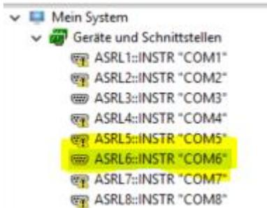
If the according Port is still marked with the yellow warning, just press [F5], sometimes it takes a while before the port can be recognized by NI MAX.
