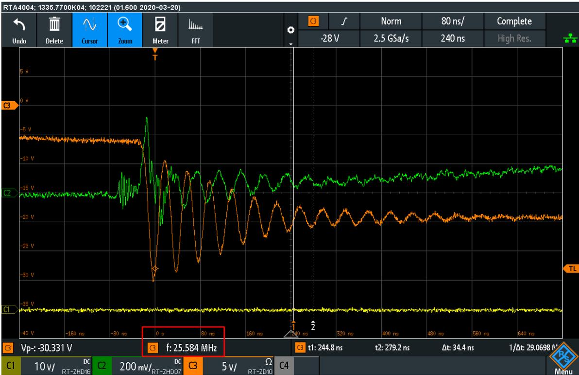
Figure 16 Rectifier Diode Oscillation (no additional capacitor)
