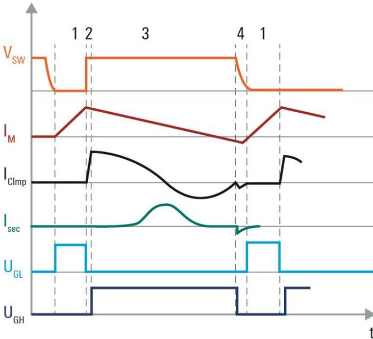
Figure 20 Active Clamp Waveforms (AAM)
