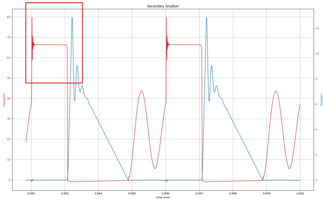
Figure 14 Simulation of Secondary Oscillation with RC-Damping
