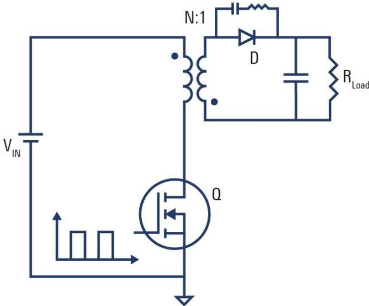
Figure 12 Secondary RC-Damping Circuit
