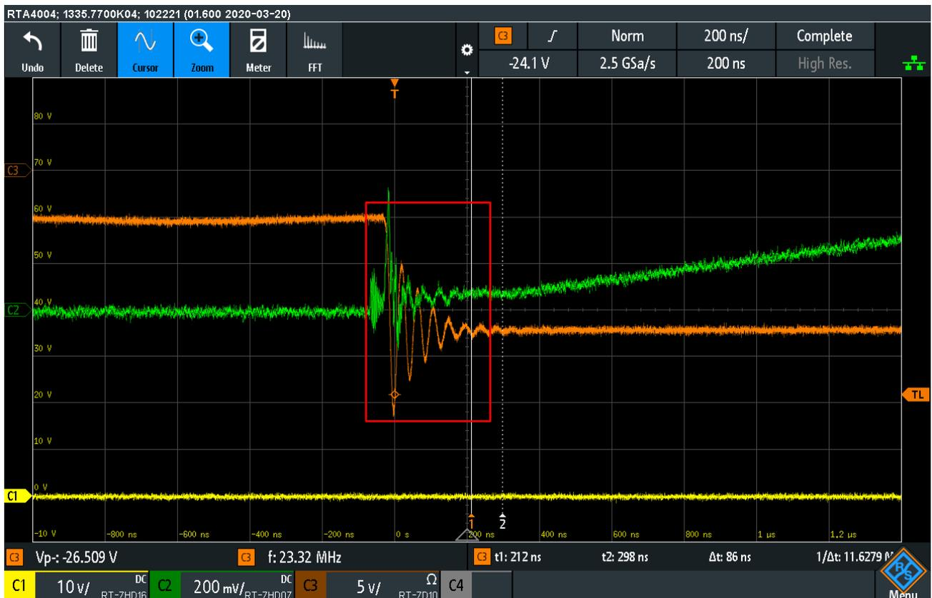
Figure 18 Rectifier Oscillation with the calculated RC damping network
