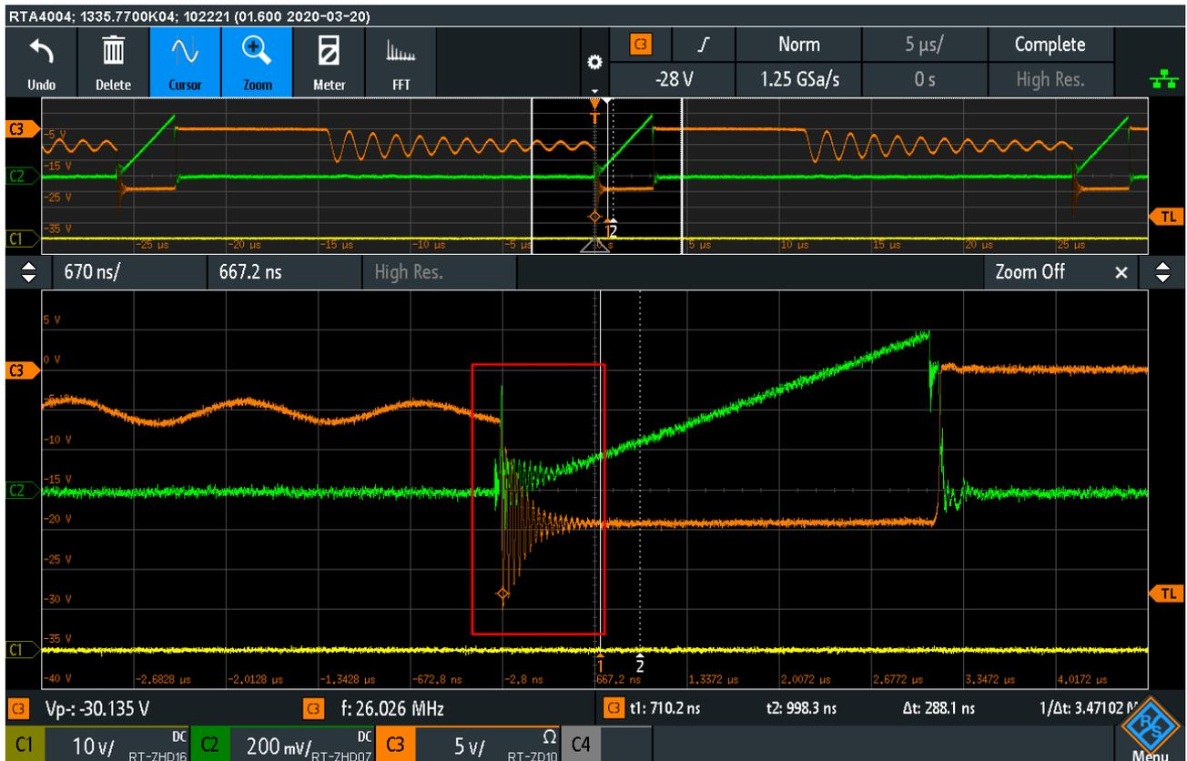
Figure 15 Rectifier Diode Oscillation
