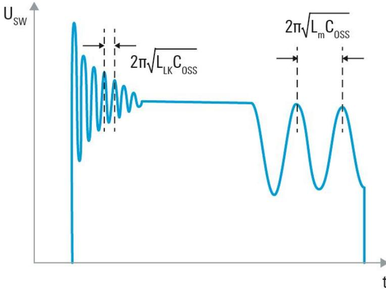
Figure 4 Switch Node Voltage Waveform
