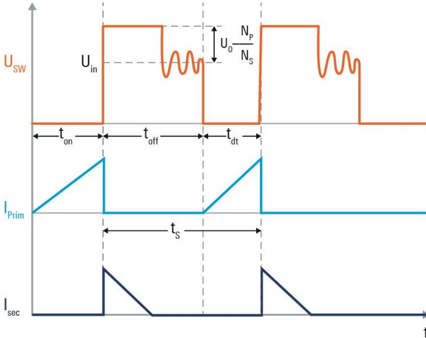
Figure 2 Flyback DCM Waveform
