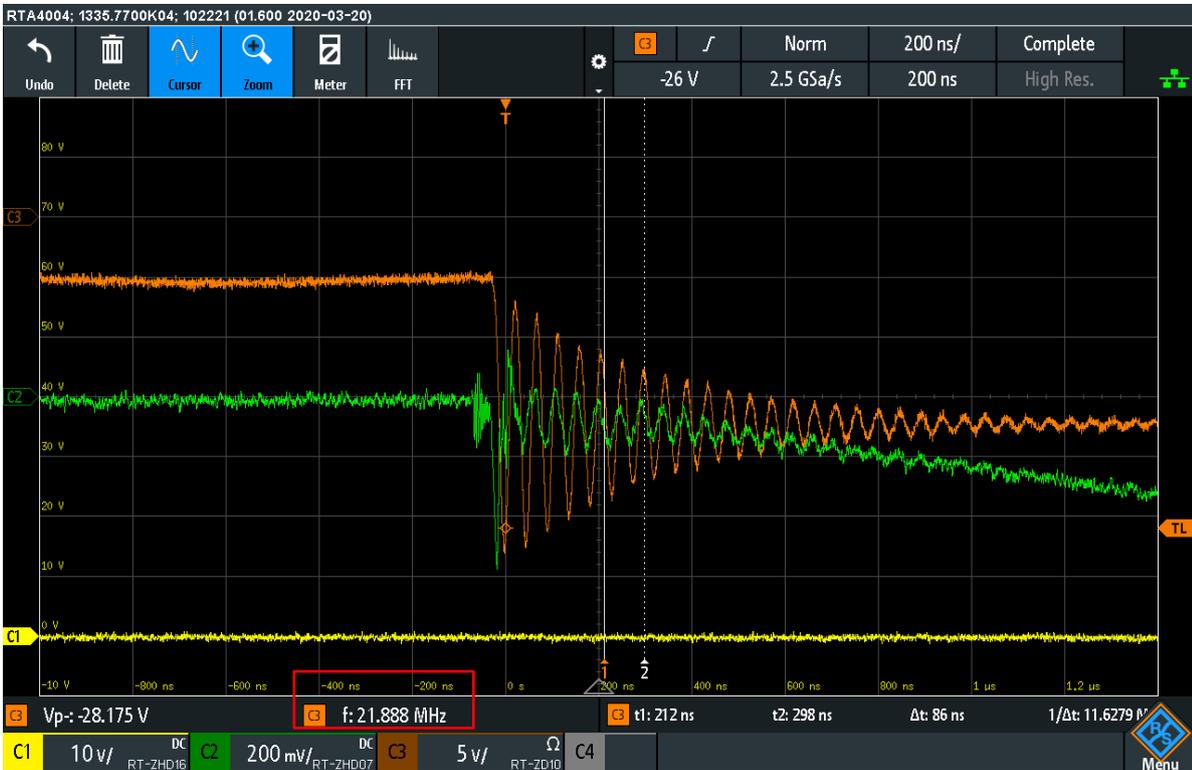
Figure 17 Rectifier Oscillation with additional 178 pF (Measured with LCR meter) capacitor
