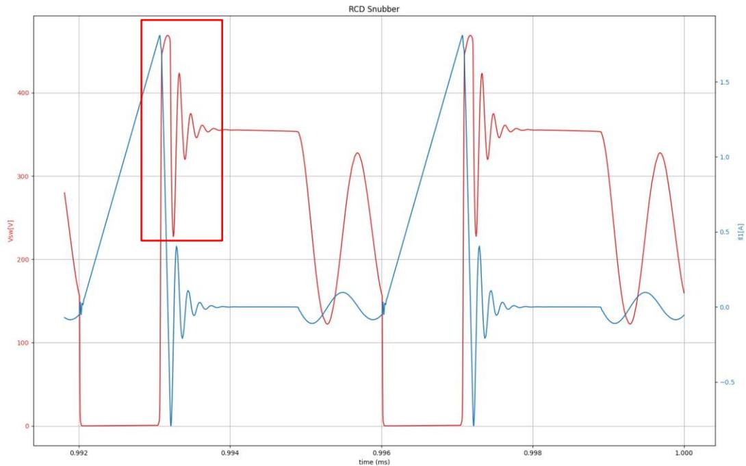
Figure 11 Simulation of RC-Damping (RCD-Snubber included)
