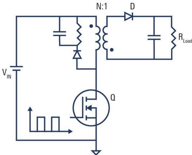
Figure 5 Passive RCD Snubber
