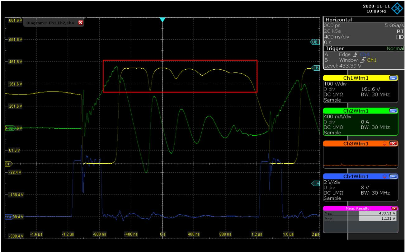
Figure 24 Low Power Mode Measurement @  $I_{out} = 100\text{mA}$
