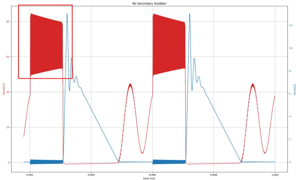
Figure 13 Simulation of secondary oscillation (RC-Damping not used)
