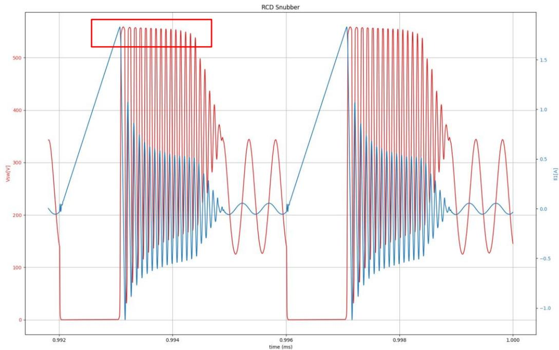
Figure 7 Simulation with RCD-Snubber
