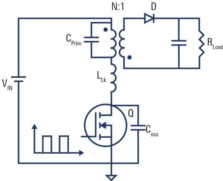
Figure 3 Flyback Structure with Parasitic Components
