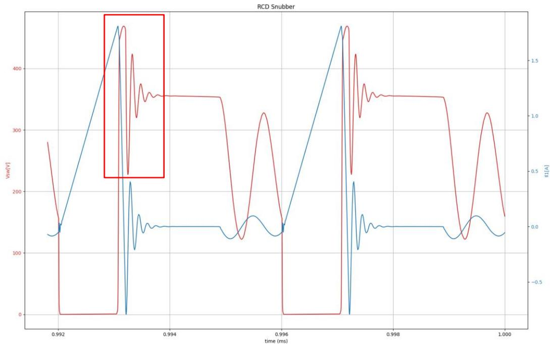
Figure 11 Simulation of RC-Damping (RCD-Snubber included)
