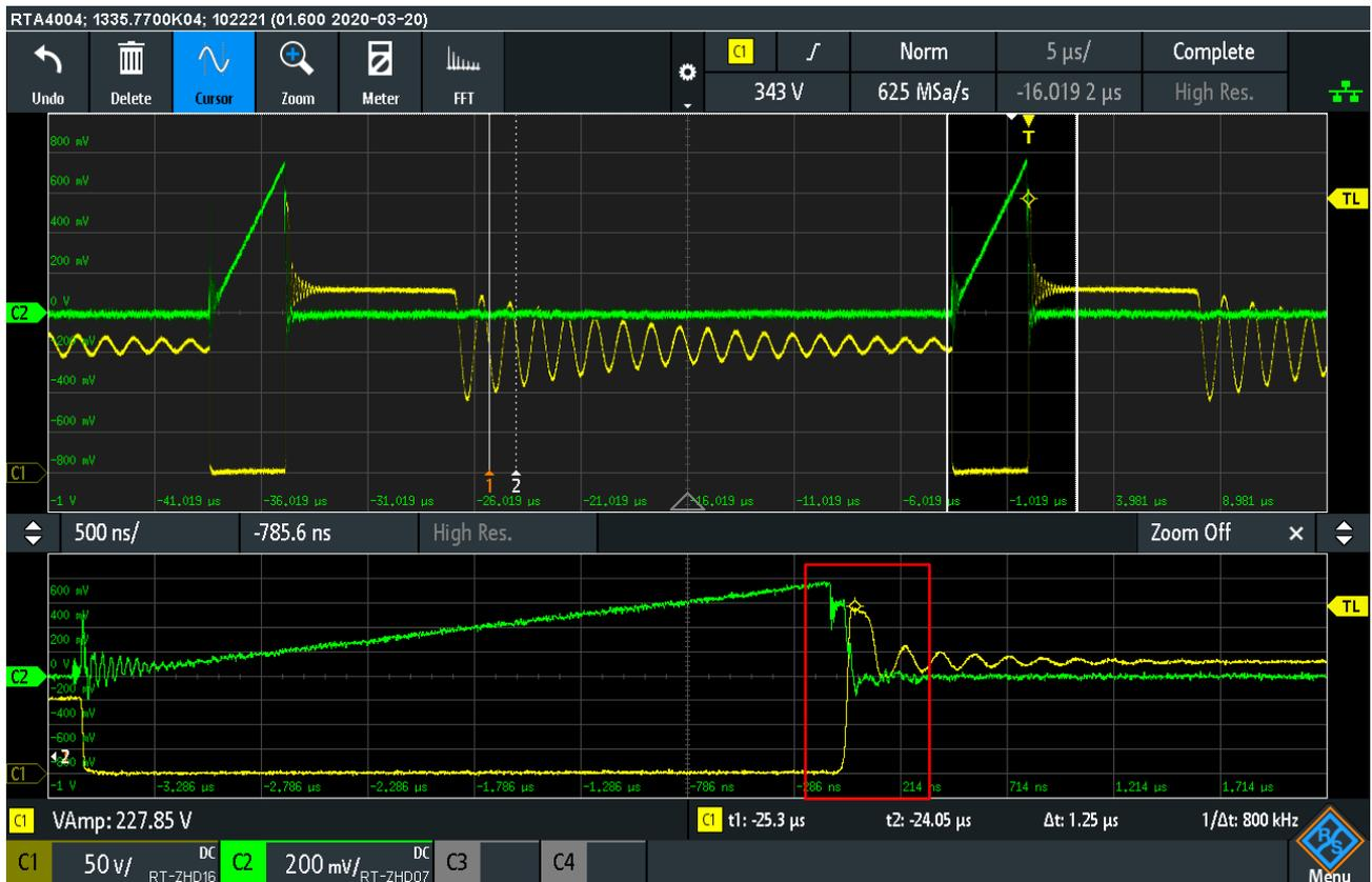
Figure 9 Maximum Drain Source Voltage with Snubber
