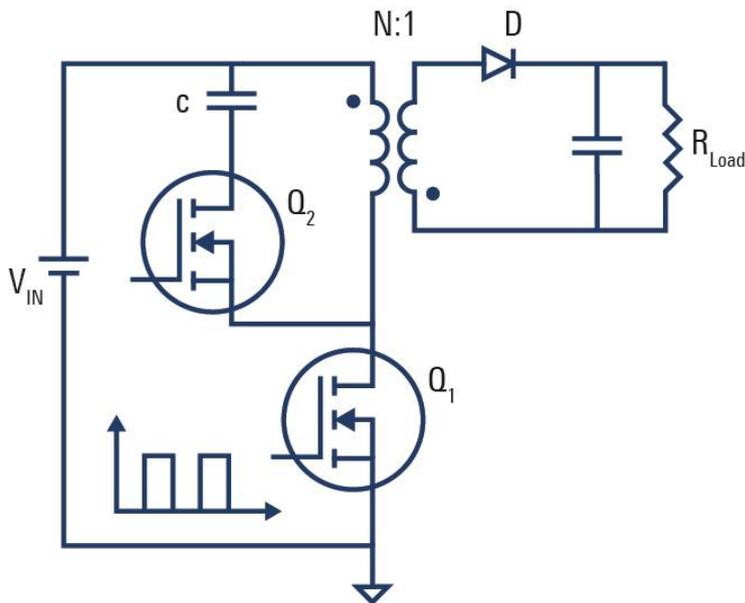
Figure 19 Active Clamp Structure
