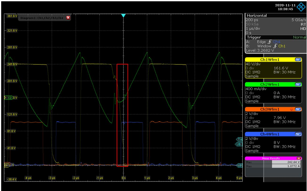
Figure 22 Transition from AAM to ABM (ZVS condition not always fulfilled)
