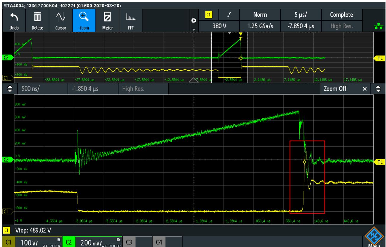
Figure 8 Maximum Drain Source Voltage (No Snubber)
