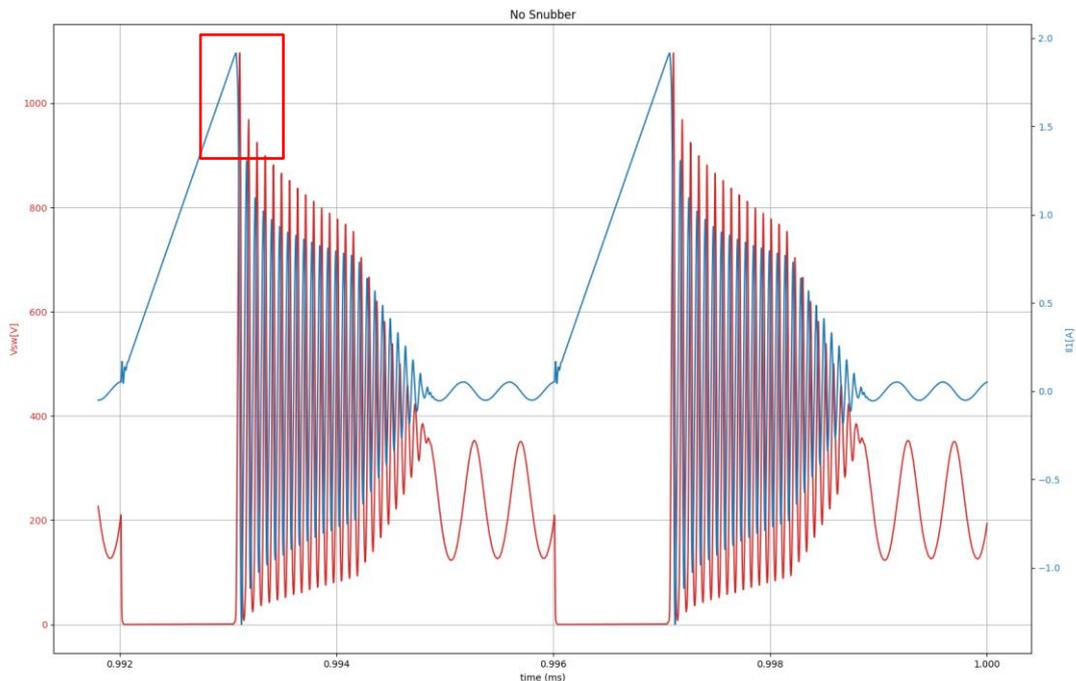
Figure 6 No Snubber Simulation
