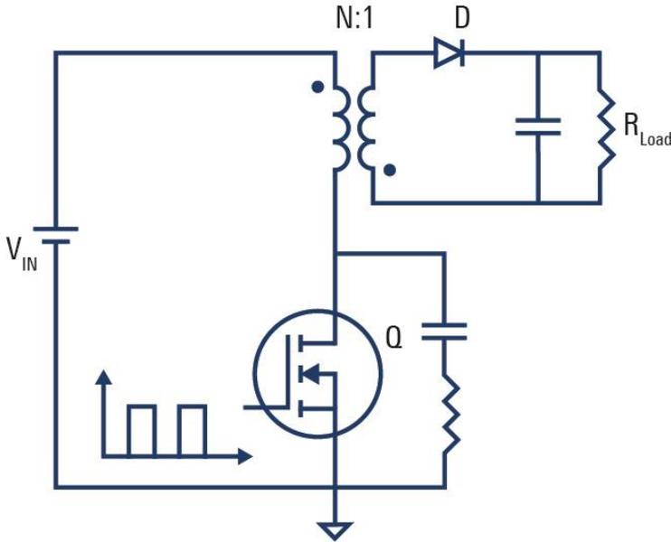
Figure 10 Primary RC-Damping
