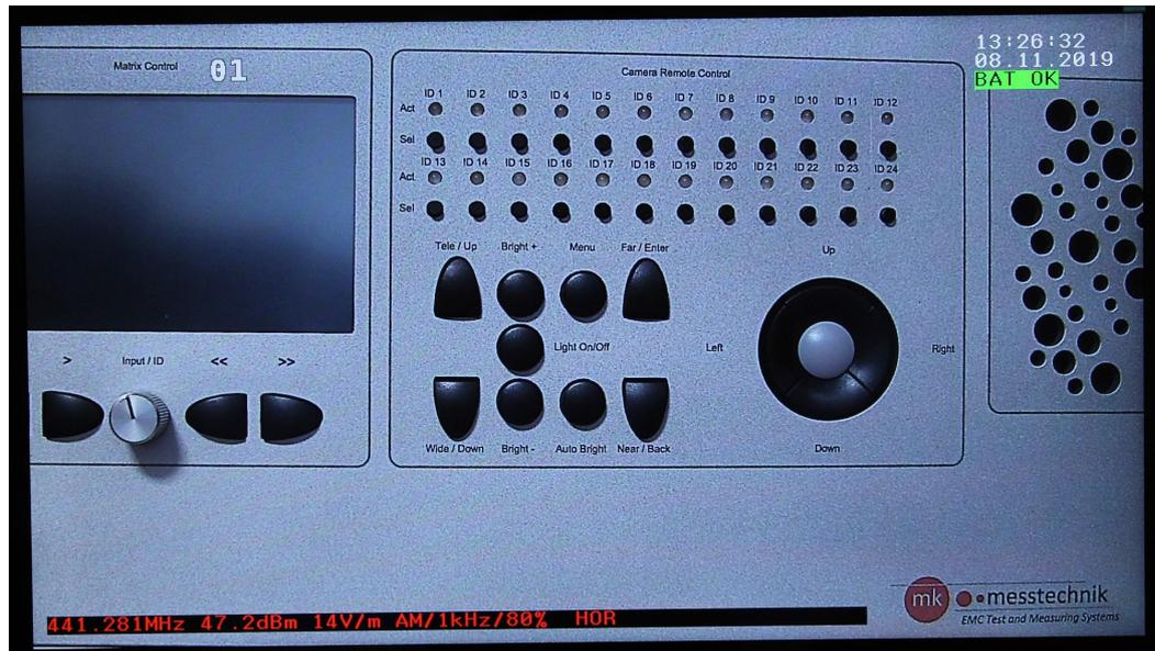
Figure 29: 1920x1080 monitor with date, time, battery status, and disturbance signal parameters
