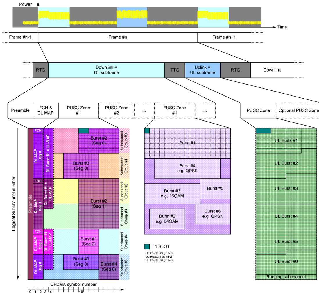
Fig. 12: OFDMA frame structure
