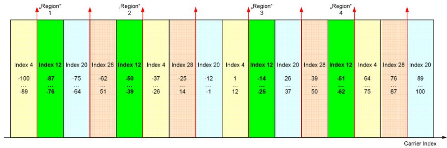
Fig. 9: Subchannelization with 4 used subchannels
