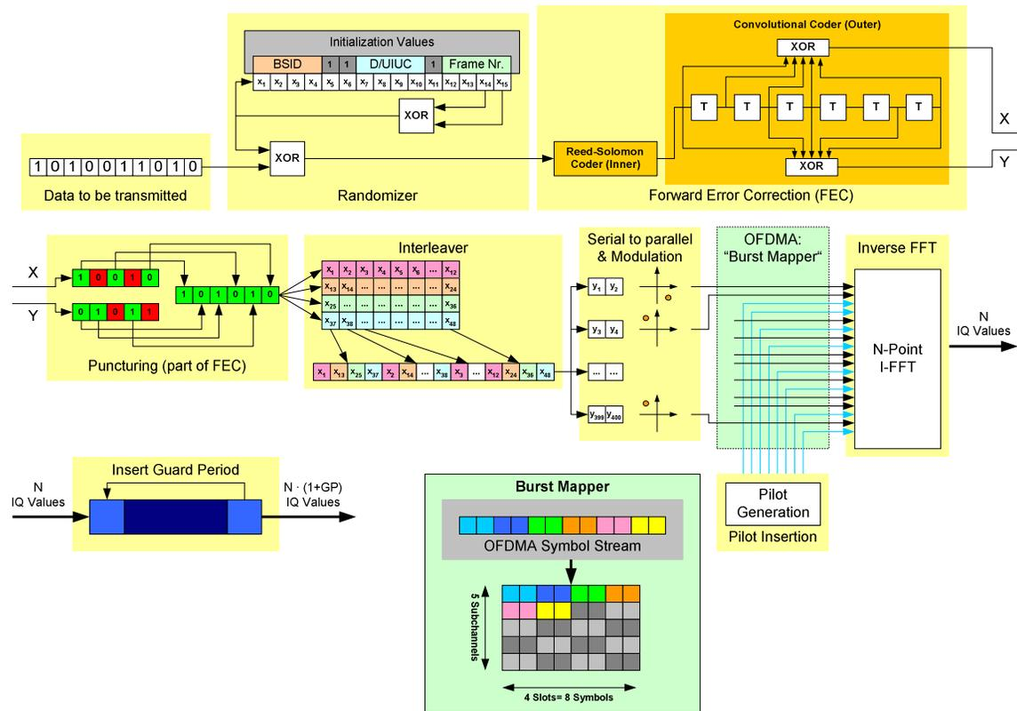
Fig. 11: OFDM / OFDMA transmitter architecture (simplified)
