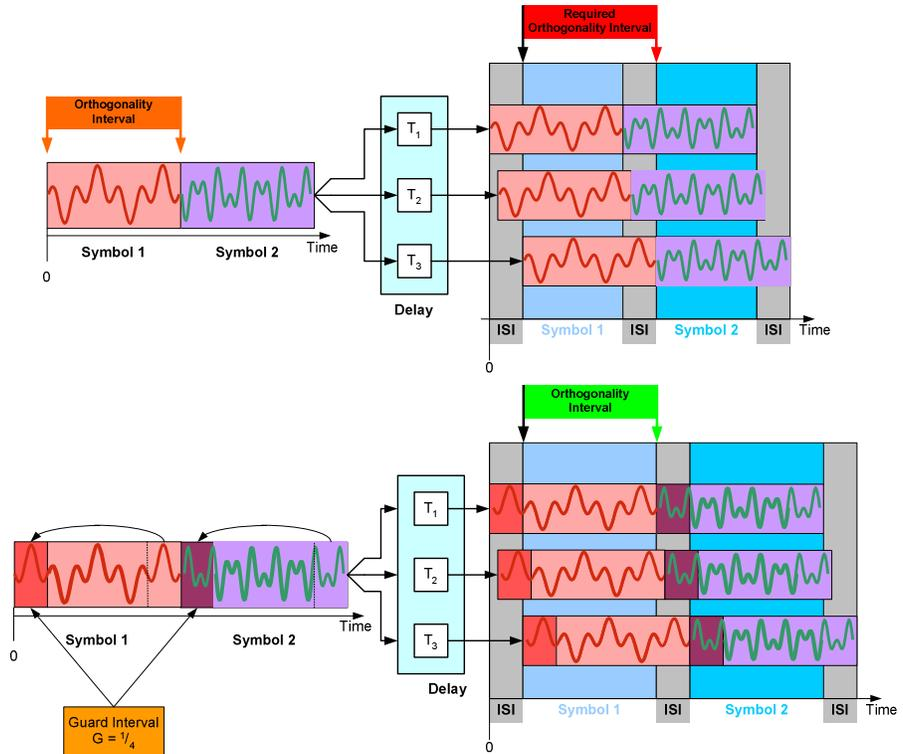
**Fig. 6: OFDM transmission with and without guard interval**
