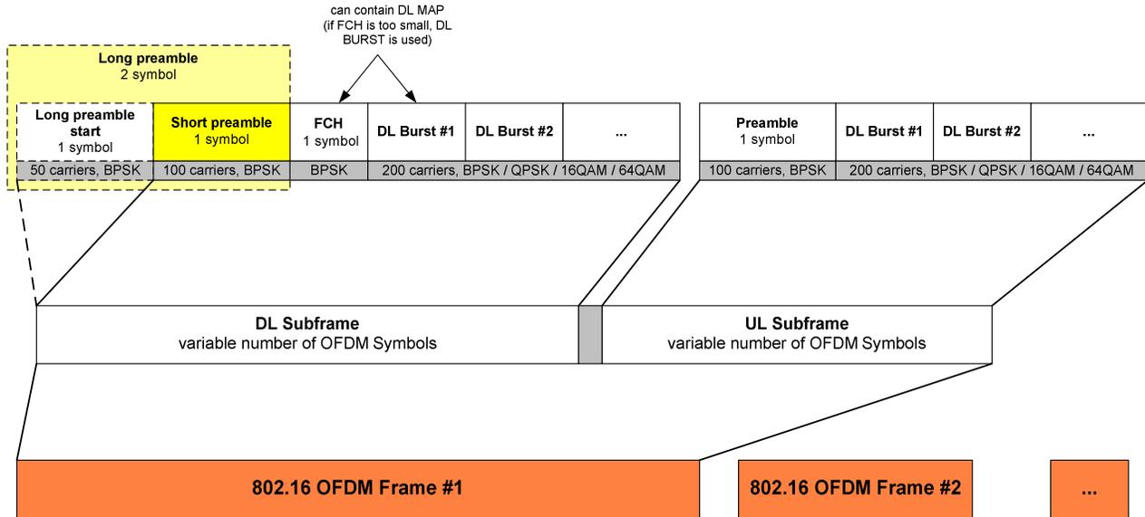
Fig. 10: 802.16 OFDM frame structure
