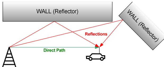
**Fig. 7: Multipath environment: direct path and reflection paths**
