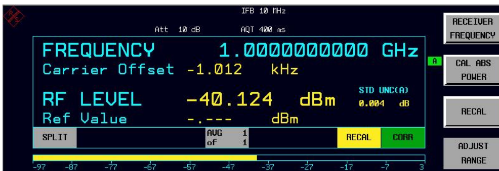
Figure 1: A portion of the FSMR display with the recalibration prompt (RECAL).
