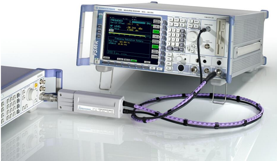
Figure 13: Test setup with an NRP-Z27 power sensor module
