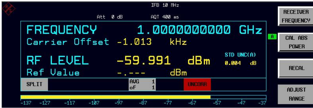
Figure 2: A portion of the FSMR display with the UNCORR indication to warn that the level is outside the permissible recalibration range.
