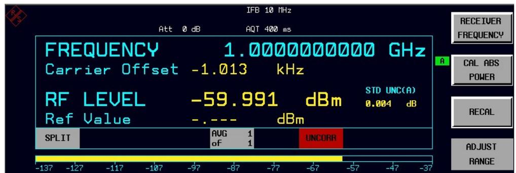
Figure 2: A portion of the FSMR display with the **UNCORR** indication to warn that the level is outside the permissible recalibration range.
