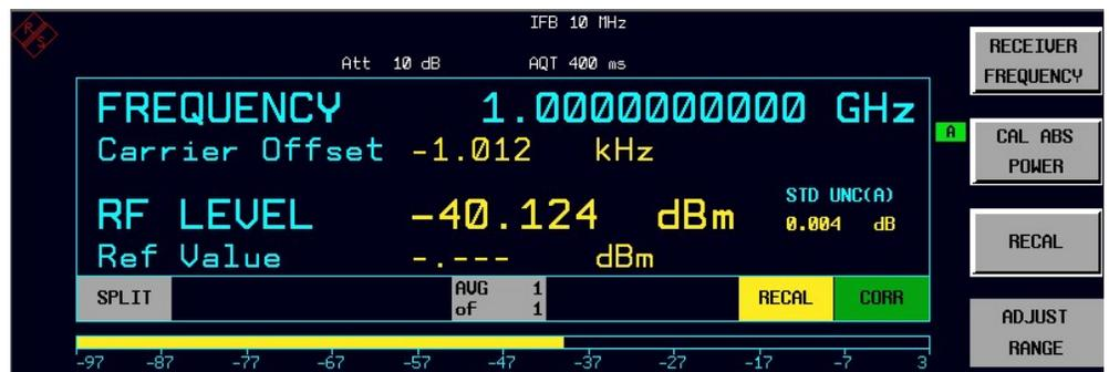
Figure 1: A portion of the FSMR display with the recalibration prompt (**RECAL**).
