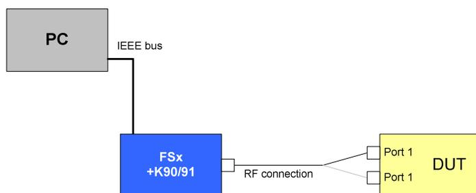
Drawing 8 – Center frequency leakage test setup
