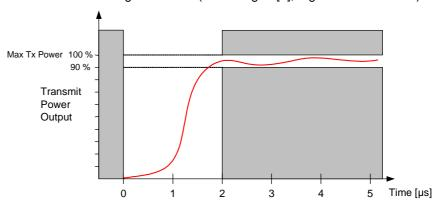
Figure 29 – 802.11b Power-up ramp specification
