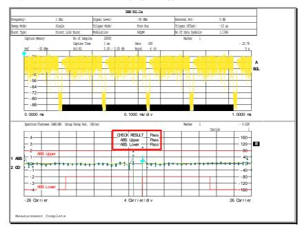
Figure 19 – Transmit spectral flatness measurement result
