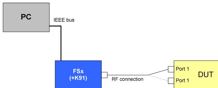
Drawing 17 – Transmit power levels test setup
