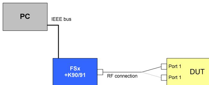
Drawing 6 – Center frequency tolerance test setup
