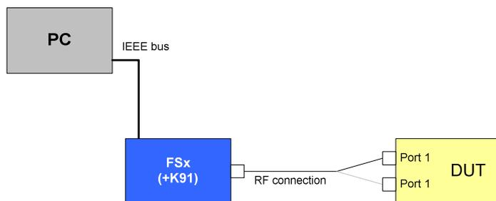
Drawing 18 – Transmit power level control test setup
