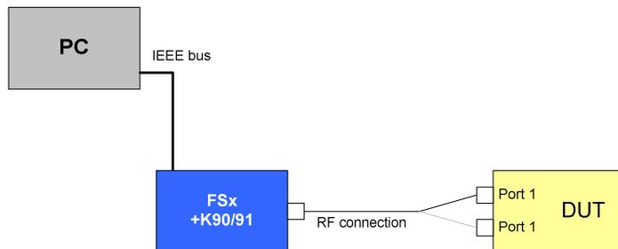
Drawing 7 – Symbol clock tolerance test setup
