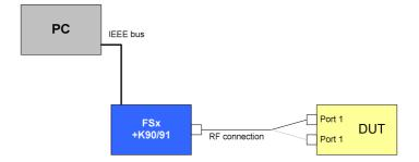
Drawing 8 - Center frequency leakage test setup
