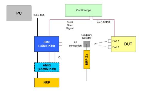
Drawing 16 - CCA sensitivity test setup
