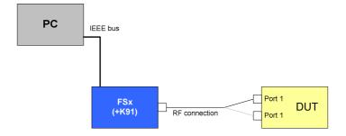
Drawing 18 - Transmit power level control test setup
