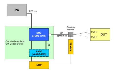
Drawing 15 - Receiver maximum input level test setup
