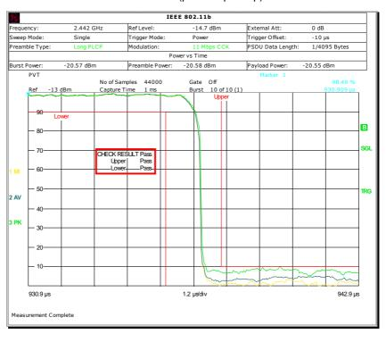
Figure 32 – Transmit power ramp typical measurement result (power-down ramp)
