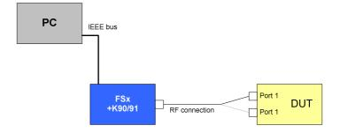
Drawing 10 – Constellation error test setup
