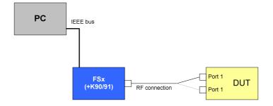
Drawing 4 - Transmit spectrum mask test setup
