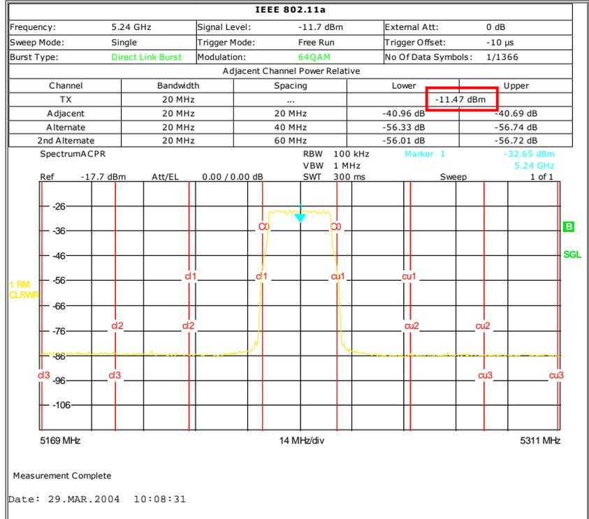
Figure 12 – Maximum transmit power level typical measurement result (using WLAN personality)
