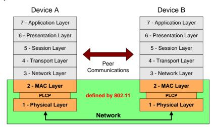
Figure 1 – The Layers of the OSI reference model applying to 802.11
