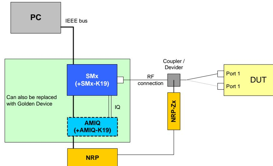
Drawing 25 – Receiver minimum input level sensitivity test setup
