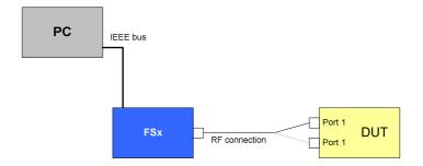
Drawing 5 – Transmit spurious test setup 1)
