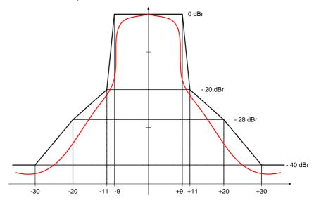
Figure 13 – 802.11a Transmit spectrum mask specification
