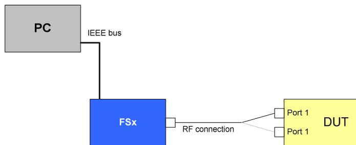
Drawing 5 – Transmit spurious test setup <sup>1)</sup>
