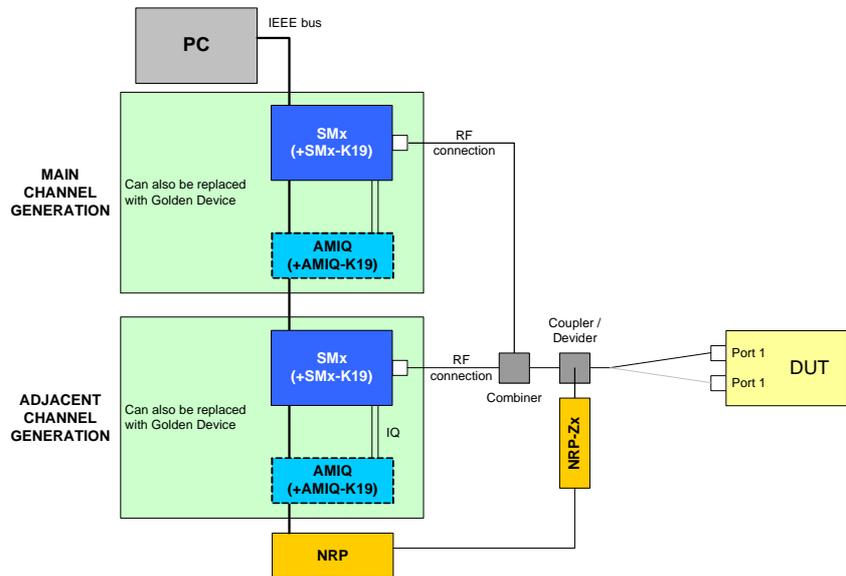
Drawing 14 – Non-adjacent channel rejection test setup
