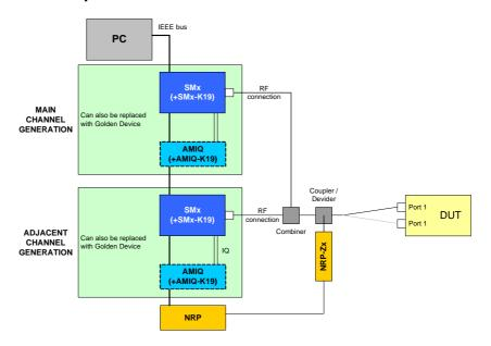
Drawing 14 - Non-adjacent channel rejection test setup
