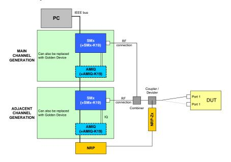
Drawing 13 - Adjacent channel rejection test setup
