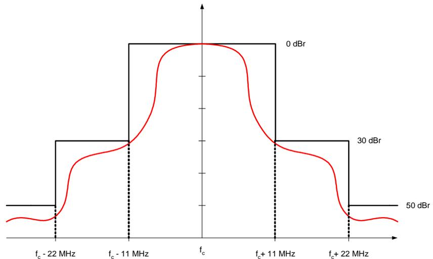
Figure 24 - 802.11b Transmit Spectrum Mask Specification
