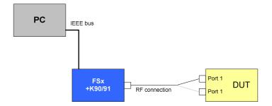
Drawing 11 - Modulation accuracy test setup
