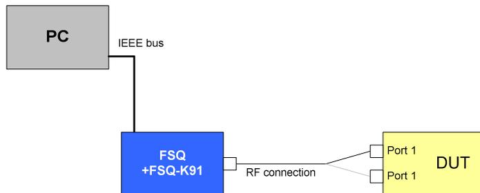
Drawing 21 – Chip clock frequency tolerance test setup
