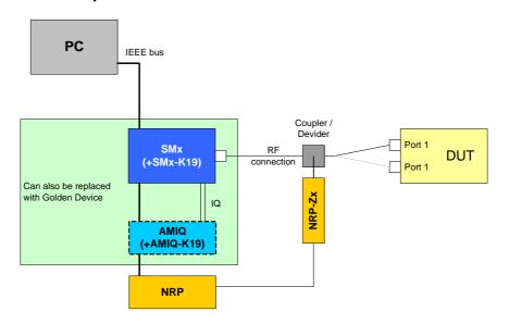
Drawing 26 - Receiver maximum input level test setup
