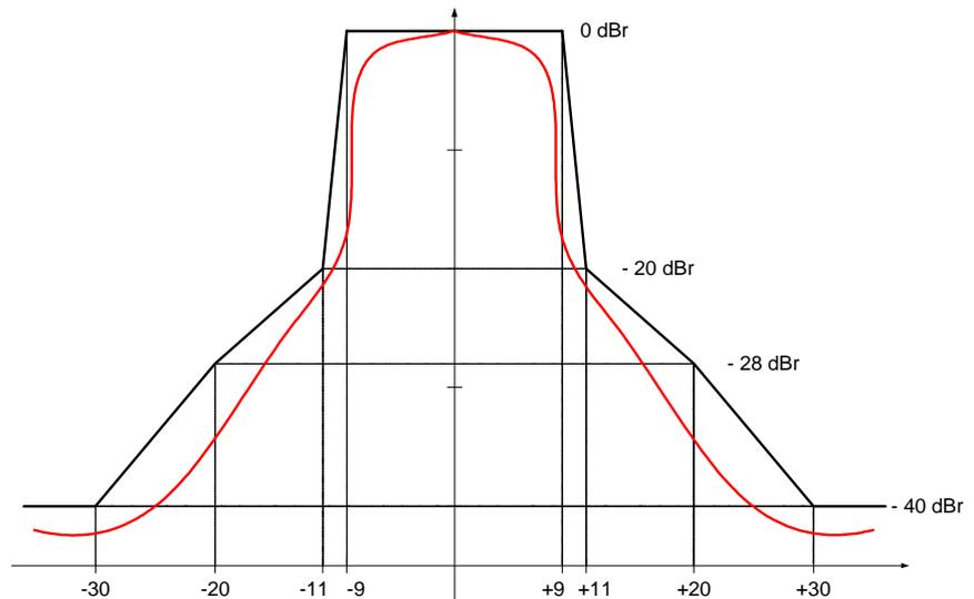
Figure 13 – 802.11a Transmit spectrum mask specification
