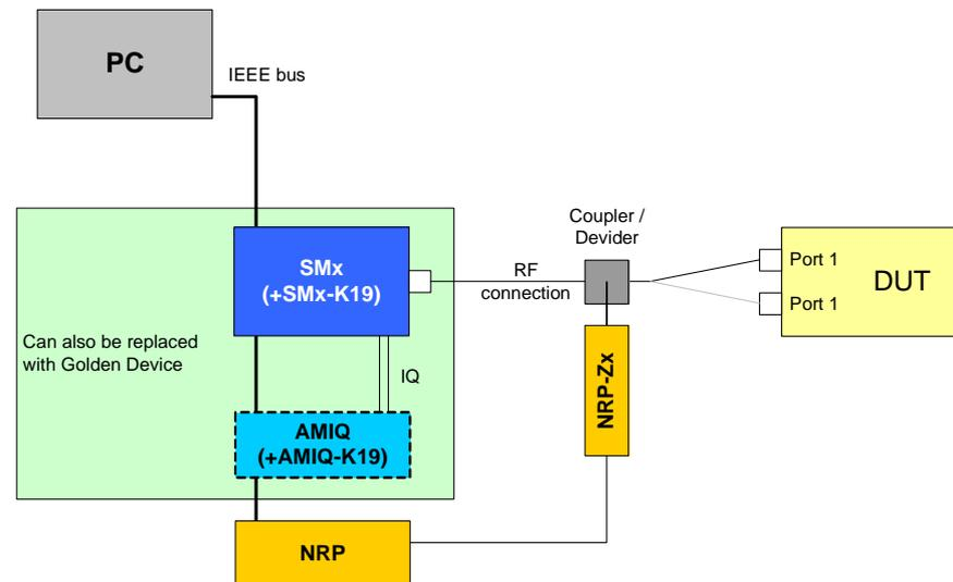
Drawing 26 – Receiver maximum input level test setup
