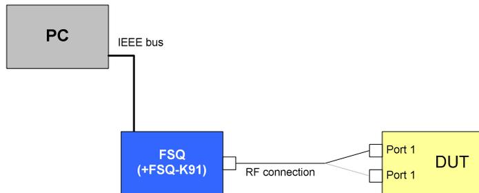
Drawing 23 – RF carrier suppression test setup
