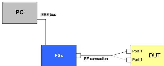
Drawing 2 – Spurious emissions test setup <sup>1)</sup>
