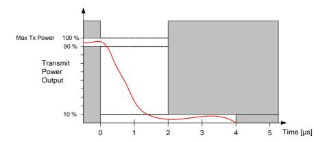
Figure 30 – 802.11b Power-down ramp specification
