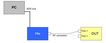
Drawing 2 – Spurious emissions test setup 1)
