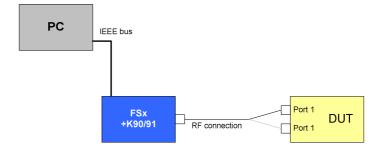
Drawing 7 - Symbol clock tolerance test setup
