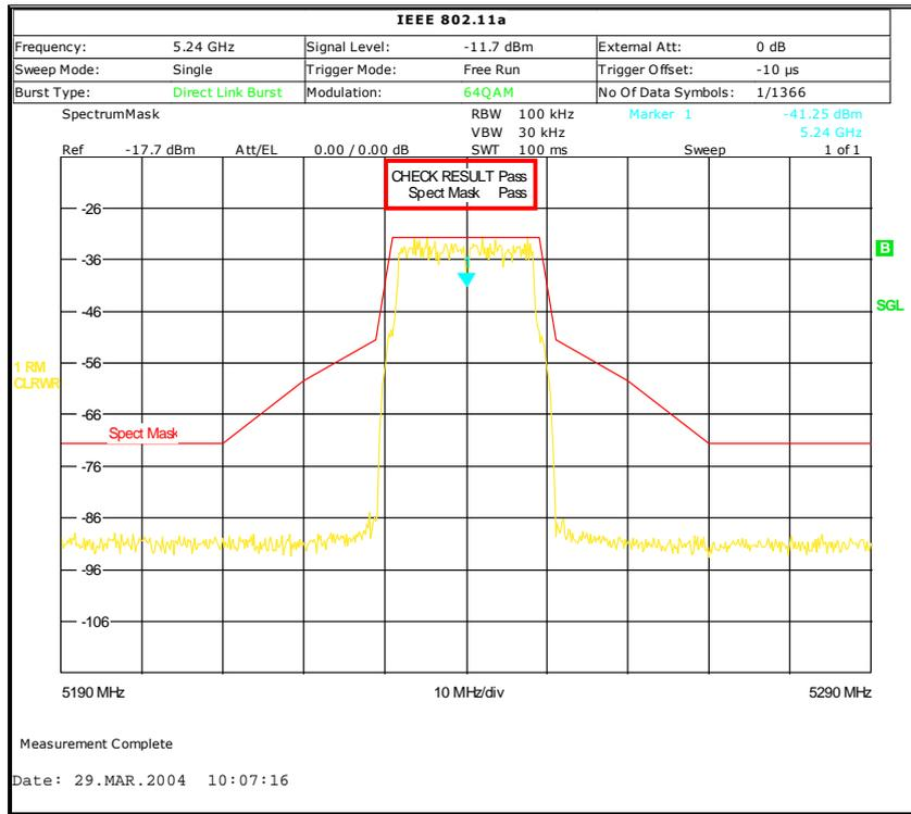
Figure 14 – Transmit spectrum mask measurement result
