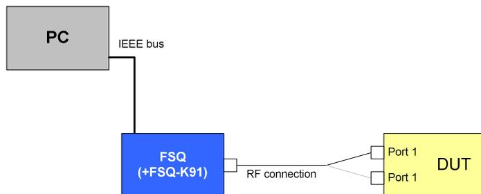
Drawing 22 – Transmit power ramps test setup
