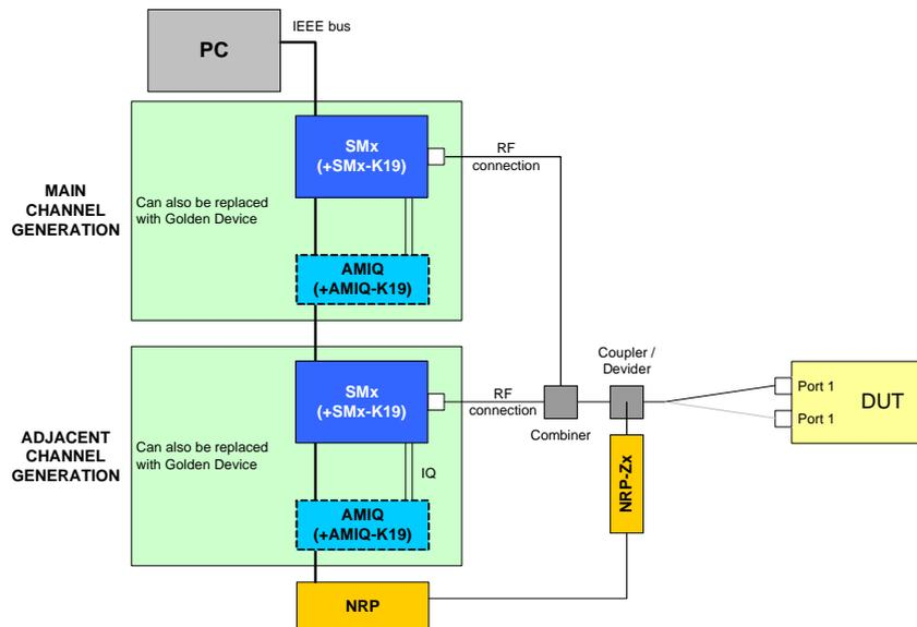
Drawing 13 – Adjacent channel rejection test setup
