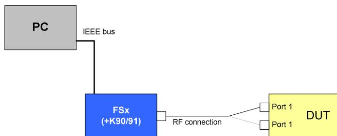
Drawing 1 – Occupied Bandwidth test setup
