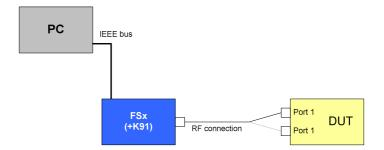
Drawing 17 - Transmit power levels test setup
