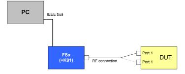
Drawing 19 - Transmit spectrum mask test setup
