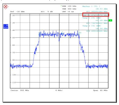
Figure 11 – Occupied bandwidth typical measurement result
