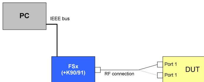
Drawing 3 – Maximum transmit power level test setup
