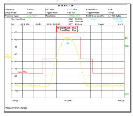
Figure 25 – Transmit spectrum mask typical measurement result
