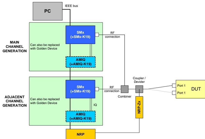
Drawing 27 – Receiver adjacent channel rejection test setup
