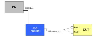
Drawing 24 - Transmit modulation accuracy test setup
