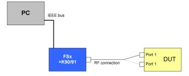
Drawing 9 - Transmit spectrum flatness test setup
