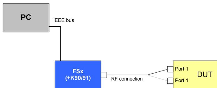
Drawing 4 – Transmit spectrum mask test setup
