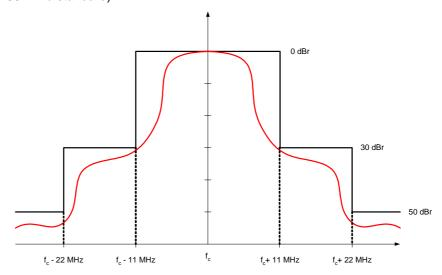
Figure 24 - 802.11b Transmit Spectrum Mask Specification
