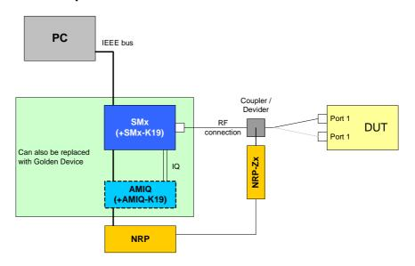
Drawing 12 - Receiver minimum input level test setup
