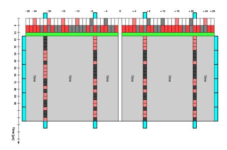
Figure 4 – 802.11a spectrogram representation (carriers vs time)
