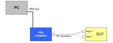
Drawing 1 - Occupied Bandwidth test setup
