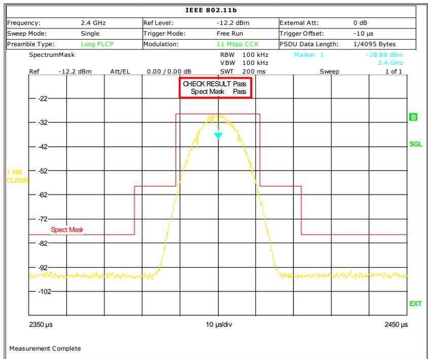
Figure 25 – Transmit spectrum mask typical measurement result
