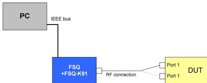
Drawing 20 – Transmit center frequency tolerance test setup
