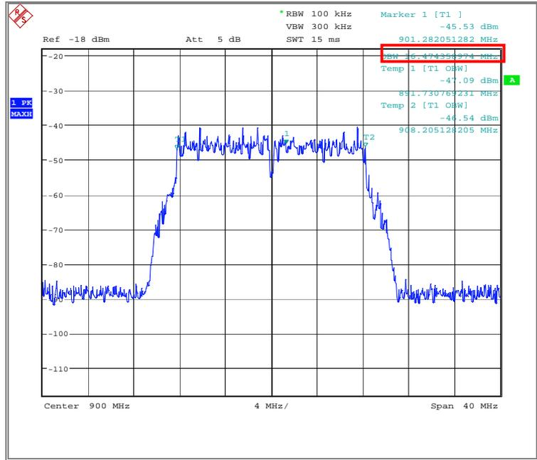
Figure 11 – Occupied bandwidth typical measurement result
