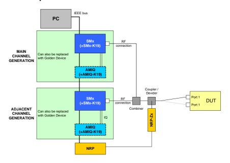
Drawing 27 - Receiver adjacent channel rejection test setup
