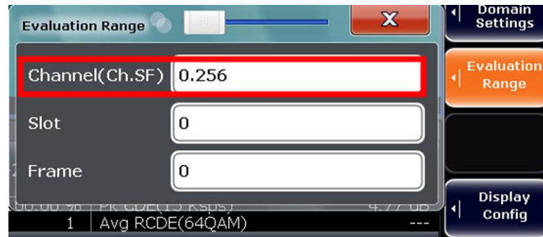
Fig. 3-28: Select channel 0 using "Evaluation Range". The spreading factor is detected automatically.
