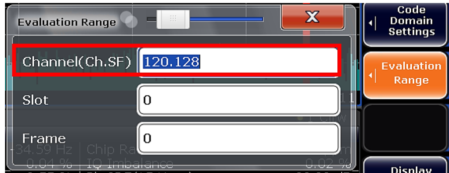
Fig. 3-49: FSx: Set Channel to 120 to measure code domain power on channel 120
