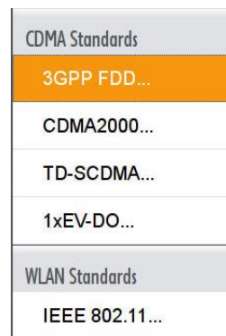
Fig. 3-6: SMW: select W-CDMA in the baseband block
