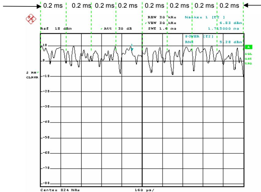
Figure 6: Gated measurement over 8 EDGE frames (50 – 90 % of slot 1) with sweep time 1.6 ms and gate length 0.2 ms. The RMS value of the trace is output.
