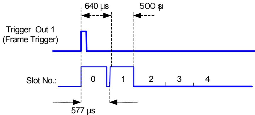
Figure 3: Setting for measuring the power of slot 1
