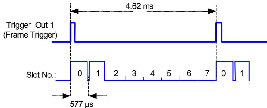
Figure 2: GSM/EDGE timing, slot 0 and slot 1 active
