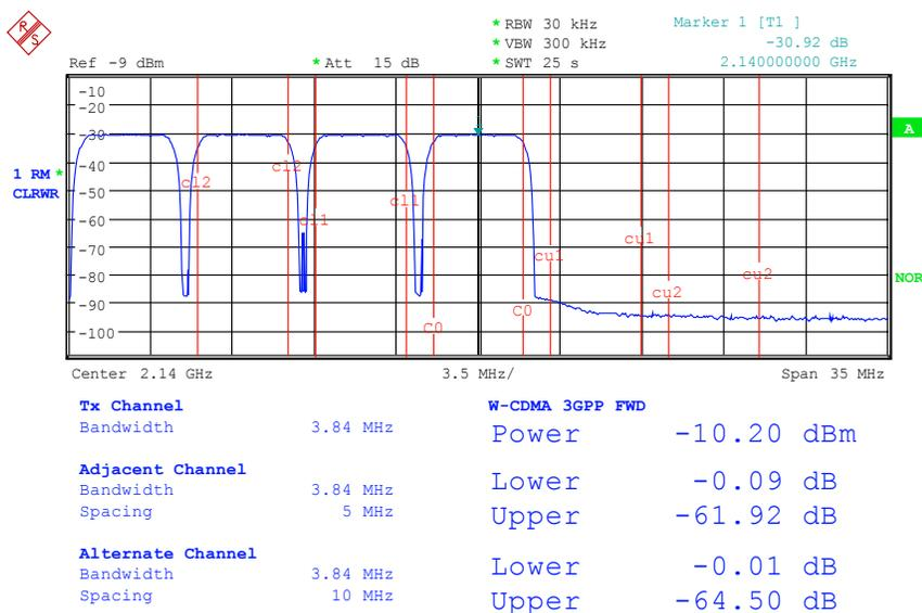
Fig. 4: ACLR measurement results, upper adjacent channel and 1st alternate channel
