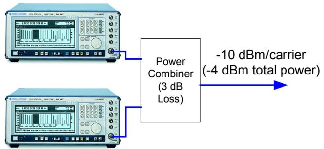
Fig. 6: Recommended simplified configuration using 2 SMIQs
