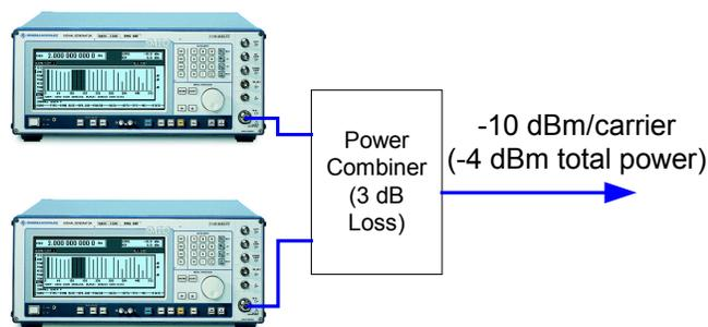
Fig. 6: Recommended simplified configuration using 2 SMIQs
