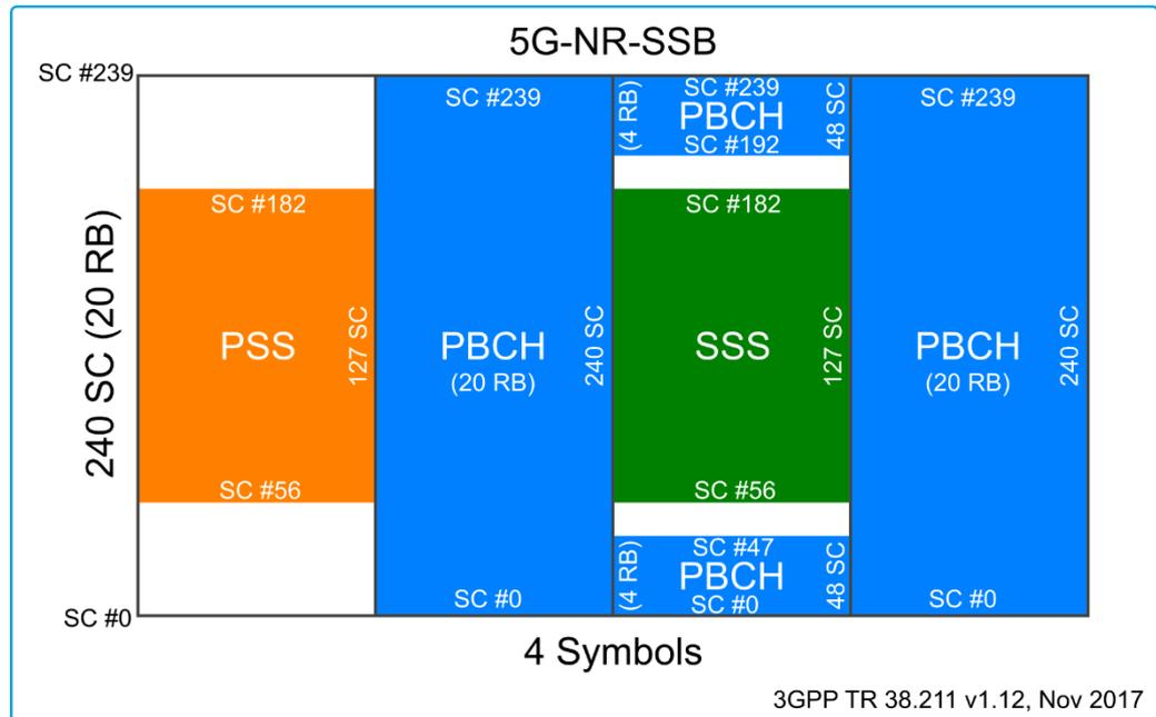
Figure 1: Synchronization Block Mapping
