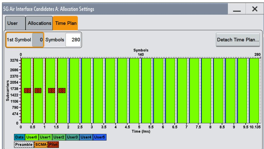
Figure 5: SMW-K114 Allocation Time Plan
