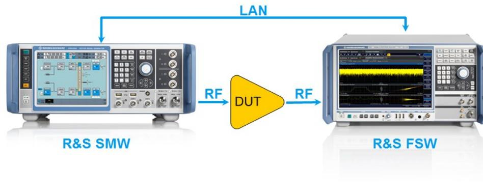
Fig. 2-1:-K18 test setup
