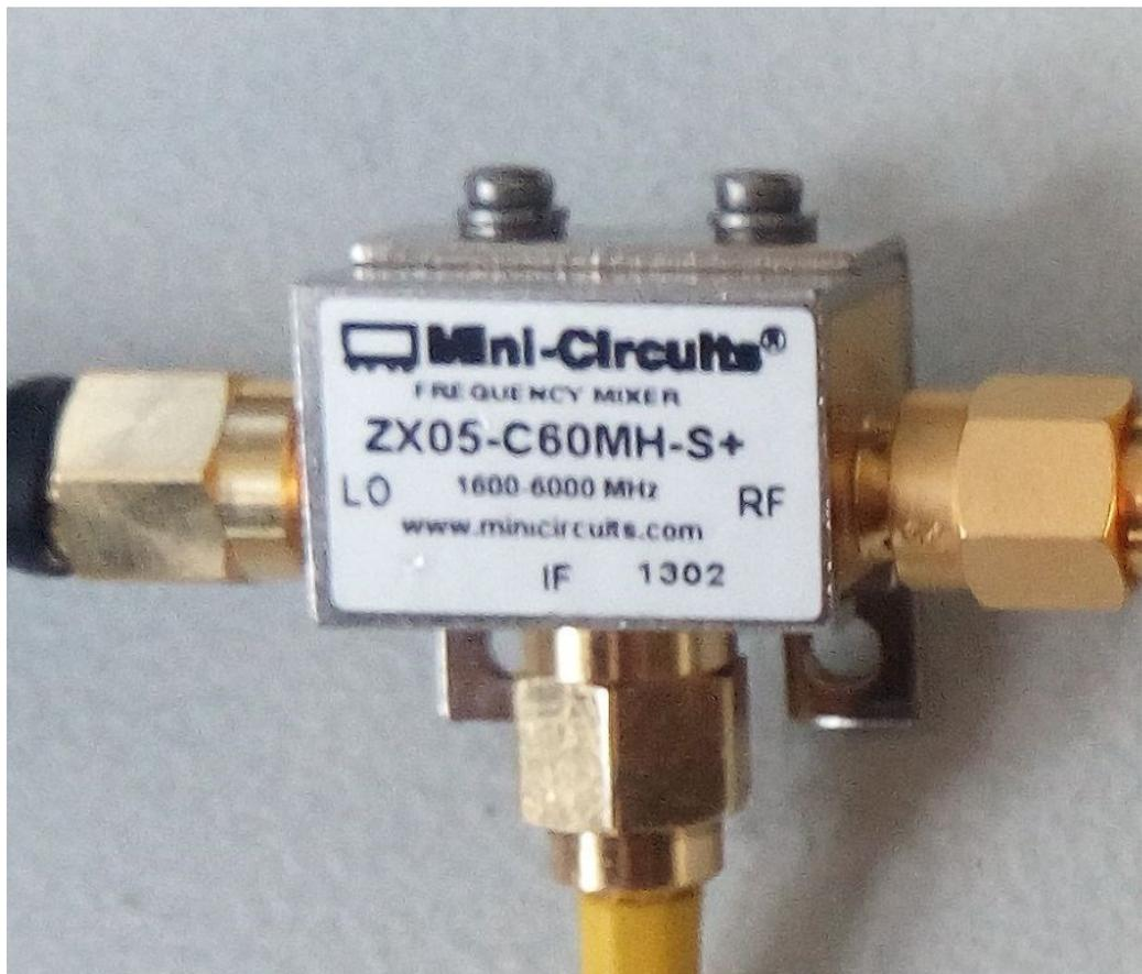
Fig. 3-4: Mixer DUT, the ZX05-C60MH-S+ from Mini-Circuits
