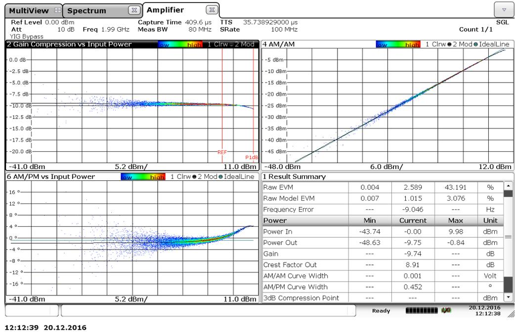
Fig. 3-8: Mixer DUT operating with signal peak envelope power (PEP) set to one dB gain compression point (P-1dB) at 1.99 GHz
