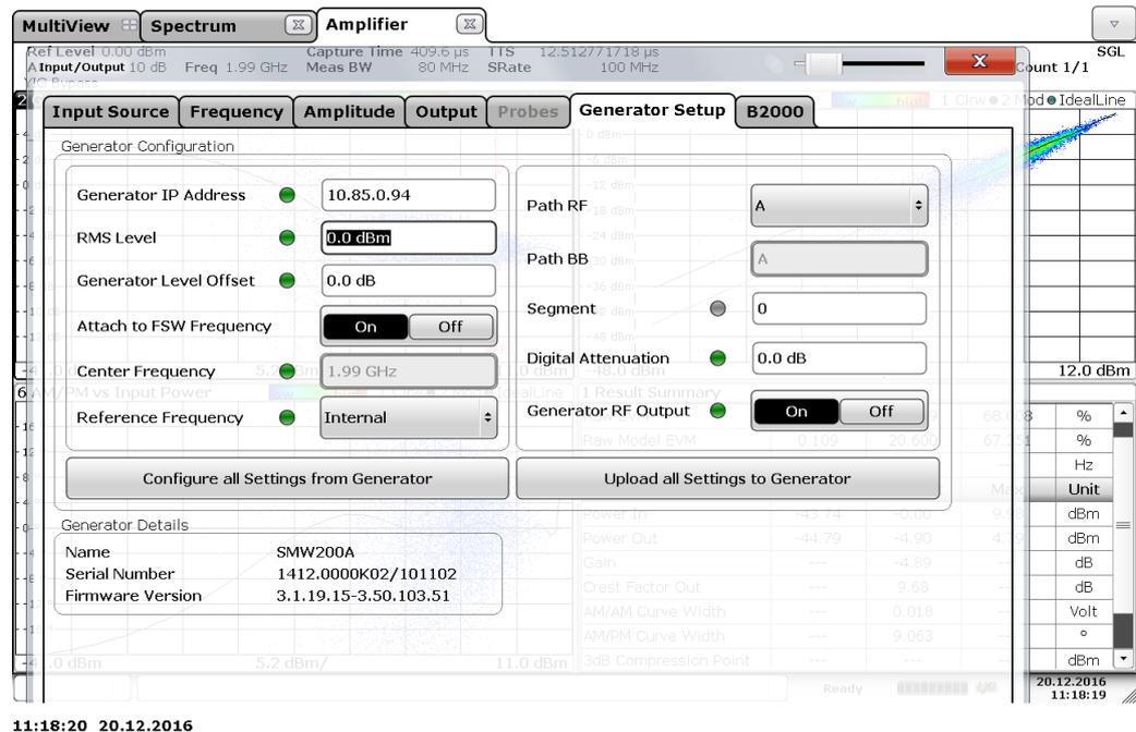
Fig. 3-2: Configuring the FSW-K18 - Modifying output level of the SMW from the FSW.
