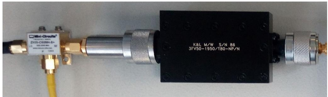
Fig. 3-9: Cascade of mixer and band pass filter
