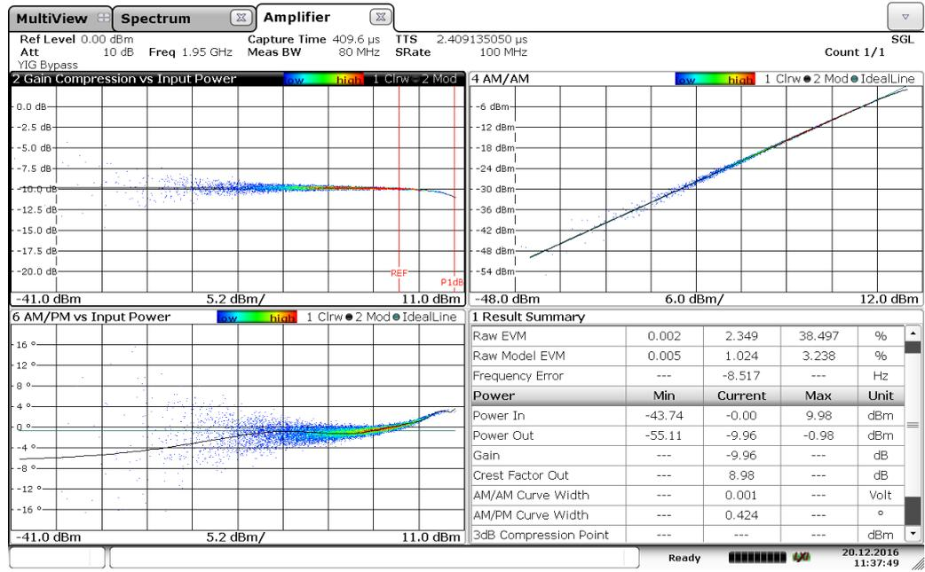
Fig. 3-7: Mixer DUT operating with signal peak envelope power (PEP) set to one dB gain compression point (P-1dB) at 1.95 GHz
