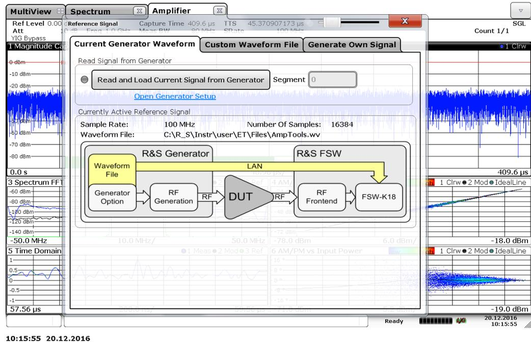
Fig. 6-1: Driving the FSW-K18 using an ARB waveform resident on the SMW
