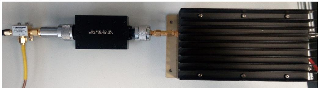
Fig. 3-11: The complete, discrete, RFFE, comprising a cascade of mixer, band pass filter and power amplifier.
