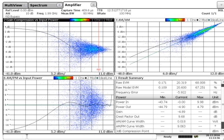
Fig. 3-3: Frequency sweep characteristic of the Band Pass Filter DUT with center frequencies 1.95, 1.97 and 1.99 GHz. Note the increasing dispersion, spreading in the AM-xM scatter plots, as the band edge is approached.
