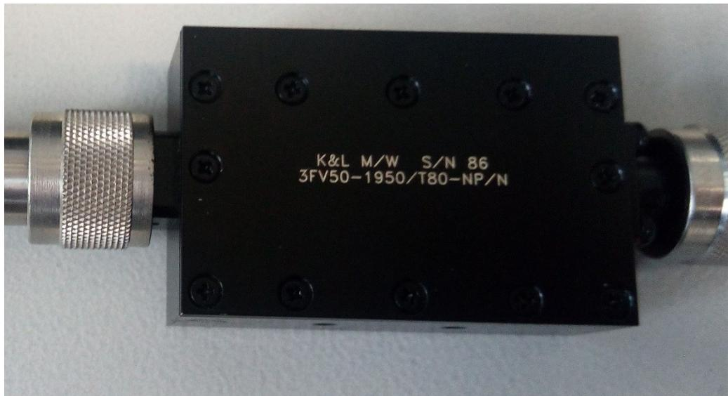
Fig. 3-1: Band Pass Filter DUT from K&L
