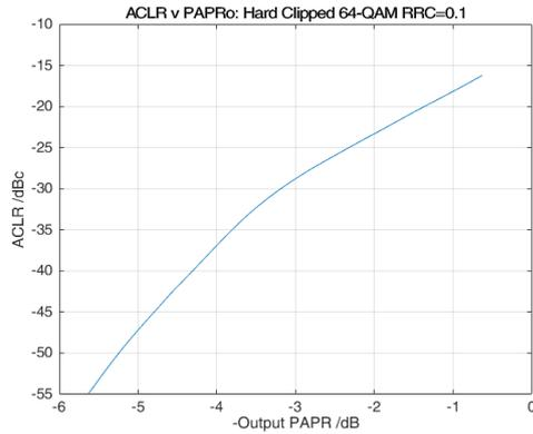
**Fig. 4-2: ACLR v PAPRo (spectral regrowth versus output peak-to-average-power ratio) behavior for the 64-QAM (RRC=0.1) test signal played through a hard clipper**
