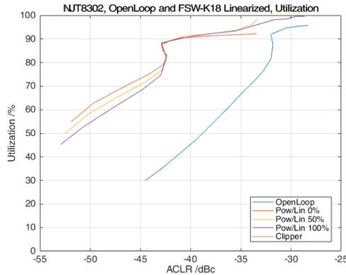
Fig. 4-6: Utilization (i.e. the ratio of PEP to PSat) of the Open Loop and Linearized NJT8302 device
