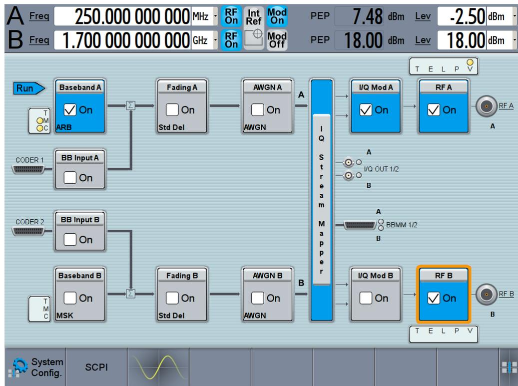
**Fig. 3-6: Configuring the SMW - Modifying the two SMW output frequencies and levels to drive the Mixer DUT**
