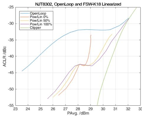
**Fig. 4-5: Measurement of Open Loop and (Exemplary) DPD Linearized performance of the NJT8302, with 10 MSym/s RRC=0.1 64-QAM test signal**
