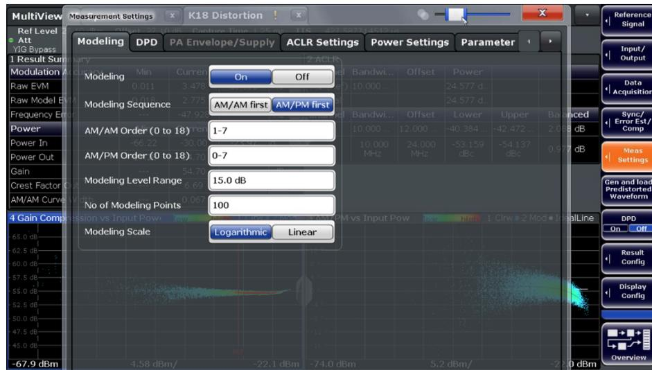
Fig. 4-1: DPD Modeling settings for Linearization of the NJR8302 BUC
