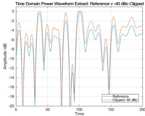
Fig. 4-3: Power v Time curves for a clean reference waveform, and the same clipped to -40 dB ACLR
