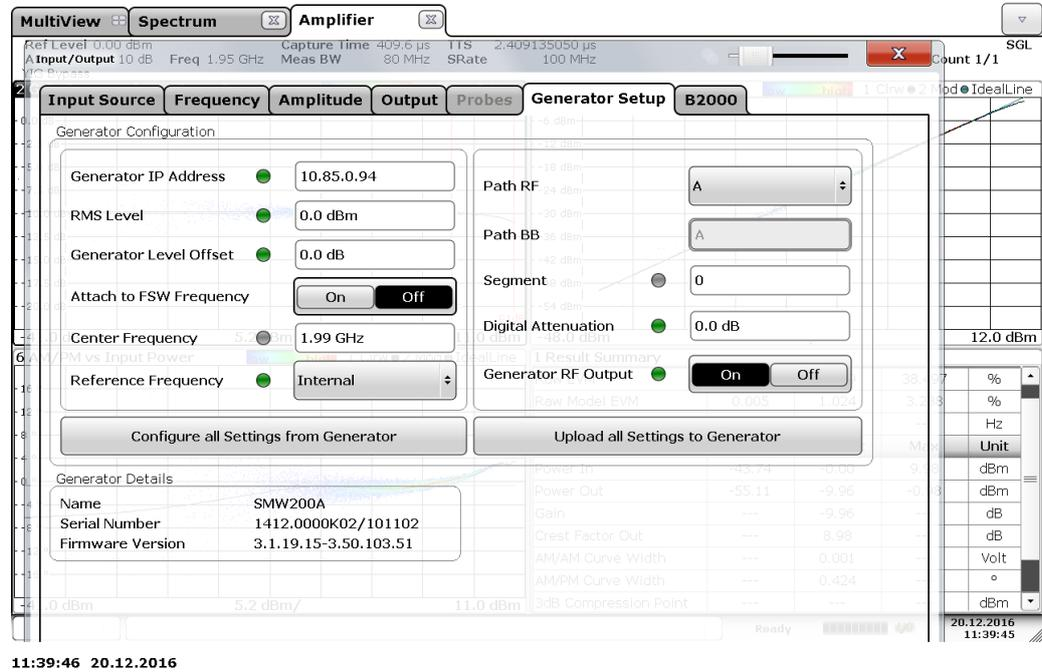
**Fig. 3-5: Configuring the FSW-K18 - Decoupling the SMW and FSW operating frequencies to test frequency conversion devices.**
