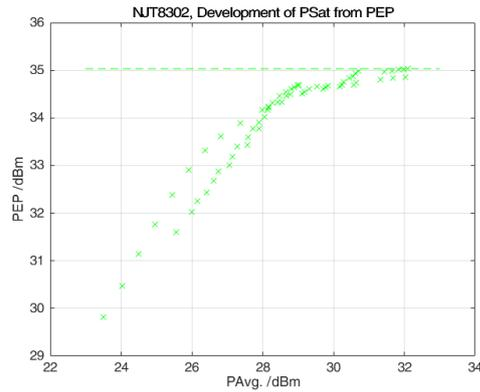
**Fig. 4-4: PSat (Saturated output power) measurement of the NJT8302) with 10 MSym/s RRC=0.1 64-QAM test signal, with PAvg x-axis and PEP = PAvg + PAPRo on the y-axis.**
