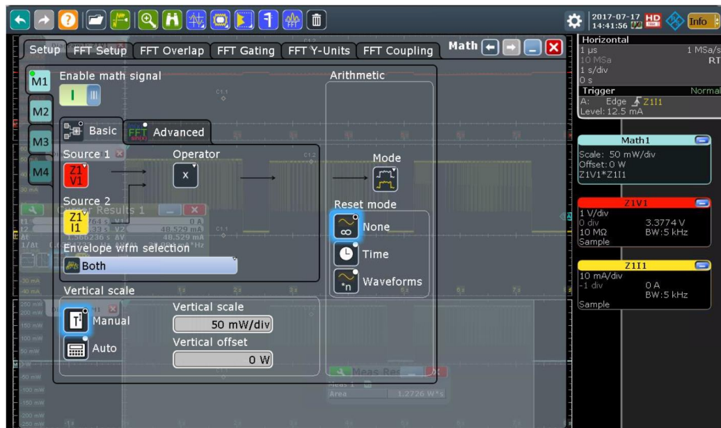
Fig. 5-6: Math function configuration on the RTO
