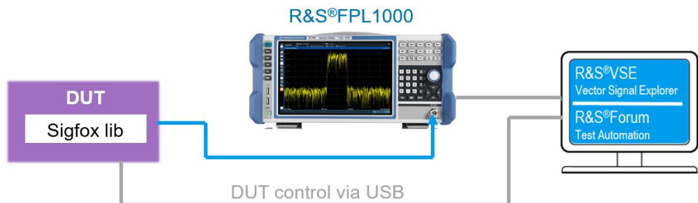
Fig. 3-1: Sigfox uplink testing (spectrum)
