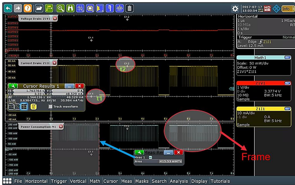
Fig. 5-7: Power consumption measurement results on the RTO
