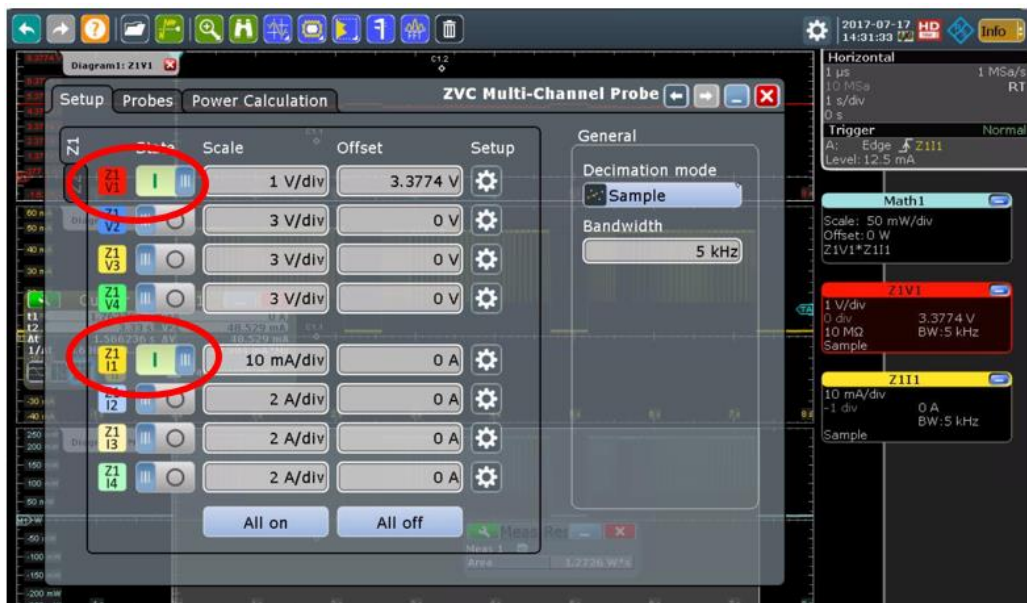
Fig. 5-3: ZVC measurement configuration on the RTO
