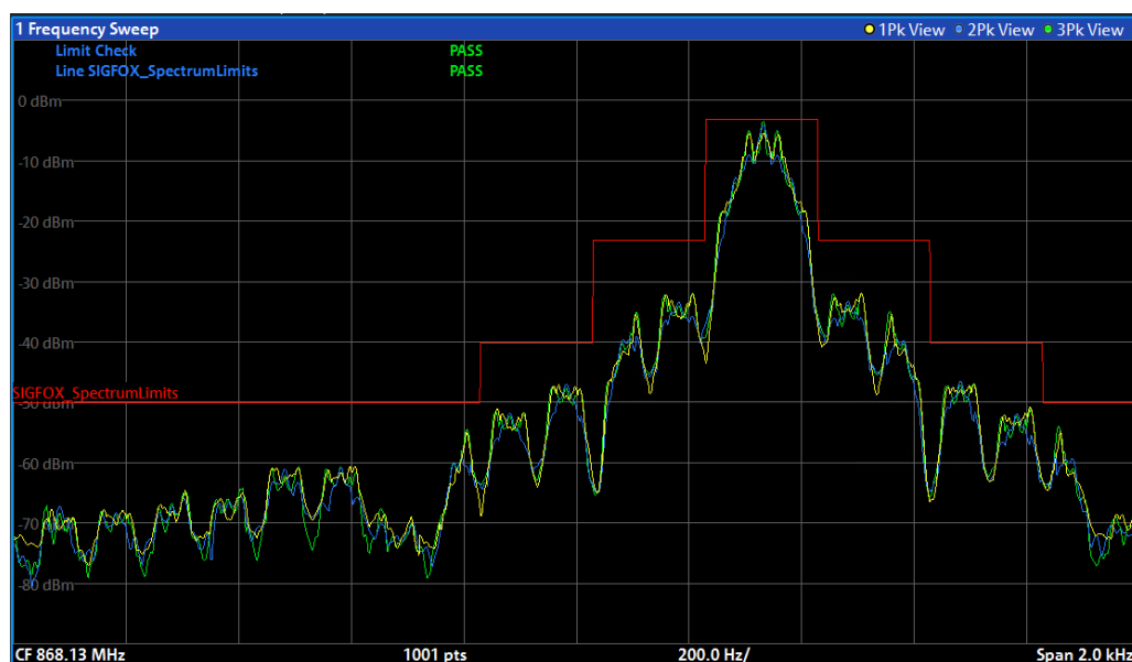
Fig. 3-8: Sigfox spectrum requirements programmed as FPL limit lines
