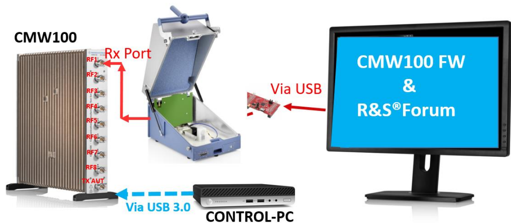
Fig. 3-14: Test setup for production testing of Sigfox devices using the CMW100
