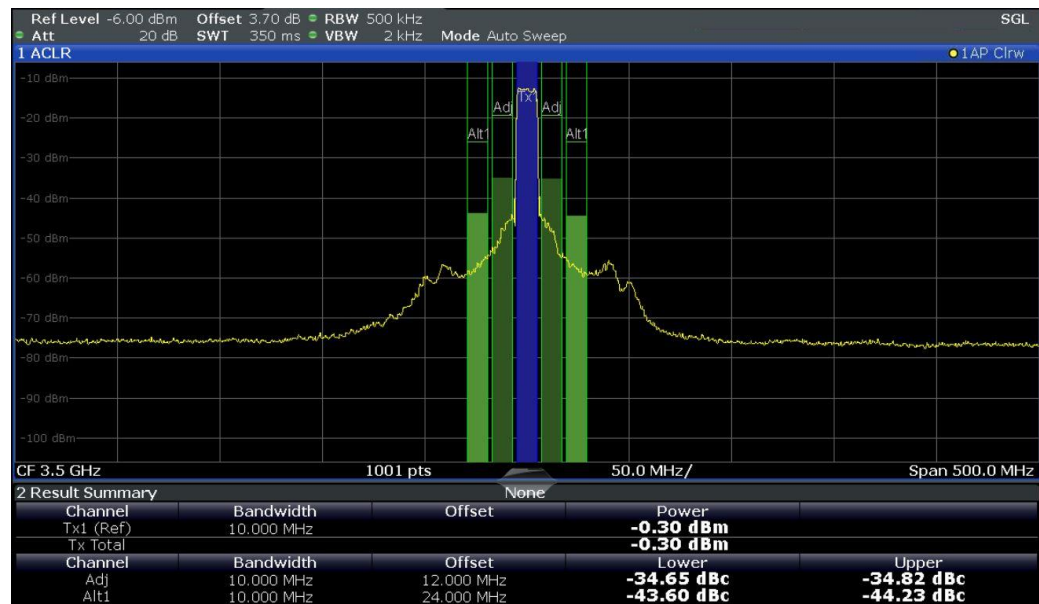
Fig. 4-4: FSW spectrum analysis of the ER output signal
