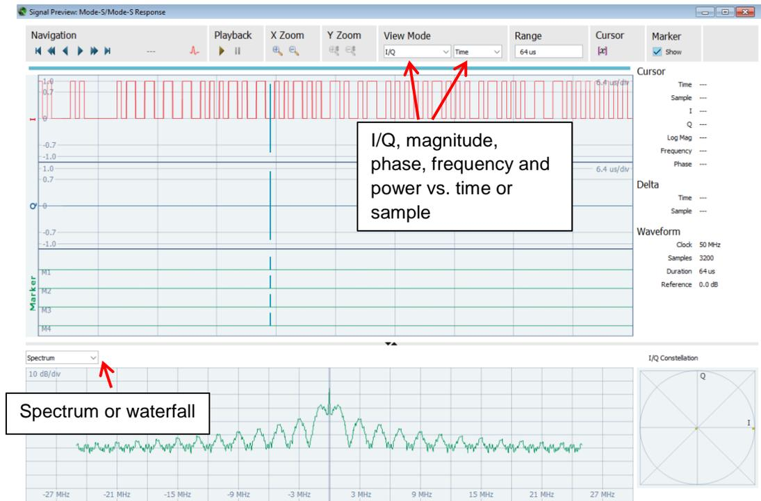
Figure 19: View the waveform of the Mode-S downlink
