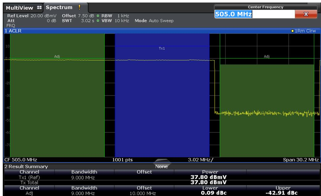
Fig. 5-54: NPR of a typical C-Line amplifier calculated with ACLR
