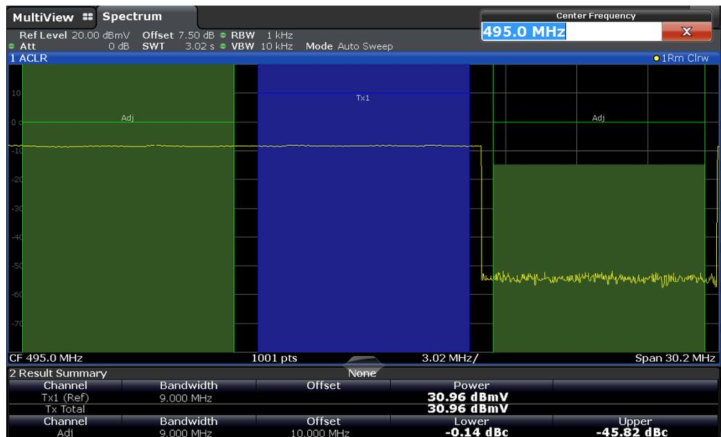
Fig. 5-55: NPR of a typical A-Line amplifier calculated with ACLR
