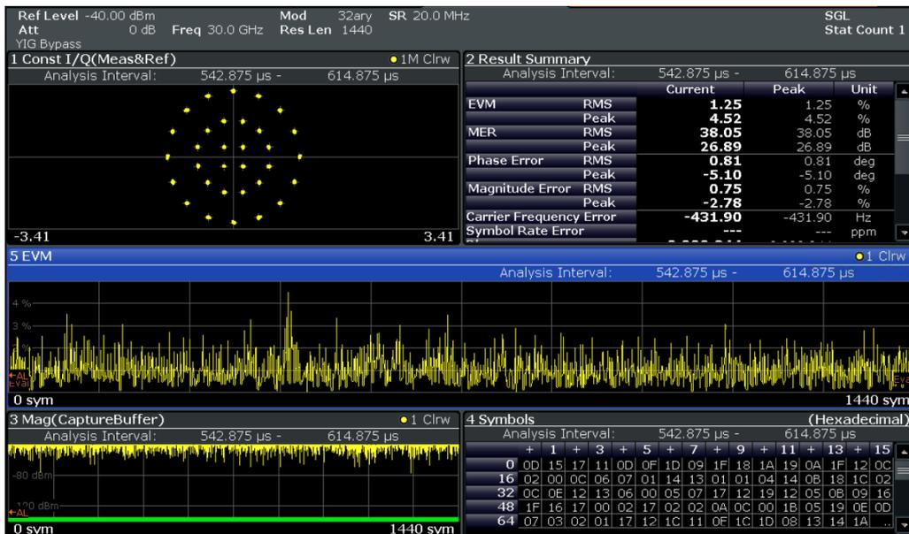
Figure 15: DVB-S2 Signal Analysis using FSW-K70 at 30 GHz
