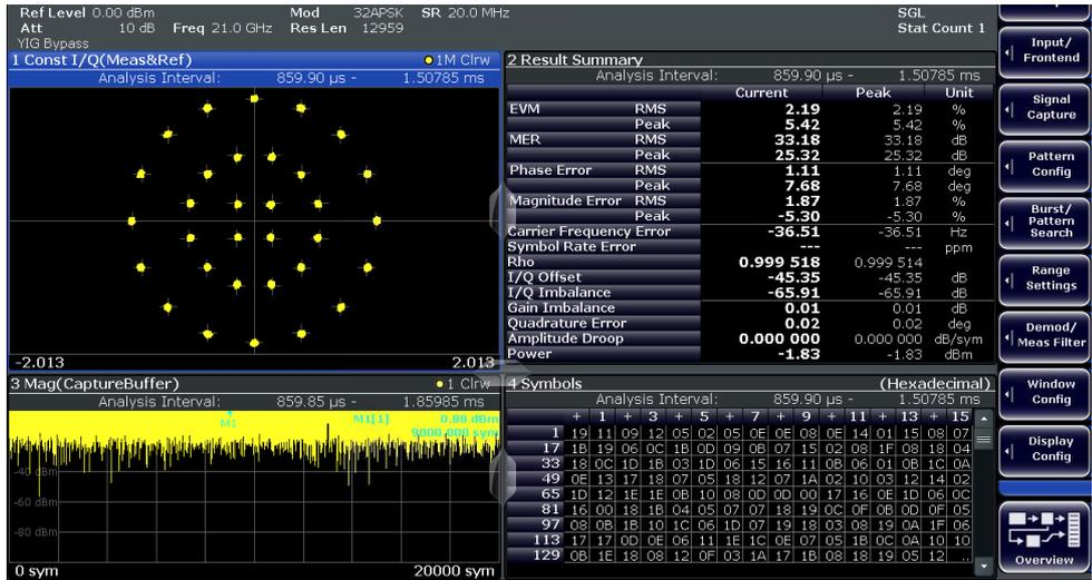
Figure 10: DVB-S2 Signal Analysis using FSW-K70 at 21 GHz
