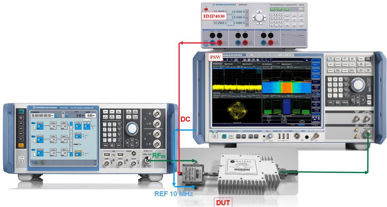
Figure 6: DVB-S2 & DVB-S2X Signal Generated using SMW and Signal Quality Analysis using FSW
