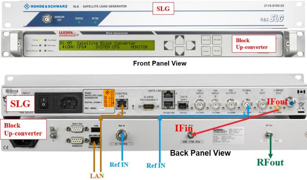
Figure 3: Front & Back Panel View of Equipment Connection
