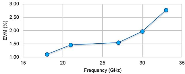
Figure 8: EVM measurement on DVB-S2X 256APSK signal generated using BTC and analyzed using FSW at different frequencies
