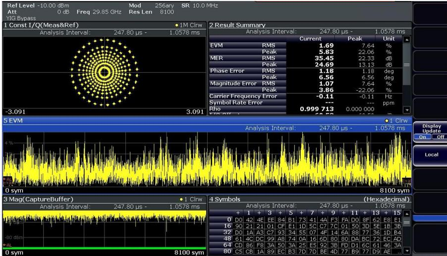
Figure 16: DVB-S2X Signal Analysis using FSW-K70 at 29.85 GHz (Ka-band)
