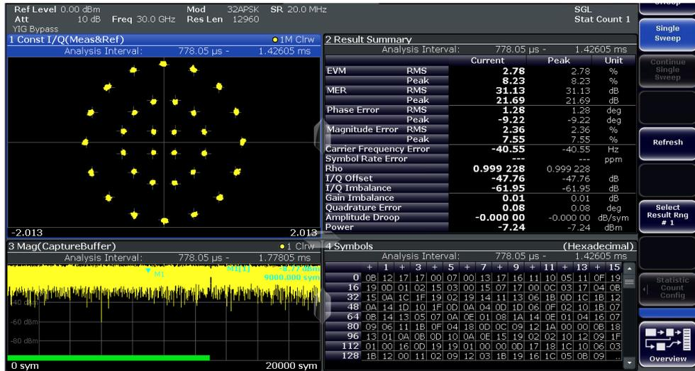
Figure 11: DVB-S2 Signal Analysis using FSW-K70 at 30 GHz
