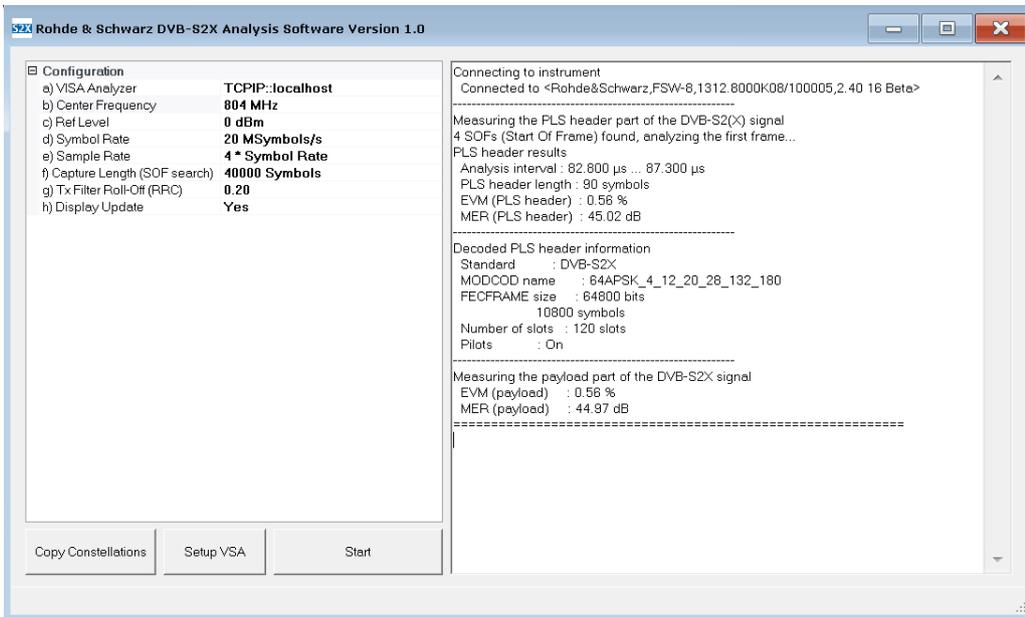
Figure 4: Screenshot of the DVB-S2X Analysis software running on an R&S FSW. A onetime "Copy Constellations" is required. "Setup VSA" sets up the MSRA and VSA channels. "Start" initiates the measurement.
