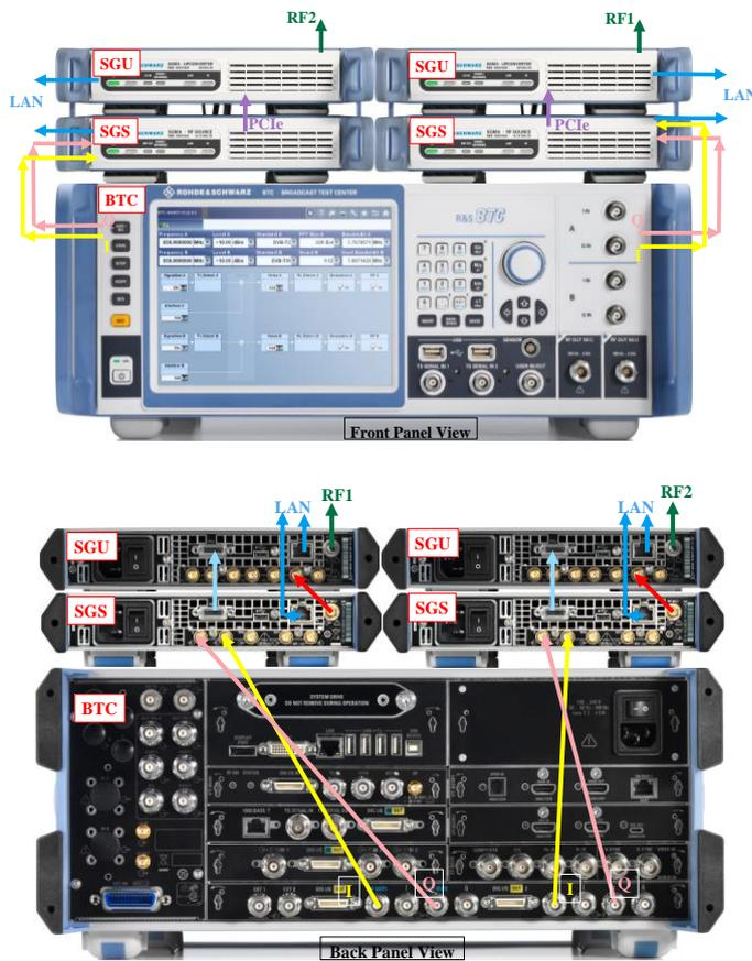
Figure 1: Front & Back Panel View of Equipment Connection
