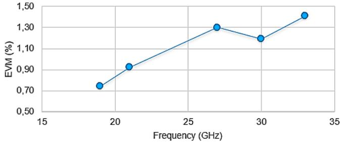
Figure 12: EVM measurement on DVB-S2X 256APSK signal generated using SMW and analyzed using FSW at different frequencies
