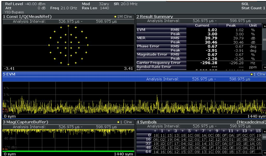
Figure 14: DVB-S2 Signal Analysis using FSW-K70 at 21 GHz
