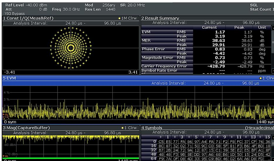
Figure 13: 256APSK modulated DVB-S2X signal measurement on the FSW at 30 GHz
