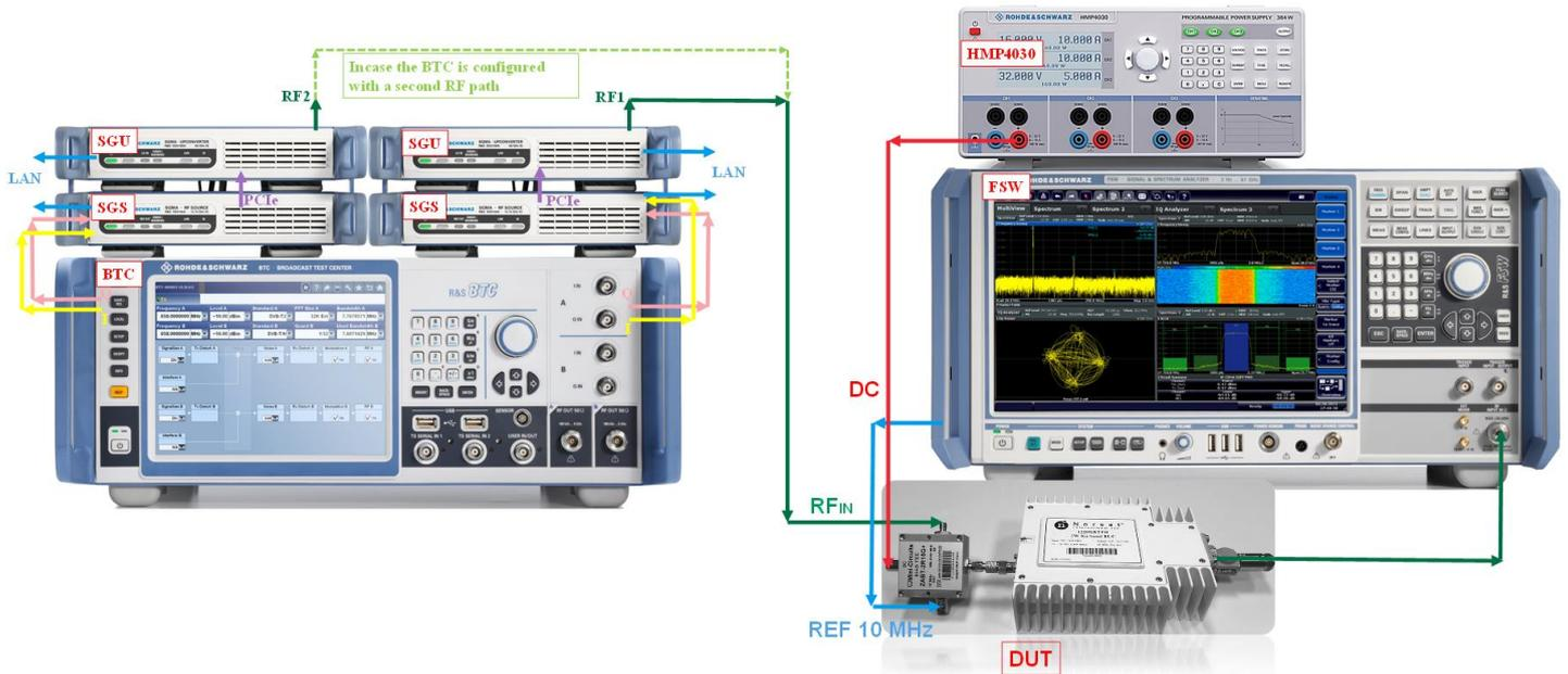
Figure 5: Generated DVB-S2 & DVB-S2X Test Signal Quality Analysis using FSW
