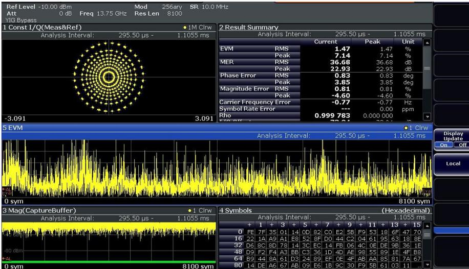
Figure 17: DVB-S2X Signal Analysis using FSW-K70 at 13.75 GHz (Ku-band)
