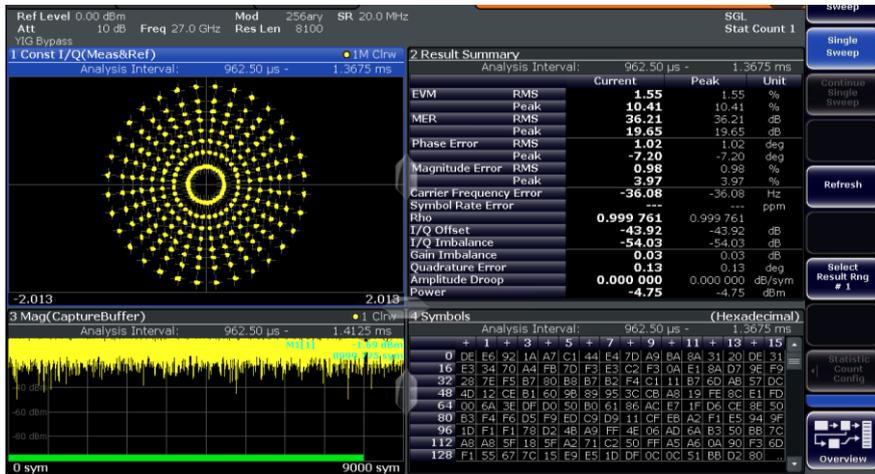
Figure 9: 256APSK modulated DVB-S2X signal measurement on the FSW at 27 GHz
