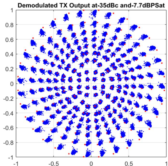
Fig. 5-16: Demodulated 256-APSK for the reference TWTA operating at -35dBc spectral regrowth
