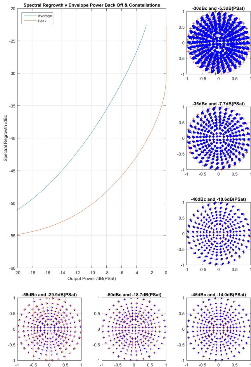
**Fig. 5-17: Swept drive level showing average and peak envelope levels and demodulated constellations at 5dB increments in spectral regrowth for the reference TWTA**
