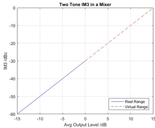
Fig. 4-1: Typical mixer two-tone third order intermodulation (IM3) from (3)
