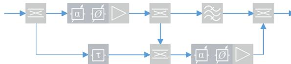
Fig. 5-7: An example feedforward schematic for the linearization of the reference TWTA
