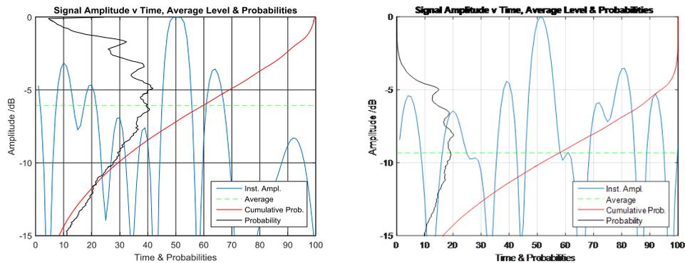
**Fig. 5-21: Amplitude and key statistics for the -45dBc/40W signal using the feedforward embodiment (left), alongside the clean modulator output (right)**
