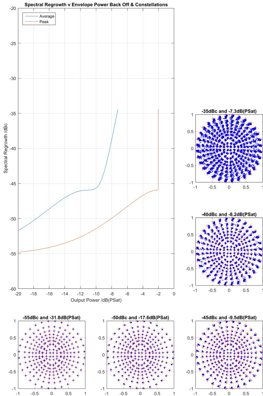
**Fig. 5-19: Swept drive level showing average and peak envelope levels and demodulated constellations at 5dB increments in spectral regrowth for the feedforward TWTA**
