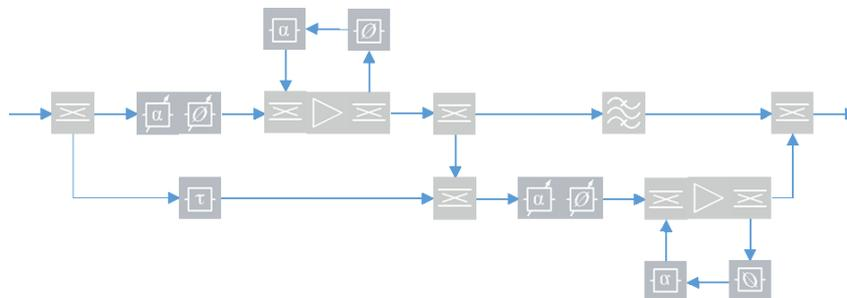
Fig. 5-12: Implementation of hybrid feedback and feedforward linearization
