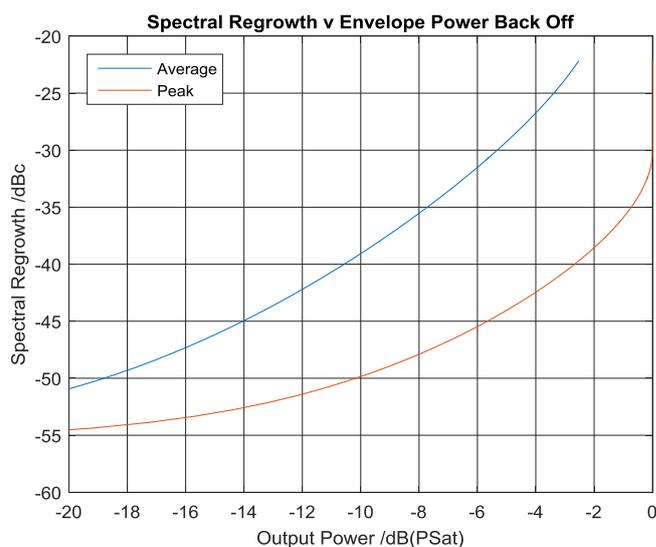
**Fig. 5-15: Spectral regrowth versus output level for the reference TWTA, without linearization, showing average and peak envelope amplitudes**
