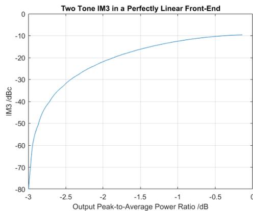
Fig. 4-2: Two-tone third-order intermodulation distortion (with 3dB source PAPR) versus output PAPR in a perfect frontend
