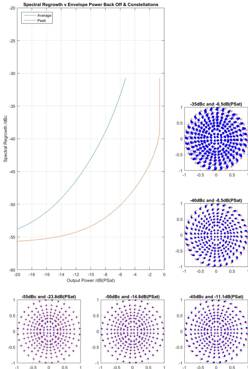
**Fig. 5-18: Swept drive level showing average and peak envelope levels and demodulated constellations at 5dB increments in spectral regrowth for the feedback TWTA**
