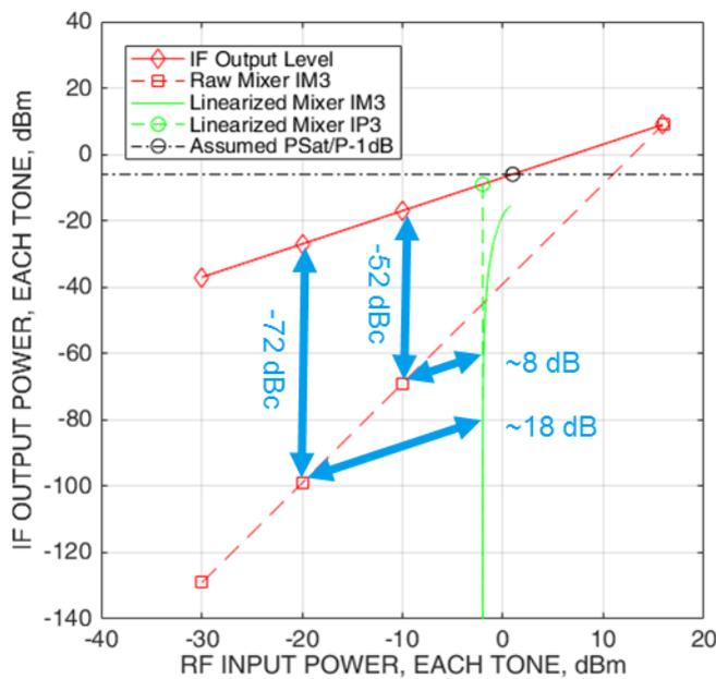
Fig. 4-3: Off-the-shelf Mixer and Linearized Mixer, IM3 and OIP3
