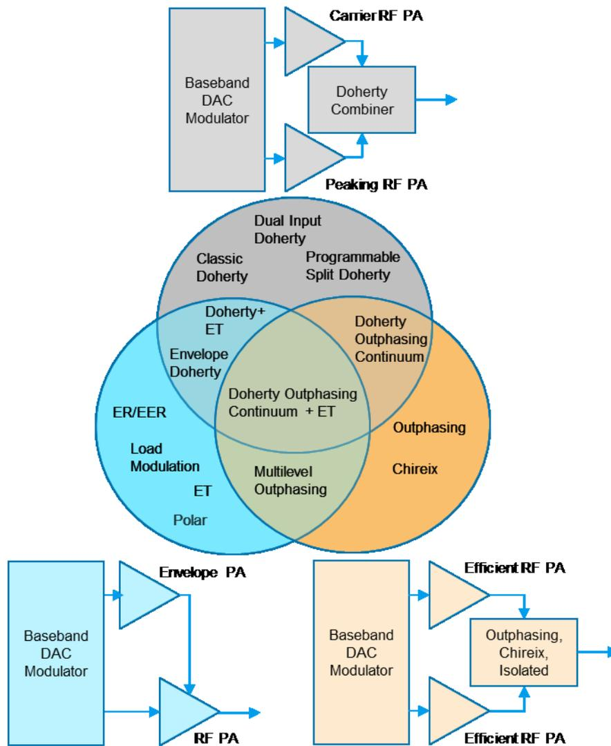
Fig. 6-1 - Extension of example multiple-input TxFE architectures, developed from (8)
