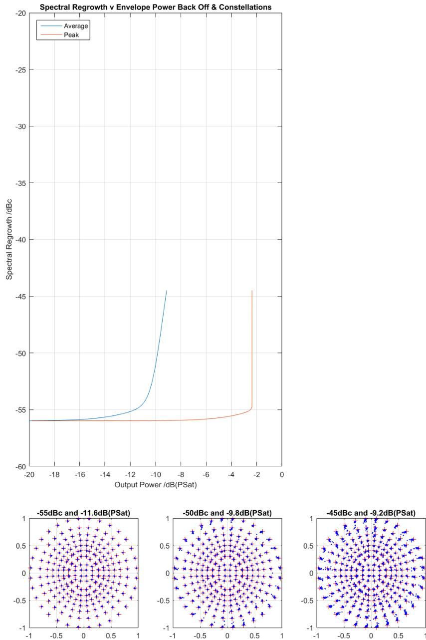
**Fig. 5-20: Swept drive level showing average and peak envelope levels and demodulated constellations at 5dB increments in spectral regrowth for the hybrid feedback/feedforward TWTA**
