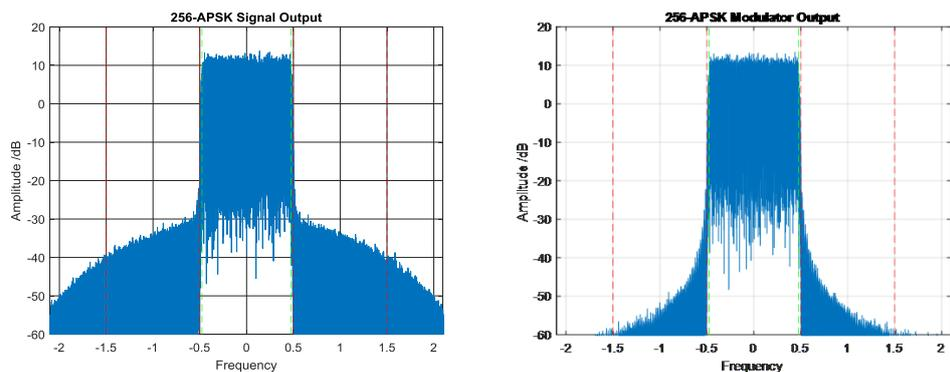
**Fig. 5-22: Spectrum output of the feedforward TWTA operating at -45dBc (left) alongside the modulator output (right)**
