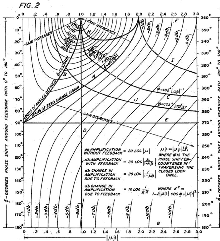
$\mu\beta$ , WHICH IS INDICATIVE OF THE AMOUNT OF FEEDBACK, IS A COMPLEX QUANTITY WHICH MAY BE VIEWED AS REPRESENTING THE RATIO BY WHICH THE AMPLIFIER AND FEEDBACK CIRCUIT (OR IN GENERAL  $\mu$  AND  $\beta$ ) MODIFY A VOLTAGE IN A SINGLE TRIP AROUND THE CLOSED PATH.
