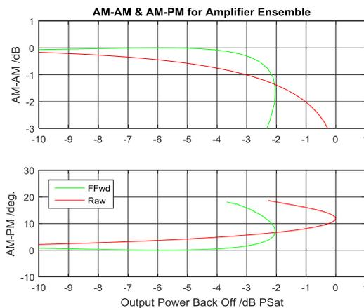
Fig. 5-8: Comparison of the feedforward and reference TWTA characteristics
