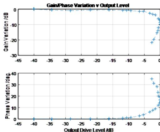
Fig. 5-5: AM-AM and AM-PM characteristics of the TWTA in (2)
