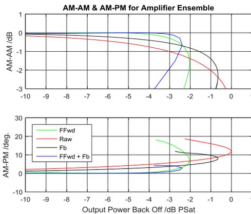
**Fig. 5-14: Ensemble of feedback, feedforward, reference and hybrid TWTA characteristics**
