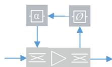
Fig. 5-10: An example direct RF feedback schematic for linearization of the reference TWTA
