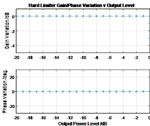
Fig. 3-1: The hard limiter's AM-AM and AM-PM characteristics
