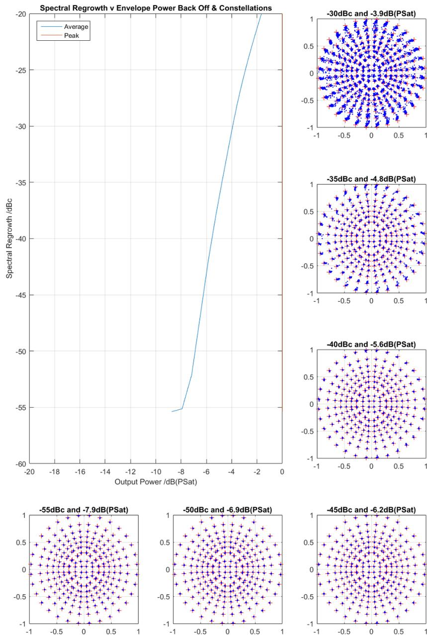
**Fig. 5-4: Drive level sweep for 256-APSK through the hard limiter**
