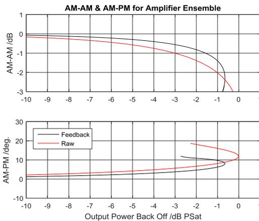
Fig. 5-11: Comparison of the feedback and the reference TWTA characteristic
