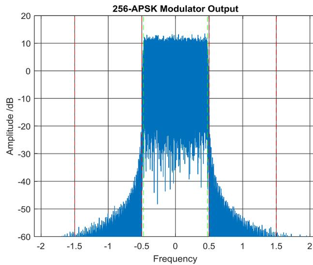
Fig. 5-2: Spectrum of the clean 256-APSK signal with 0,05 roll-off factor
