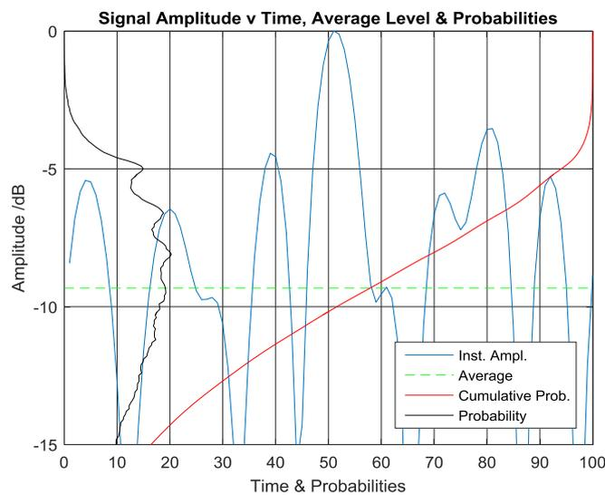
Fig. 5-3: Extracted time domain amplitude and bulk signal statistics for the 256-APSK signal
