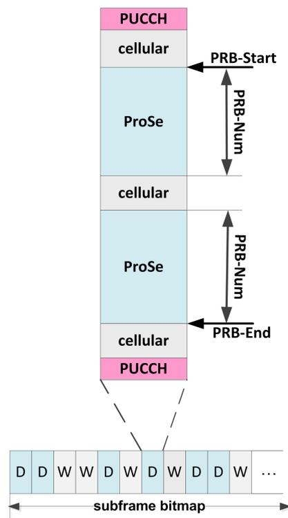
Fig. 3-3: Resource Pool for SL Communication. Subframes to be used for the RP are indicated in blue.
