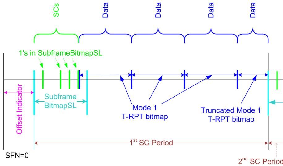
Fig. 3-4: Example of a subframe allocation for Mode 1
