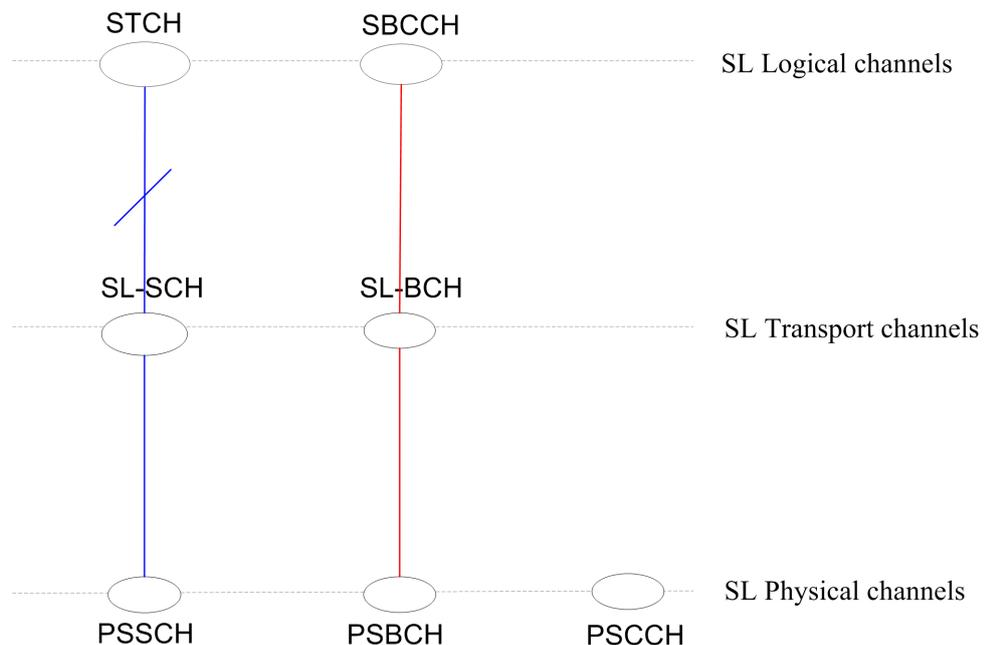
**Fig. 3-2: Sidelink channels for the air interface. In blue is the data path, whereas the path for control signaling is indicated in red.**
