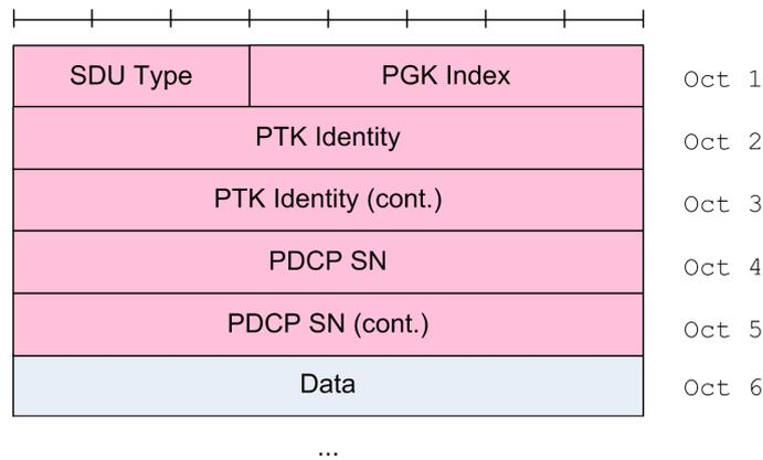
**Fig. 5-5: PDCP header for SL communication [5]**
