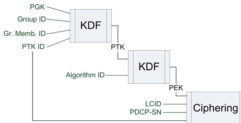
**Fig. 5-3: Key derivation for data ciphering. The two KDFs are different, they are described in Annex A3 and A4 of [12], respectively.**
