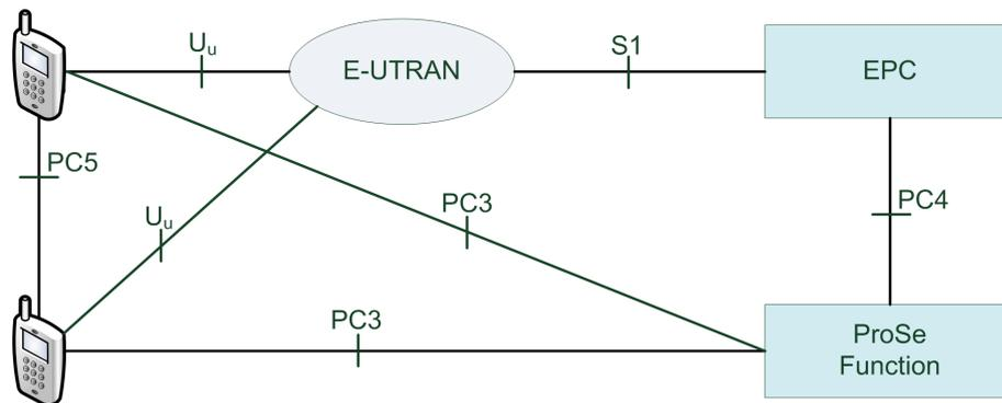
Fig. 2-2: Simplified architecture for ProSe (non-roaming)
