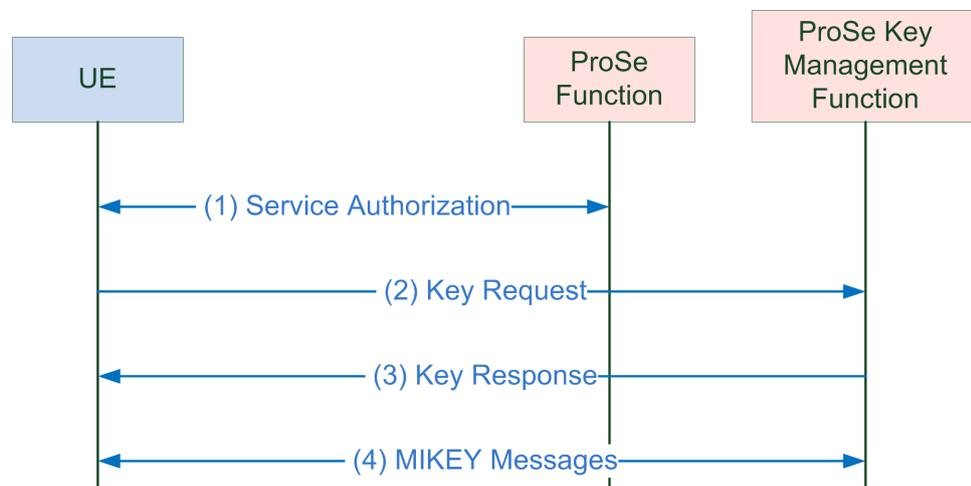
**Fig. 5-2: Key exchange procedure to provide the UE with the required parameters**
