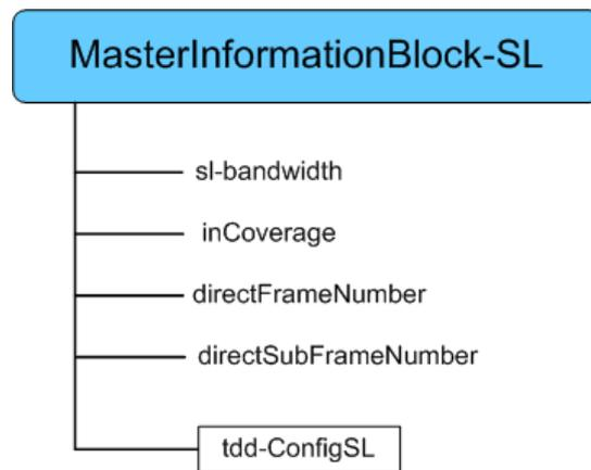
Fig. 4-1: MIB-SL transmitted from a UE
