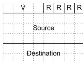
**Fig. 3-10: SL-SCH subheader, prepended to the legacy fields in the MAC header [7]**
