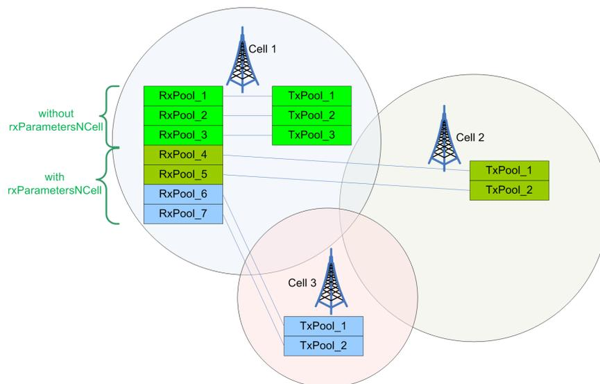
**Fig. 4-8: Example of an rx pool configuration**
