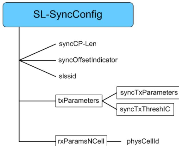
**Fig. 4-4: SL-SyncConfig information element with the content for sidelink operation**
