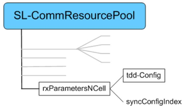
**Fig. 4-7: Indication that the UE has to synchronize to the sender**
