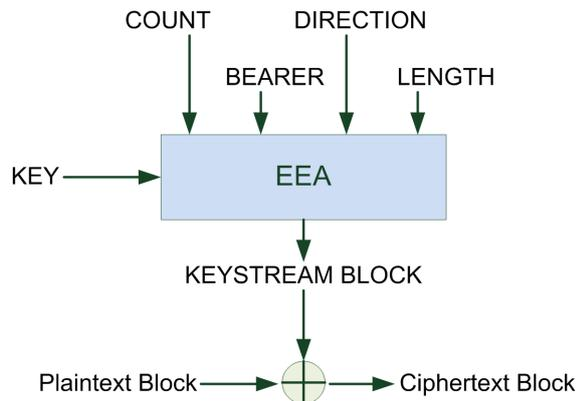
**Fig. 5-4: Data encryption for ciphering. The different ciphering methods are realized by choosing the pertinent EEA procedure (source: [13])**
