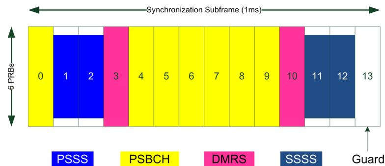
Fig. 4-2: Subframes used for the synchronization signals PSSS, SSSS, DMRS, and MIB-SL contained in the PSBCH
