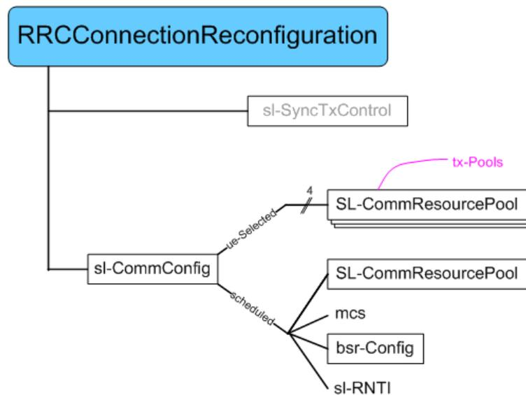
**Fig. 3-8: Extensions of the RRCConnectionReconfiguration message for SL-Communication**
