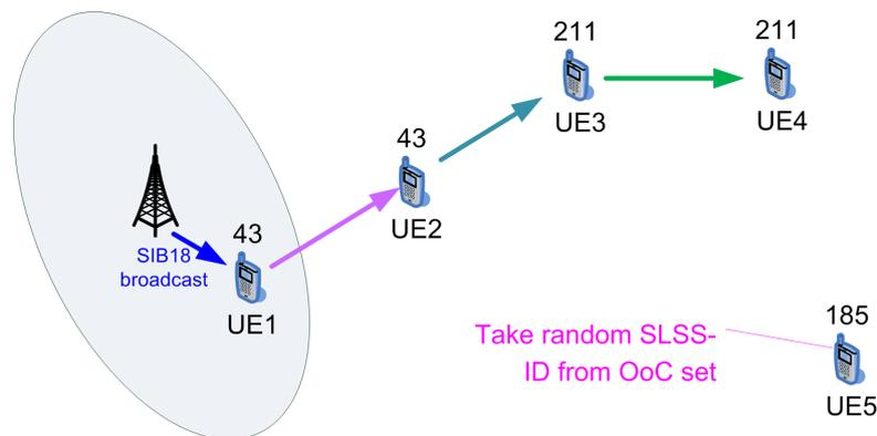
**Fig. 4-6: Example network configuration. The numbers indicate the SLSS ID which the UE uses when it transmits the SLSS itself.**
