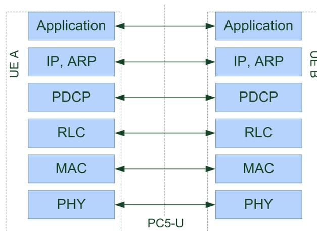
**Fig. 2-3: Radio protocol stack for data transmission [3]**
