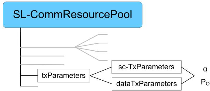
Fig. 3-11: Tx parameter in the resource pool for power control
