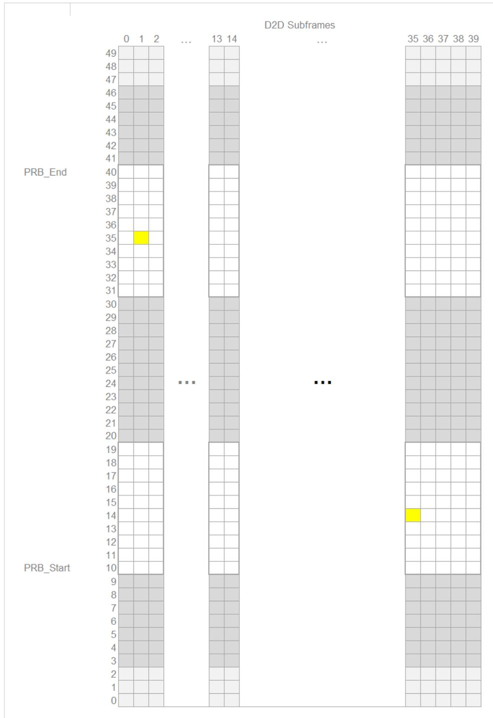
**Fig. 3-9: Example of SCI0 transmissions in the control region of the SC Period. Only the subframes indicated with 1 in the SubframeBitmapSL are shown.**
