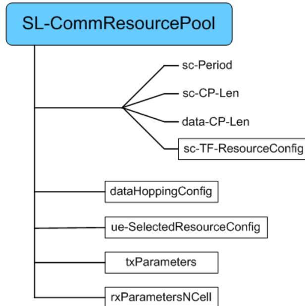
**Fig. 3-5: Resource pool structure in RRC signaling**
