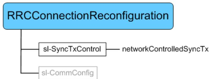
**Fig. 4-3: Network controlled transmission of Synchronization Signals**
