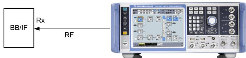
Figure 5-2: RX test setup on the BB/IF chip – in principle, the same as the overall setup. However, a cable connection can be used thanks to the lower IF frequency of the BB chip and no upconverter is needed. The RF path needs the 20 GHz or 40 GHz option
