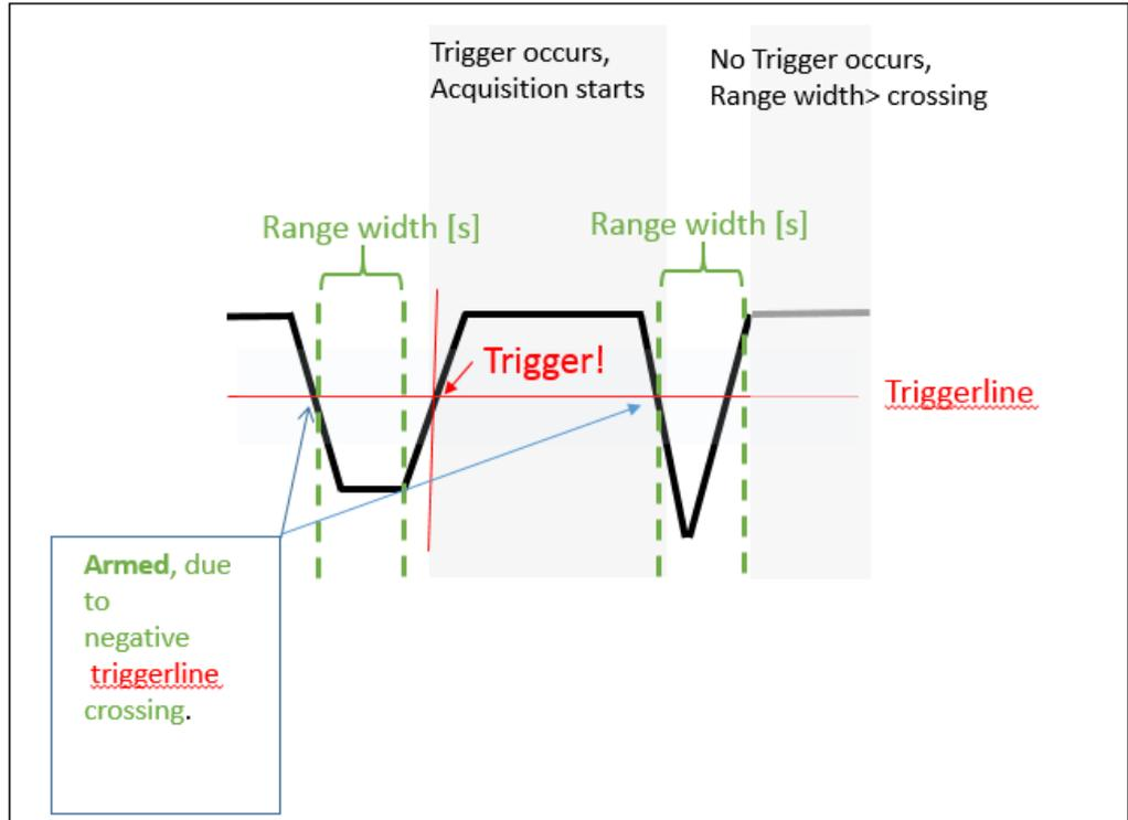
Figure 14: Width trigger schematic
