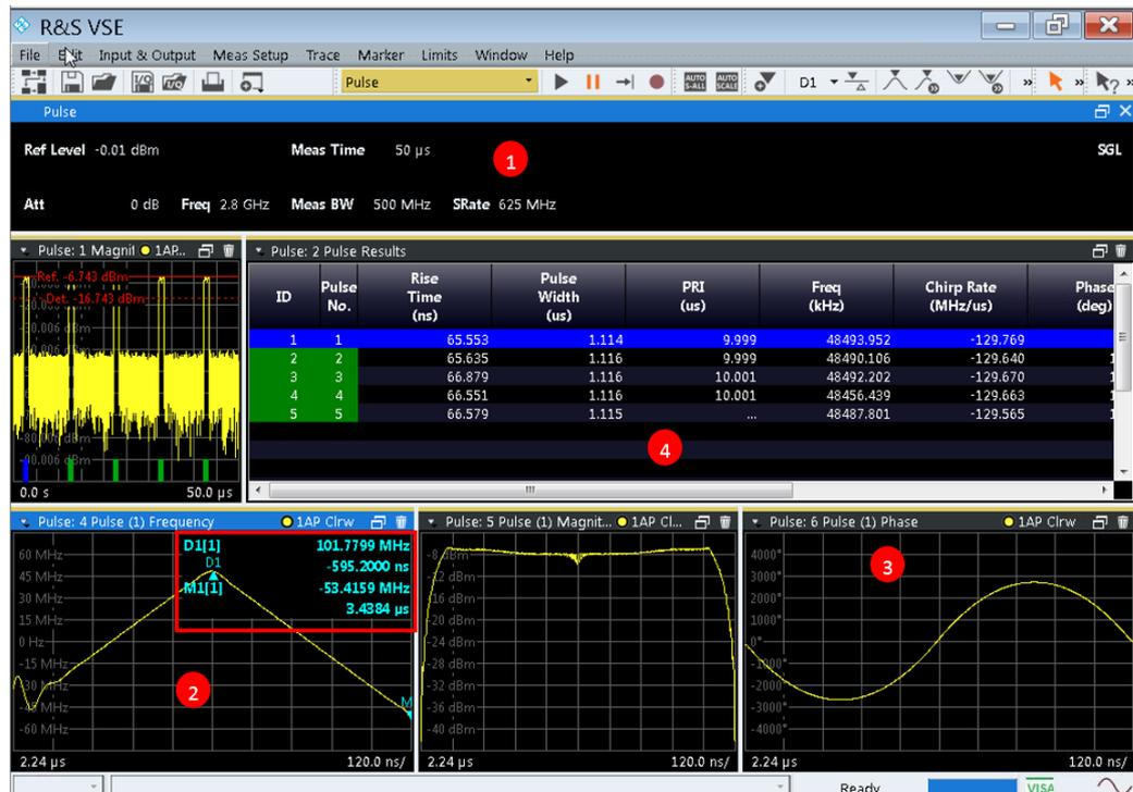
Figure 28:VSE-K6 modulation on pulse
