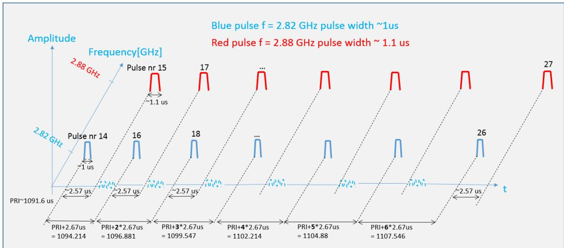
Figure 36: ATC pulse properties
