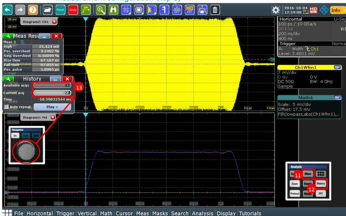
Figure 17: RTO Single pulse analysis
