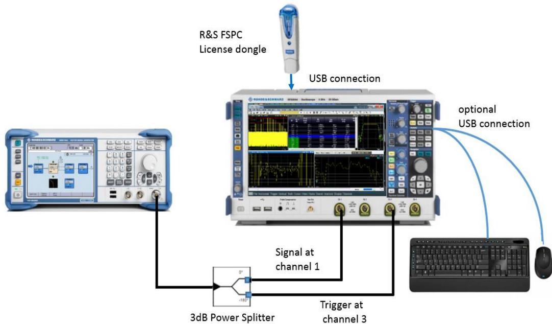
Figure 22: Lab Setup for RTO & VSE-K6
