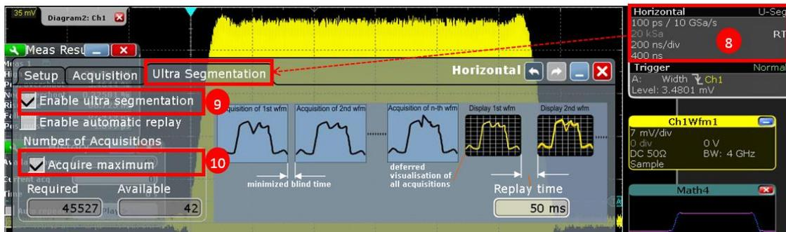
Figure 16: Horizontal/Ultra Segmentation
