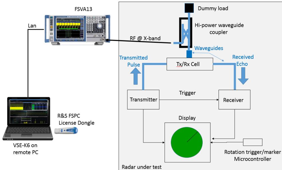
Figure 37: X-band RADAR measurement setup
