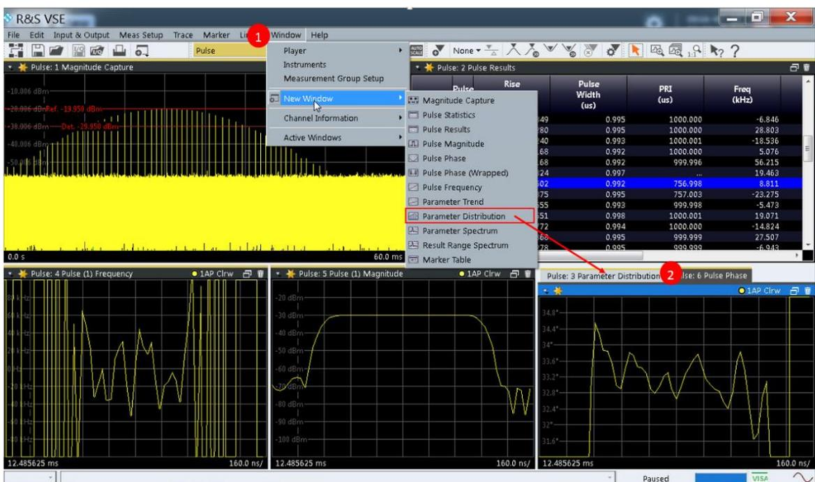
Figure 25: VSE-K6 Measurements
