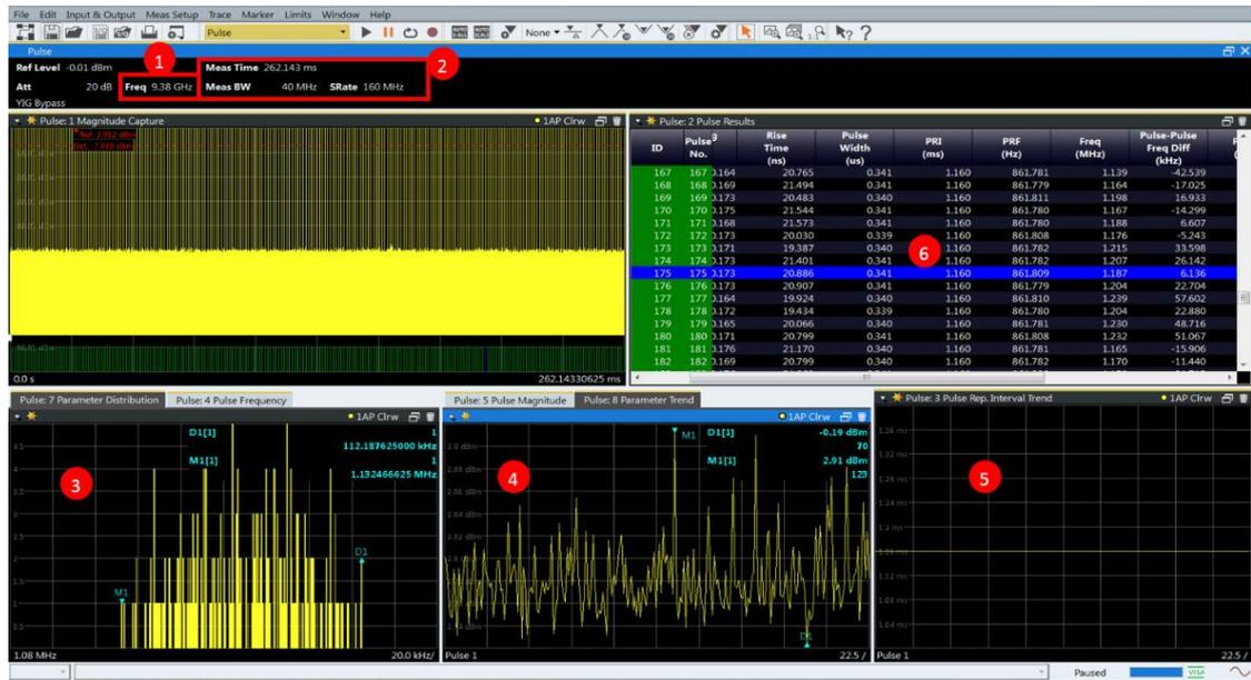
Figure 38:VSE-K6 measurement X-band radar
