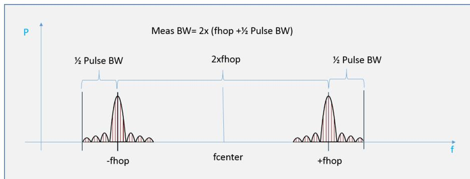
Figure 33: Measurement bandwidth calculation
