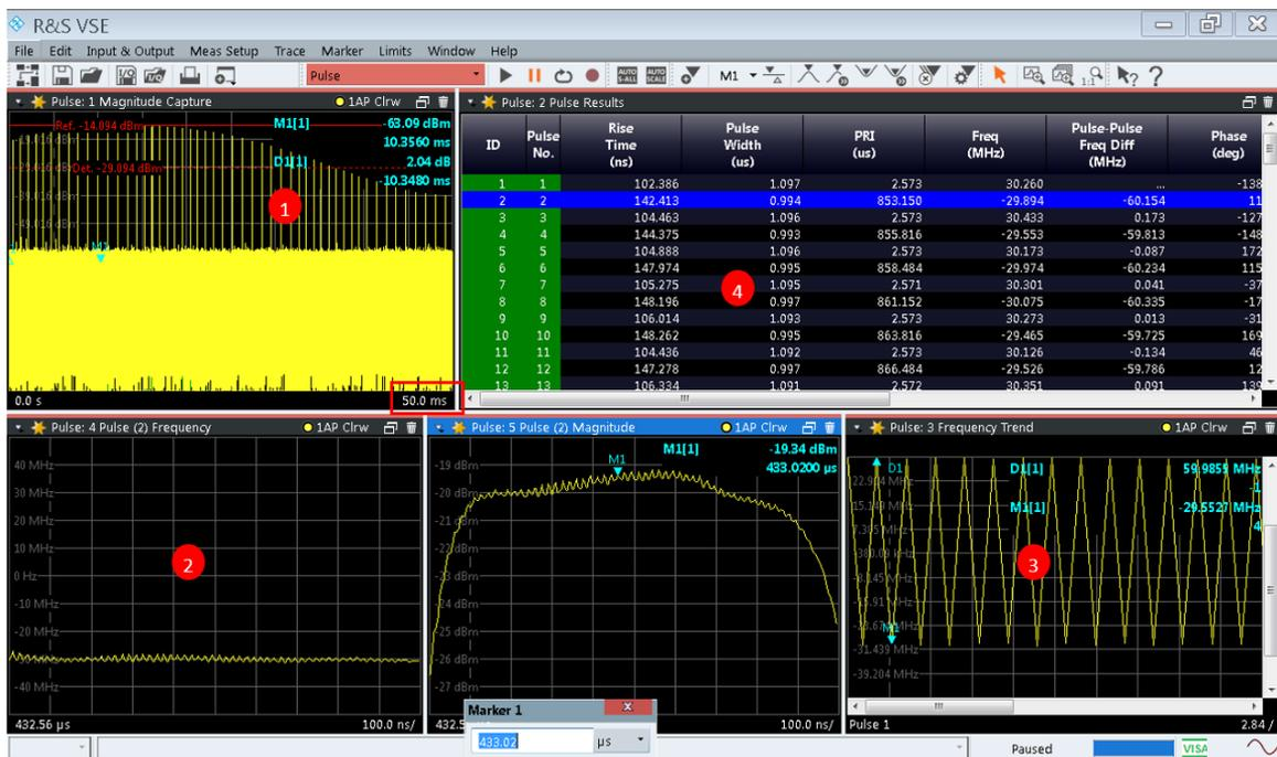
Figure 34: VSE-K6 ATC radar capture
