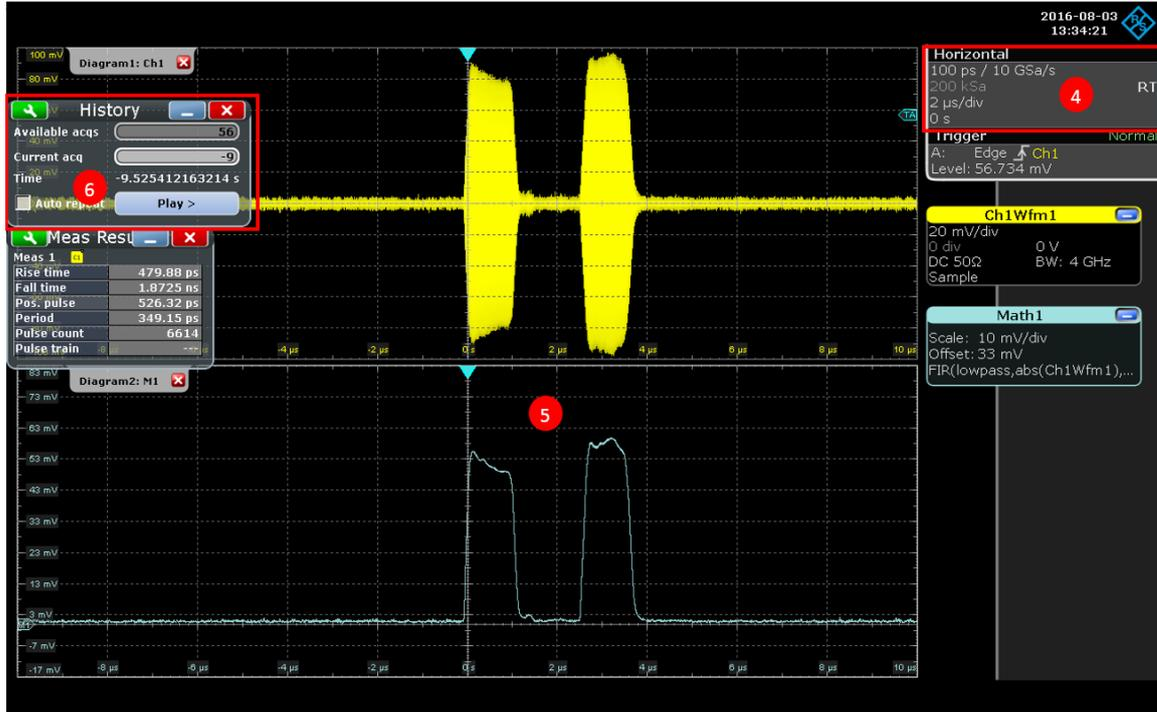
Figure 32 : ATC envelope results, the first pulse shows a magnitude droop
