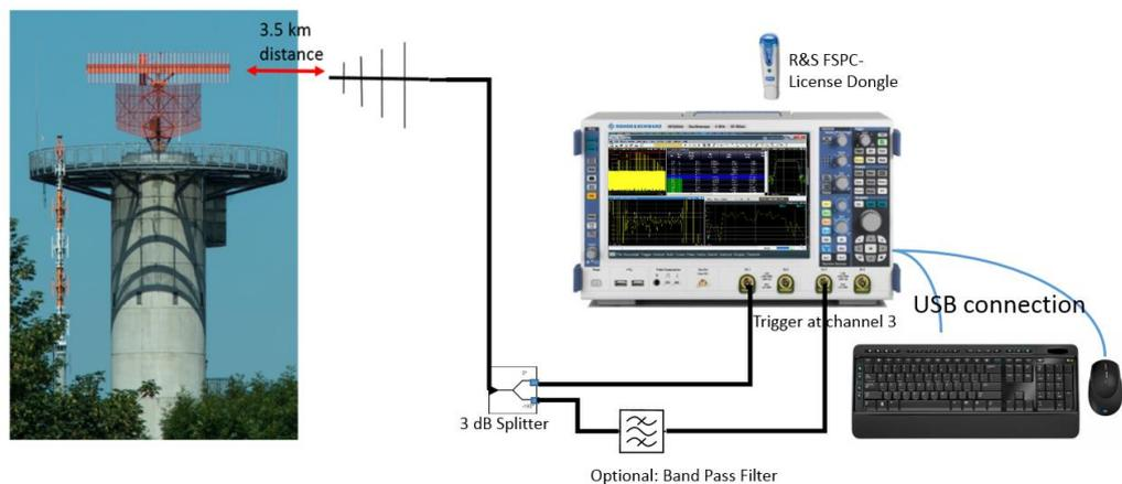
Figure 30: Field test setup
