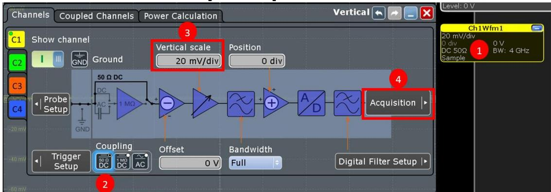
Figure 3: Channel configuration
