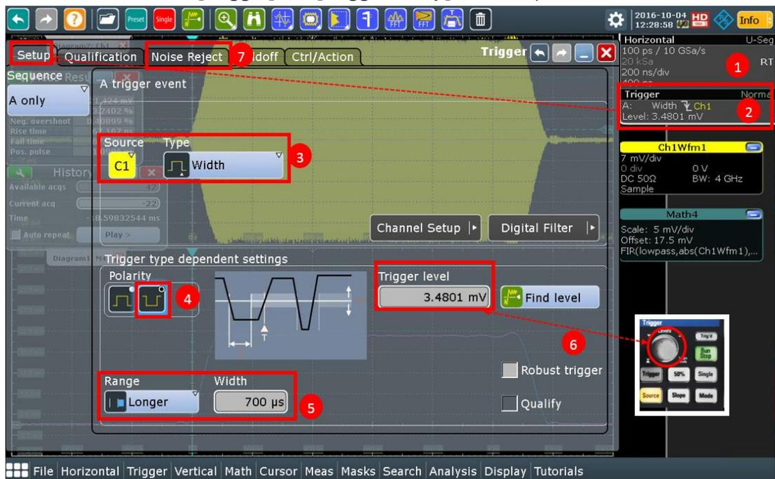
Figure 15: RTO Width trigger settings
