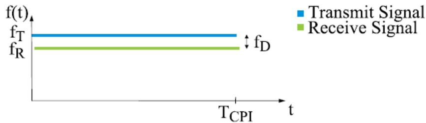
Figure 4-1: Monofrequent Continuous Wave radar.
