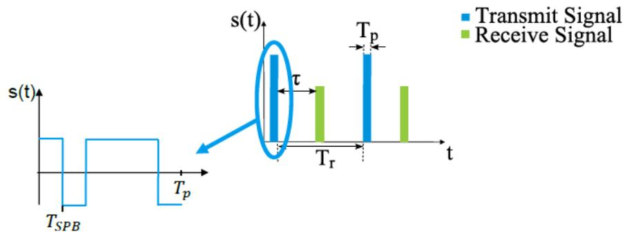
Fig. 3-3: Pulse compression in a single pulse.
