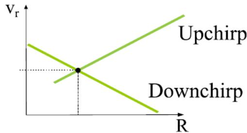
**Figure 5-2: Intersection between Up- and Downchirp Radar Echo Signals.**
