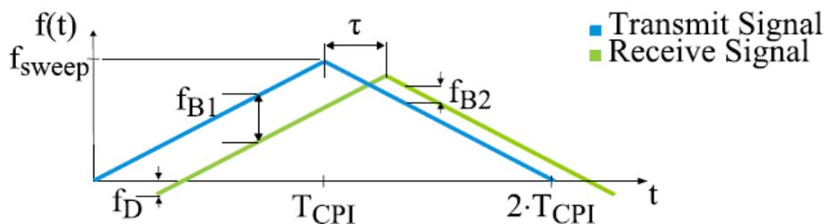
Figure 5-1: LFMCW radar with upchirp and downchirp.
