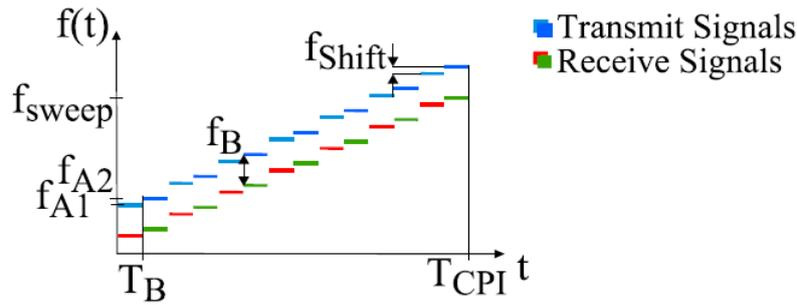
Fig. 5-4: Multiple Frequency Shift Keying.
