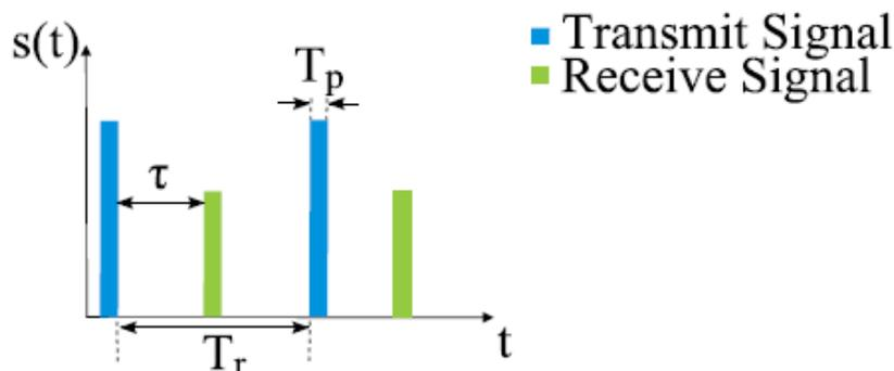
**Figure 3-1: Radar Principle.**
